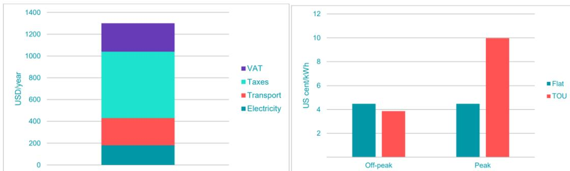
Figure 9 – a) Typical composition of electricity bill for a Danish household and b) Comparison between DSO tariffs (flat and ToU) for electricity in Copenhagen
