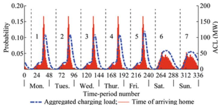
Figure 5 – Aggregated charging load and distribution of time when vehicles arrive home in the week [19]
