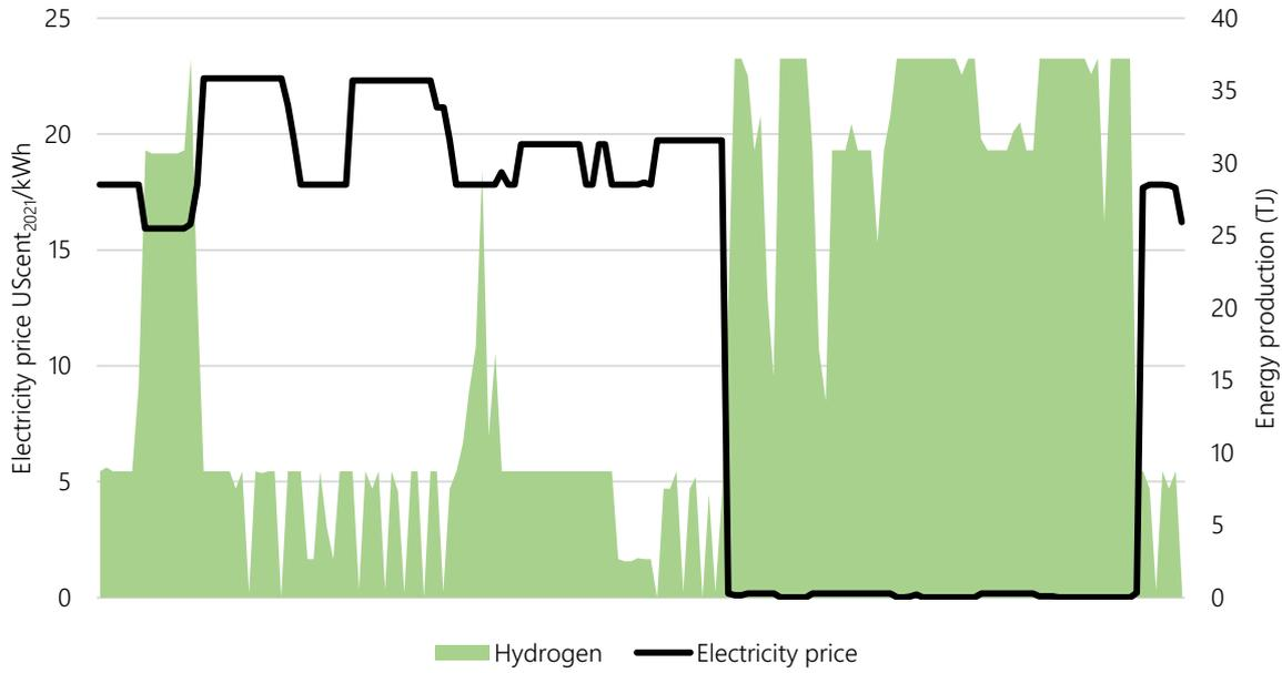
**Figure 5.13 Operation of electrolyzers during a week in 2050 for Net-Zero scenario in the South Central region.**
