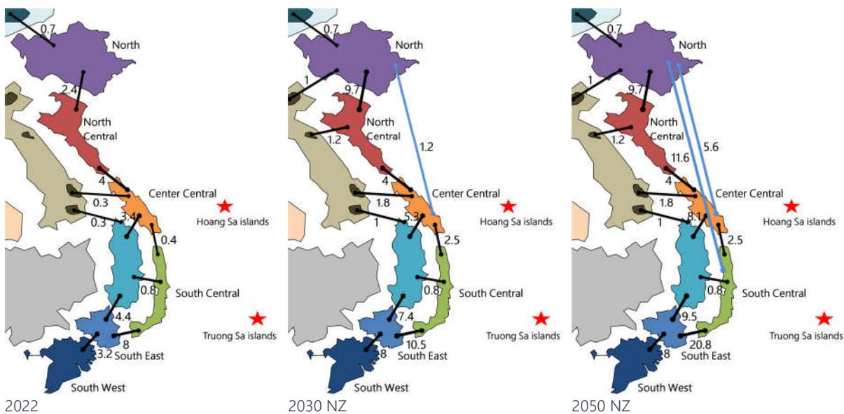
**Figure 5.6 Installed transmission lines in GW in 2022, 2030 and 2050 in the Net-Zero scenario (black lines indicate HVAC connections, and blue lines indicate HVDC connections).**
