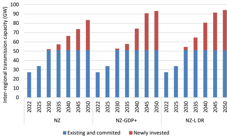
Figure 96: The inter-regional transmission capacity of NZ-GDP+ and NZ-L DR scenarios comparing with the NZ scenario.
