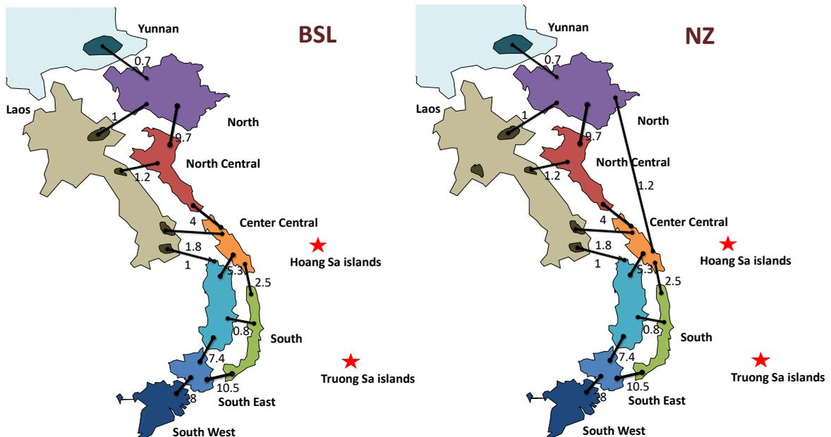
Figure 54: Transmission capacity (GW) between regions in 2030 for both core scenarios.
