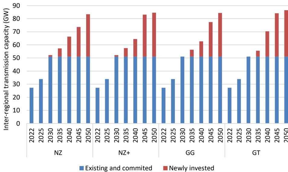
Figure 87: The inter-regional transmission capacity of main variation scenarios comparing with the NZ scenario.
