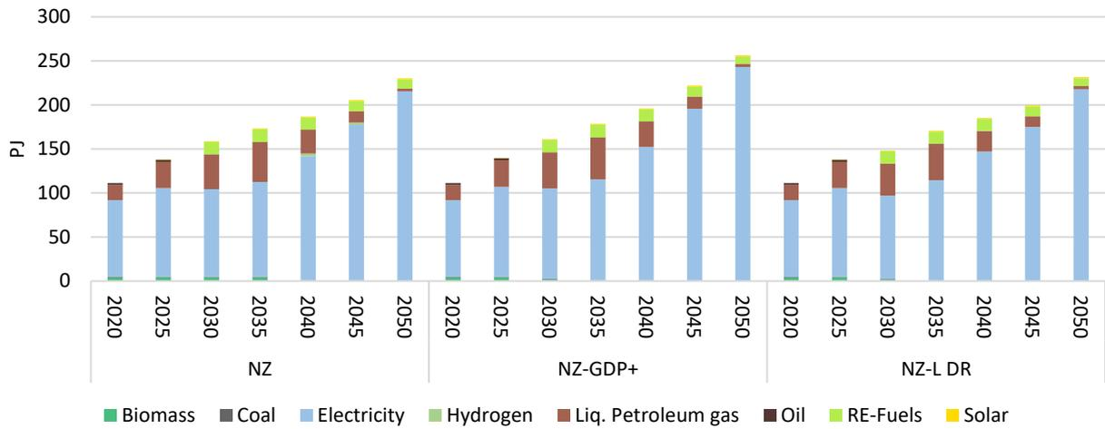
Figure 116: Final energy consumption in Services, TIMES [PJ]
