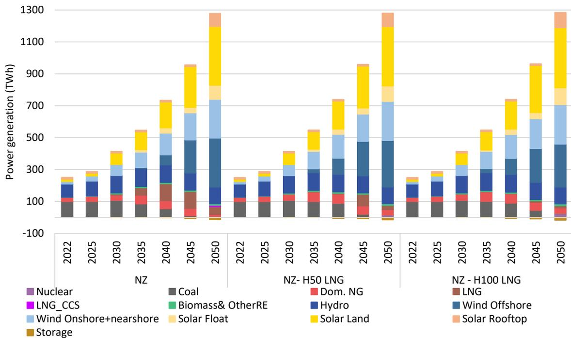
Figure 108: Power generation by technology of the NZ scenario and LNG price sensitivity scenarios.
