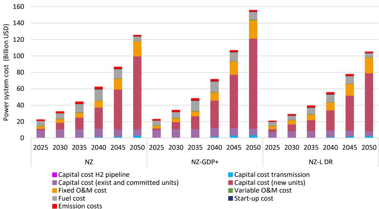
Figure 97: Power system cost of NZ-GDP+ and NZ-L DR scenarios comparing with the NZ scenario.
