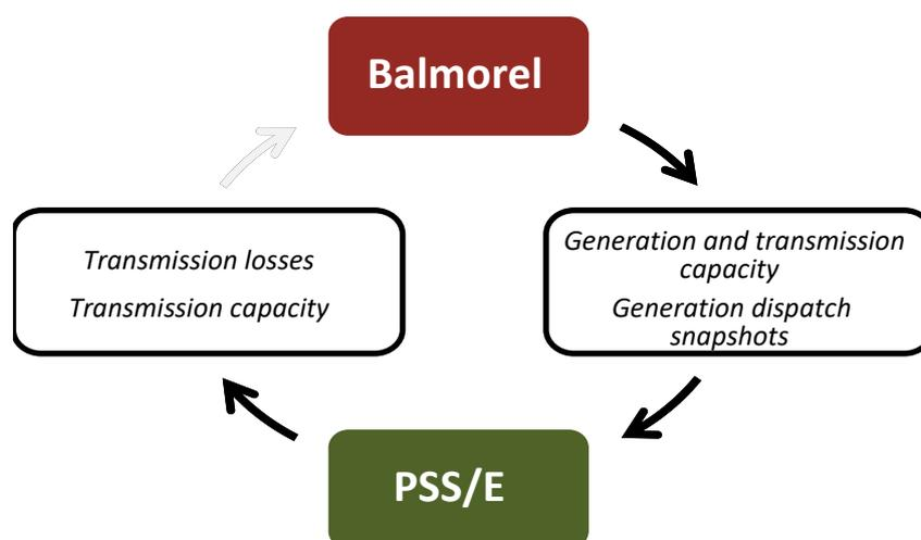
Figure 7: Linking between the Balmore and PSS/E model. Grey linking arrow has not been performed in this EOR.
