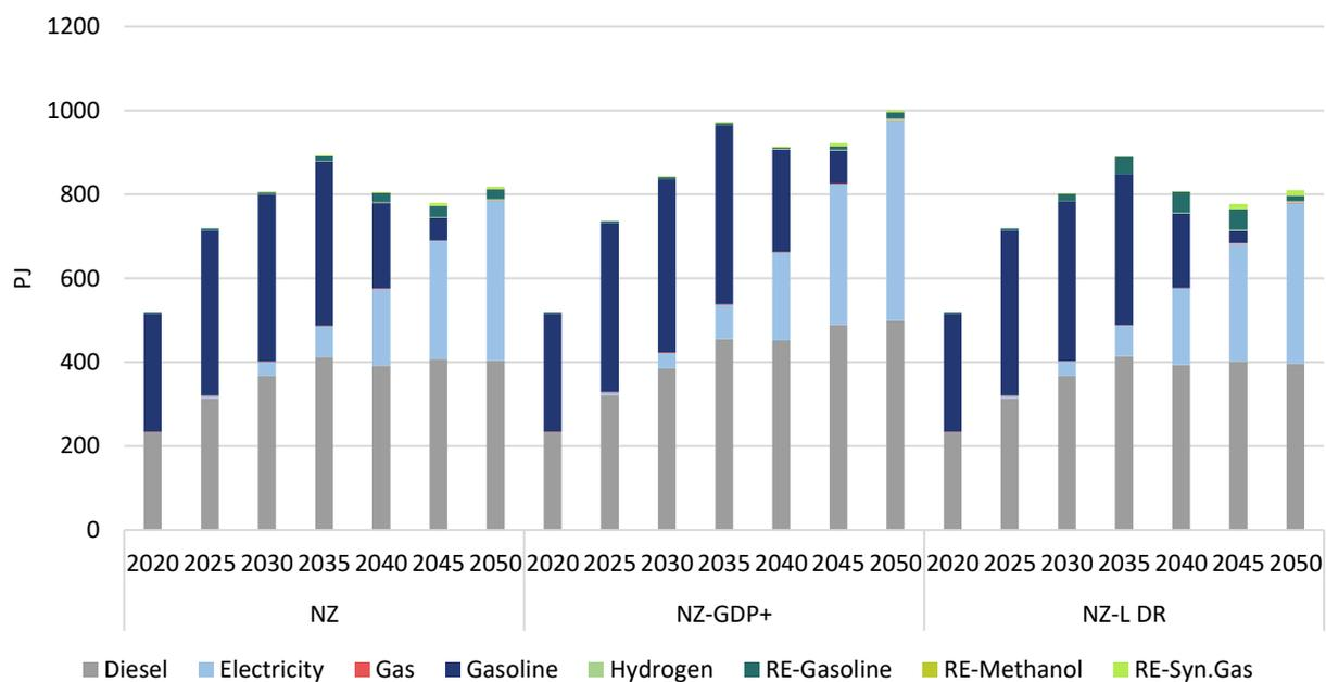
Figure 118: Road transport fuel consumption, TIMES [PJ]
