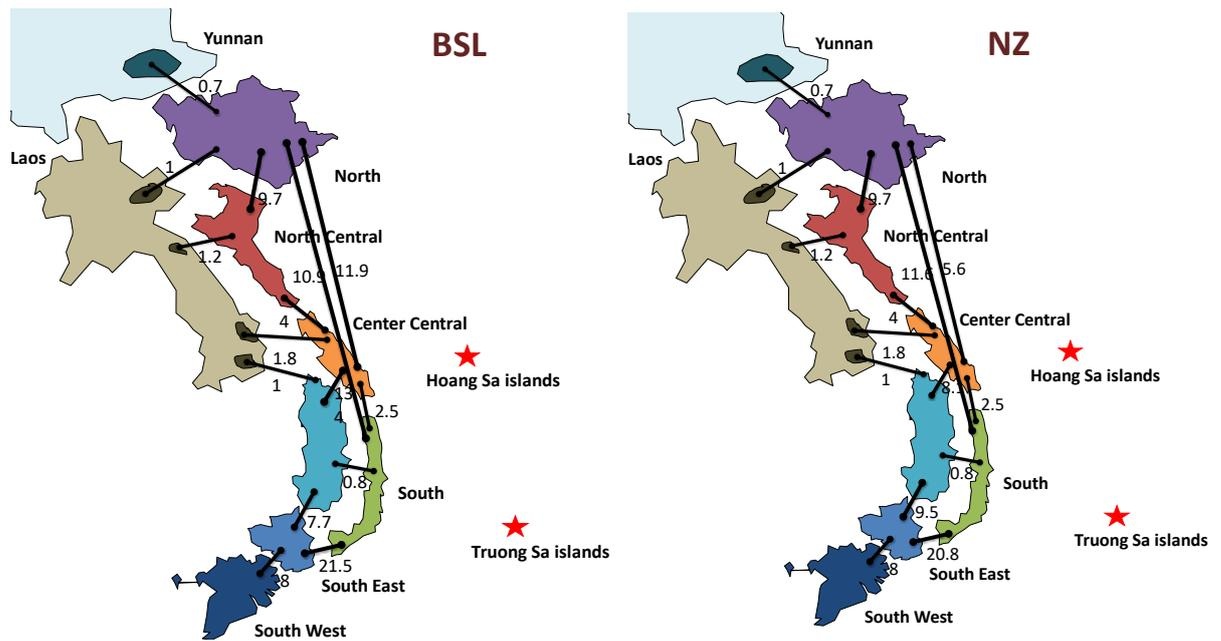
Figure 55: Transmission capacity (GW) between regions in 2050 for both core scenarios. Lines from Center Central to North and South Central to North are HVDC lines.
