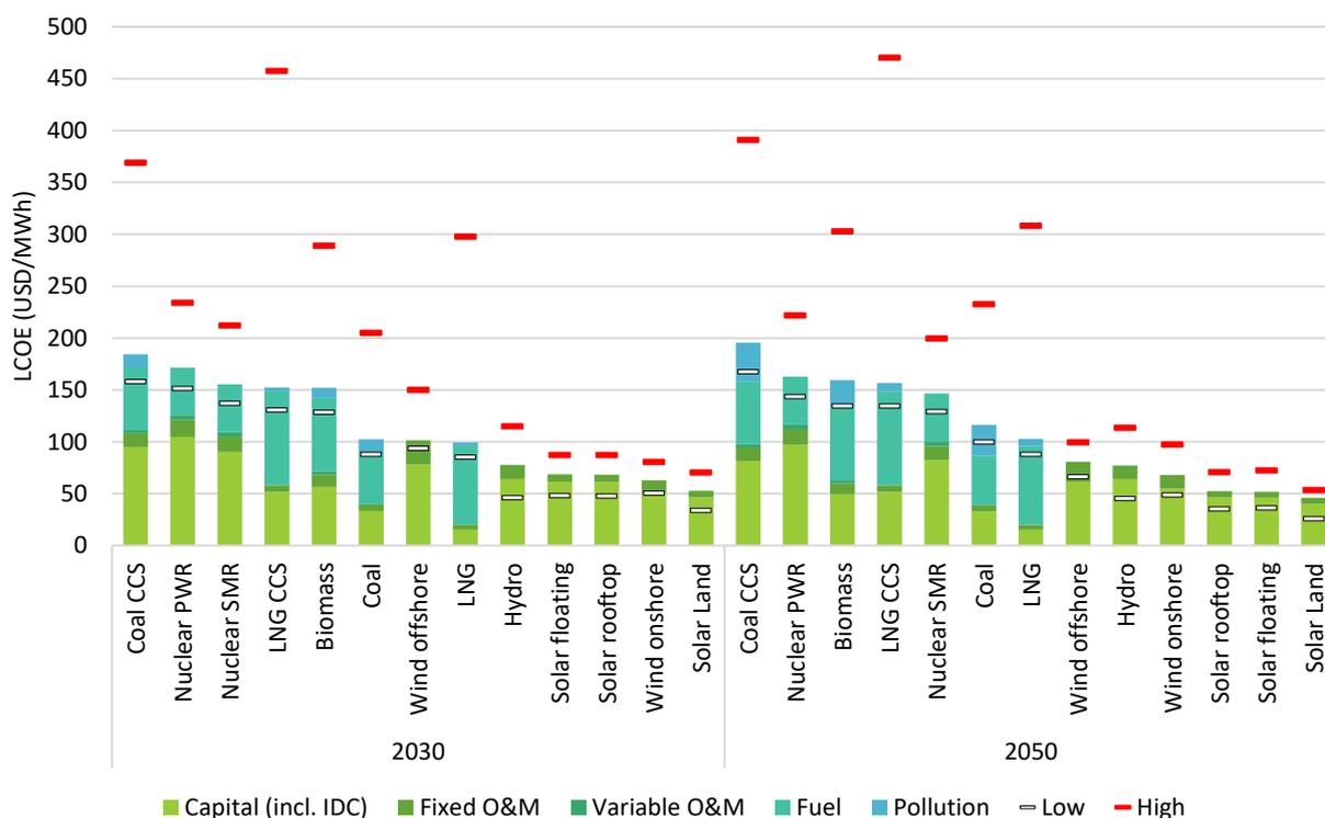
Figure 122: LCOE values for the various technologies. "Low" and "High" indicate the LCOE result with low and high FLH assumptions.
