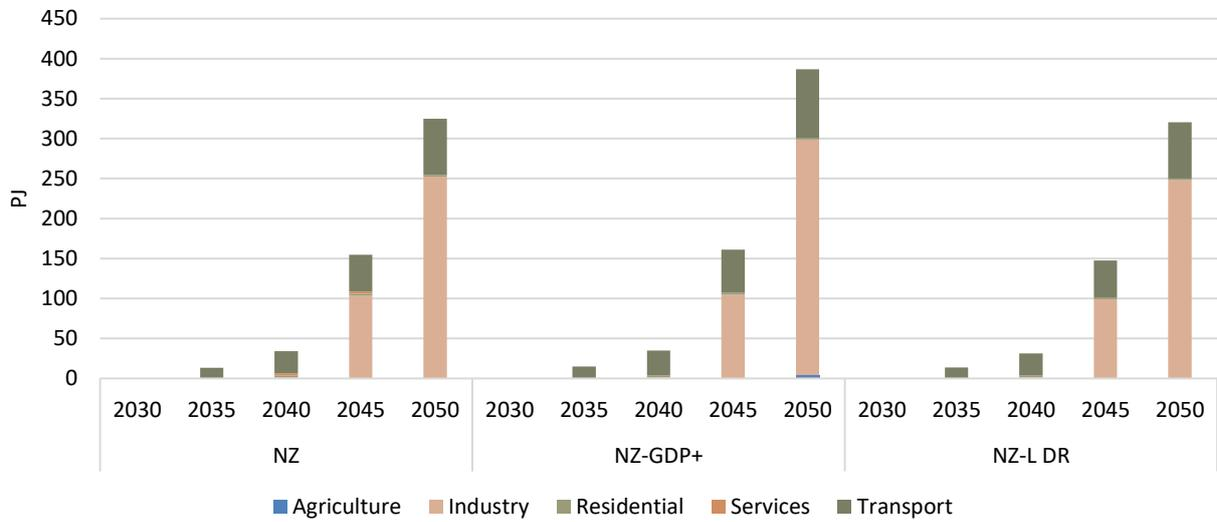
Figure 112: Final H<sub>2</sub> consumption by sector, TIMES [PJ]
