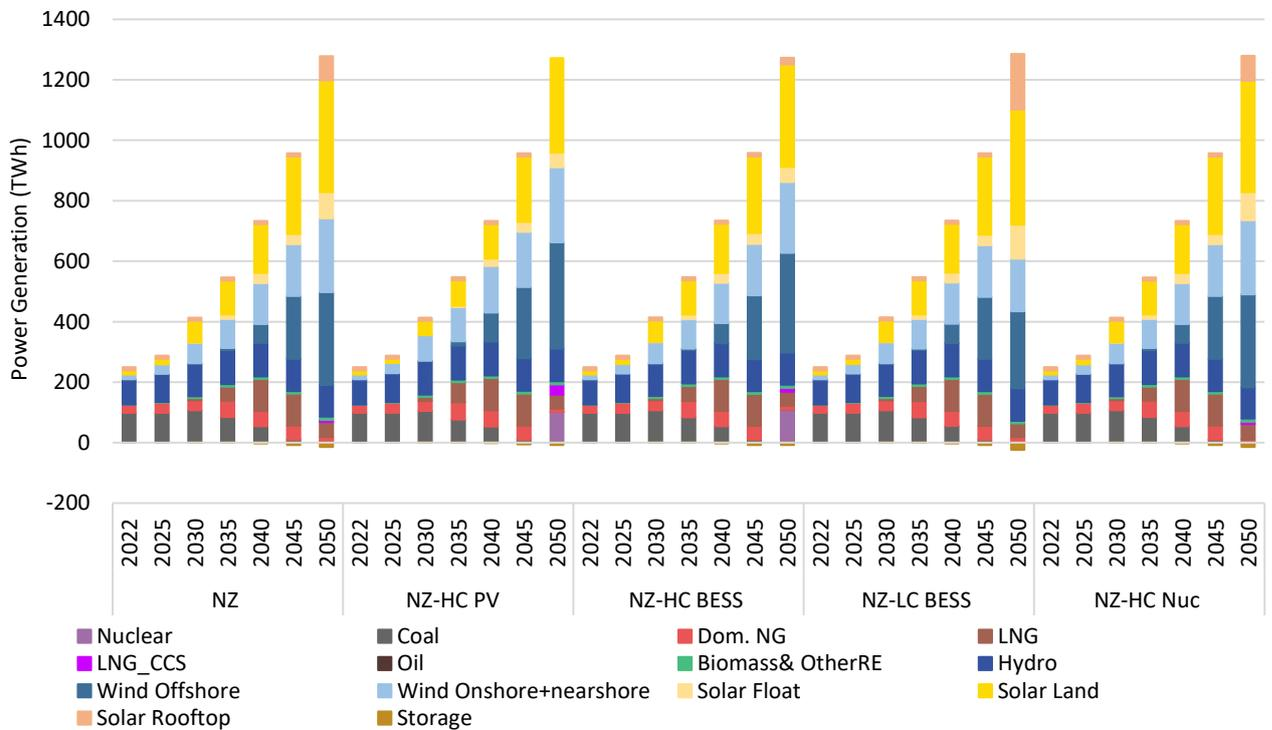
Figure 105: The generation of technology cost sensitivity scenarios comparing with the NZ scenario. Fixed import from neighbouring countries is not included in the figure.
