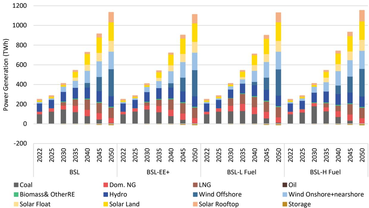
Figure 99: The power generation of BSL sensitivity scenarios comparing with BSL scenario. Fixed import from neighbouring countries is not included in the figure.
