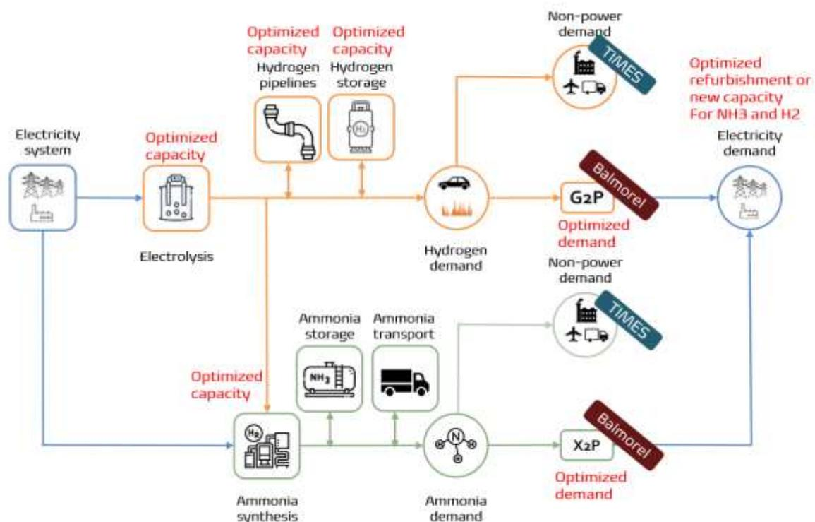
Figure 4: Schematic representation of how the Power-to-X modelling works between TIMES and Balmorel. The models (TIMES or Balmorel) responsible for determining the different types of hydrogen and ammonia demand is indicated.
