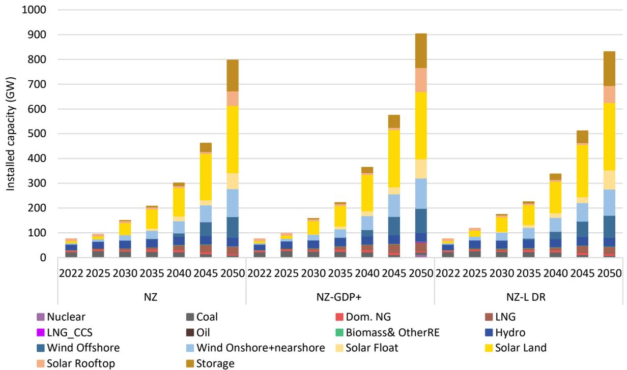
Figure 94: The installed capacity of NZ-GDP+ and NZ-L DR scenarios comparing with NZ scenario. Fixed import from neighbouring countries is not included in the figure.
