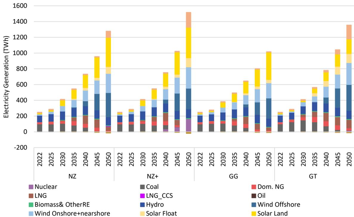
Figure 86: The electricity generation of main variation scenarios comparing with the NZ scenario. Fixed import from neighbouring countries is not included in the figure.
