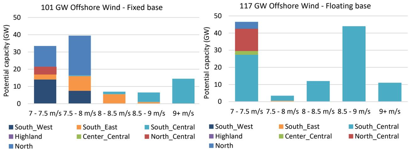
Figure 25: Offshore wind potential implemented in Balmore (218 GW - Potential of offshore wind with distance to the shore below 150 km, more than 6 nautical miles from shore, outside the maritime channel, average wind speed is higher 7 m/s at height 100 m)
