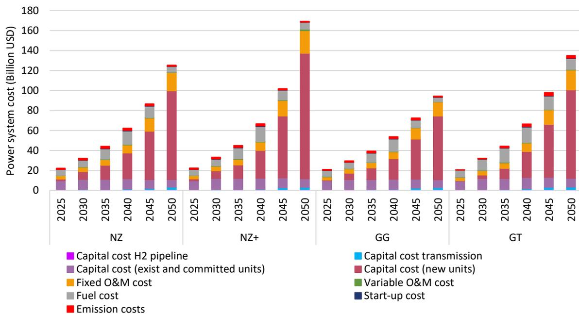
Figure 89: Power system cost of main variation scenarios comparing with the NZ scenario.
