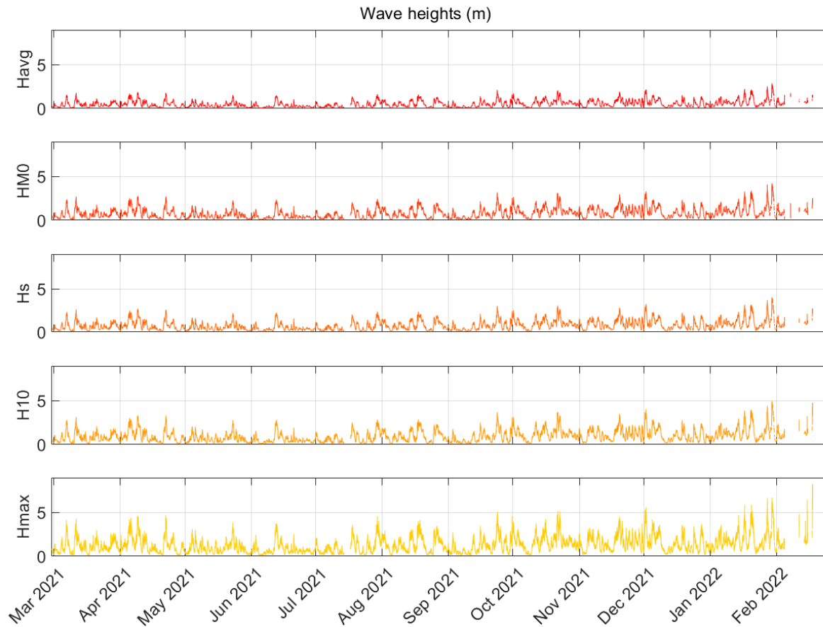
Figure 180. Time series of wave heights. The panels from top to bottom present: average wave height, spectral significant wave height, significant wave height, average height of the highest 1/10 th of all waves, and maximum wave height.
