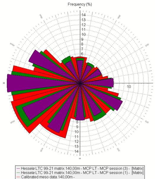
Figure 36. Directional distribution of the three long term wind models. Green: Primary model, red: Calibrated mesoscale model, purple: Translated Læsø data.
