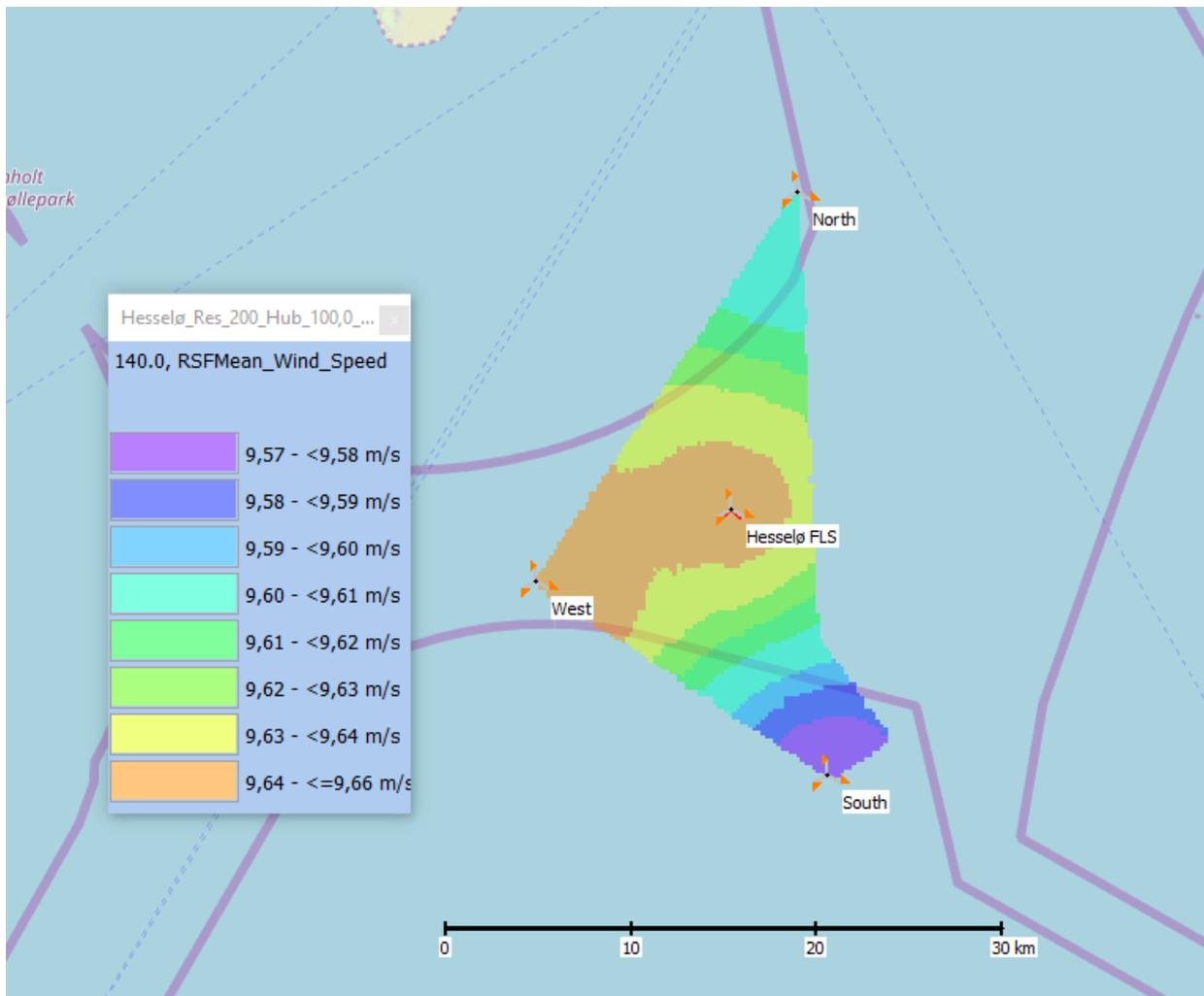
Figure 37. Wind resource map for Hesselø offshore wind farm zone. Wind speeds are Weibull derived mean wind speeds.
