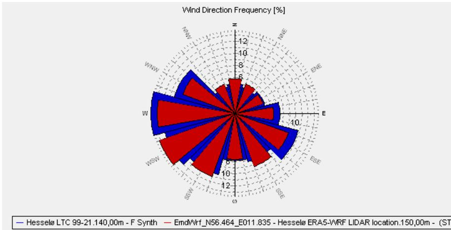
Figure 34. Directional distribution of translated Læsø data at 140 m (blue) and EMD-WRF (Hesselø FLS) (red), concurrent period.
