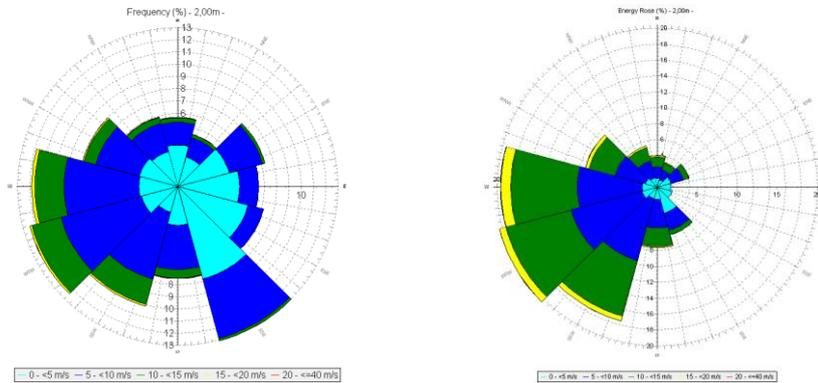
Figure 22. Wind direction frequency (on the left) and energy (on the right) distribution, Väderö 26 years (2005-2021)
