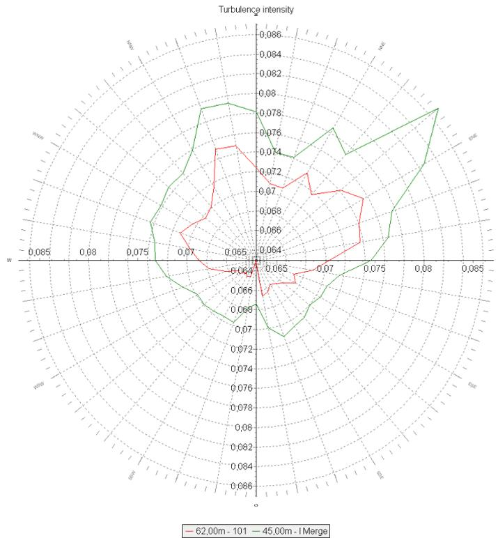
Figure 9. Turbulence intensity measured at Læsø mast (4 years) at 62 and 45 m per wind direction (36 sectors)
