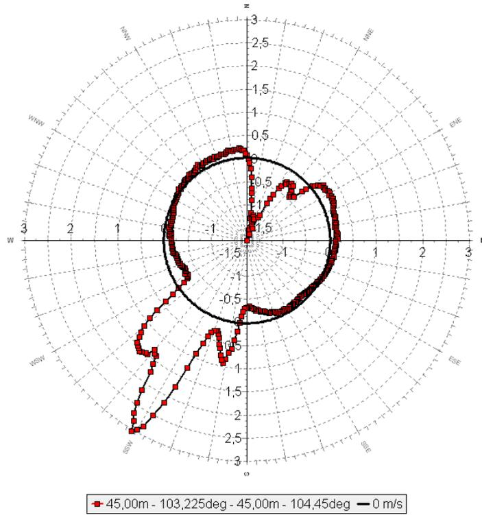
Figure 6. Wind speed difference between 45 m SV and 45 m NE, binned by direction at Læsø
