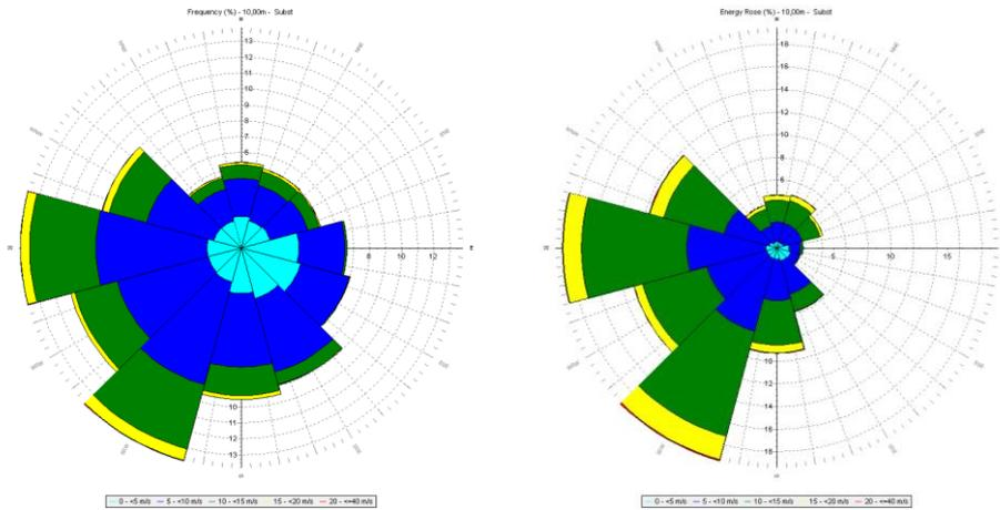
Figure 15. Wind direction frequency (on the left) and energy (on the right) distribution, Anholt 22 years (11/1999-11/2021)
