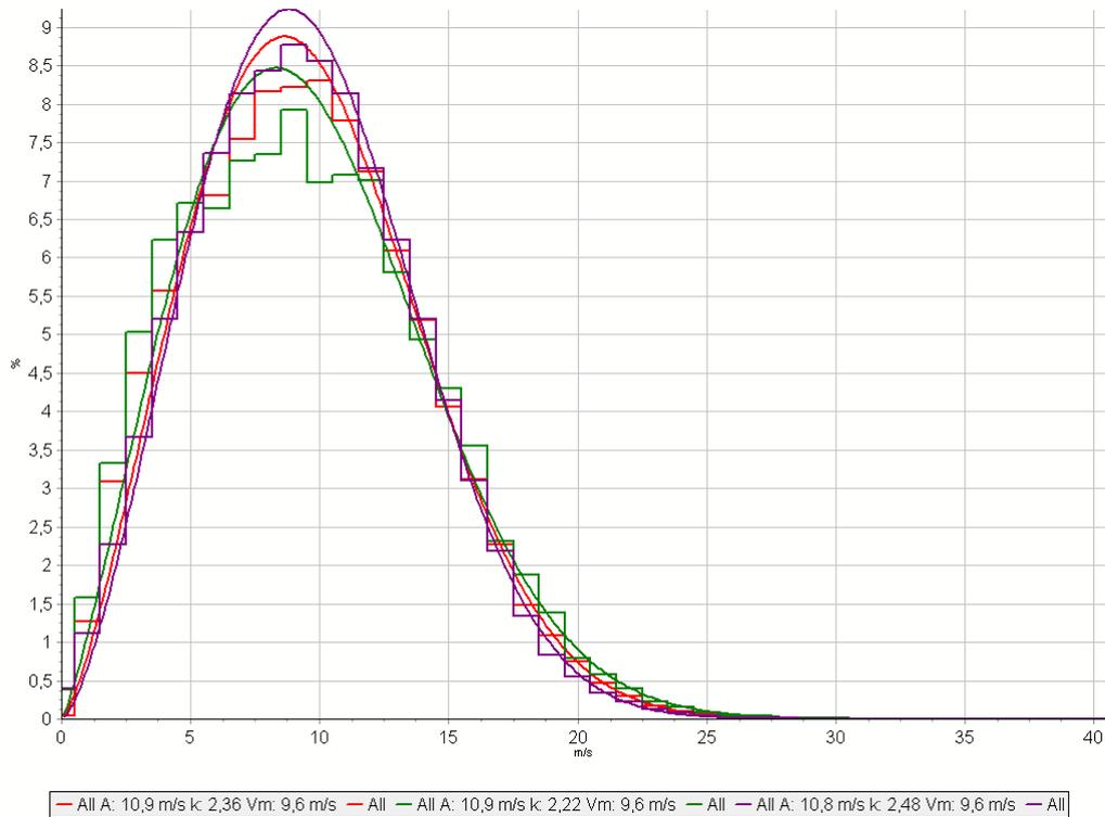
Figure 35. Wind speed probability function for the three datasets. Primary model (green) has a poor fit to a Weibull distribution compared to the calibrated mesoscale model (red) and the translated Læsø data (purple).
