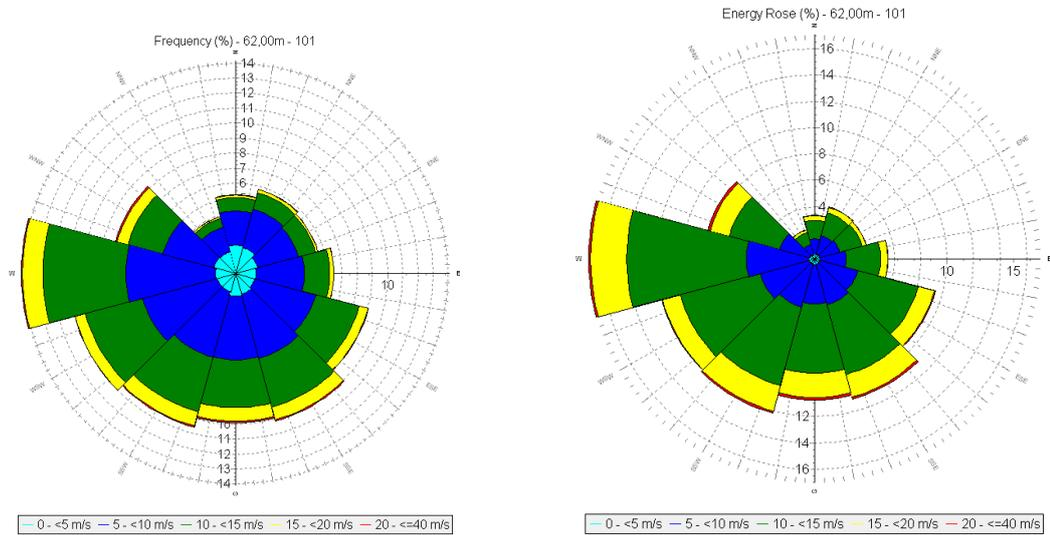
Figure 7. Wind direction frequency (on the left) and energy (on the right) distribution, Læsø 4 years, at 62 m ASL (07/1999-07/2003)
