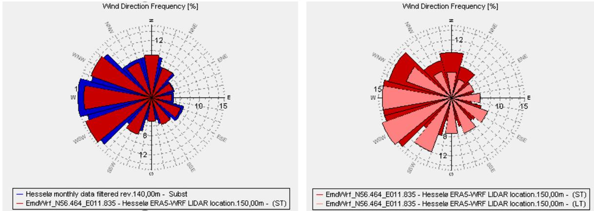
Figure 27. Left: Wind direction roses for the concurrent period of LIDAR (blue) and EMD-WRF (red) data. Right: Wind direction roses for EMD-WRF data. Deep red represents the entire long-term period, light red represents the period concurrent with LIDAR measurements.
