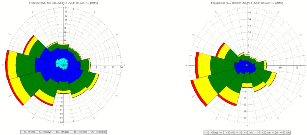
Figure 28. Left: wind direction distribution of long term corrected LIDAR data at 140 m. Right: Energy distribution of long term corrected LIDAR data at 140 m. Both are divided in wind speed intervals.
