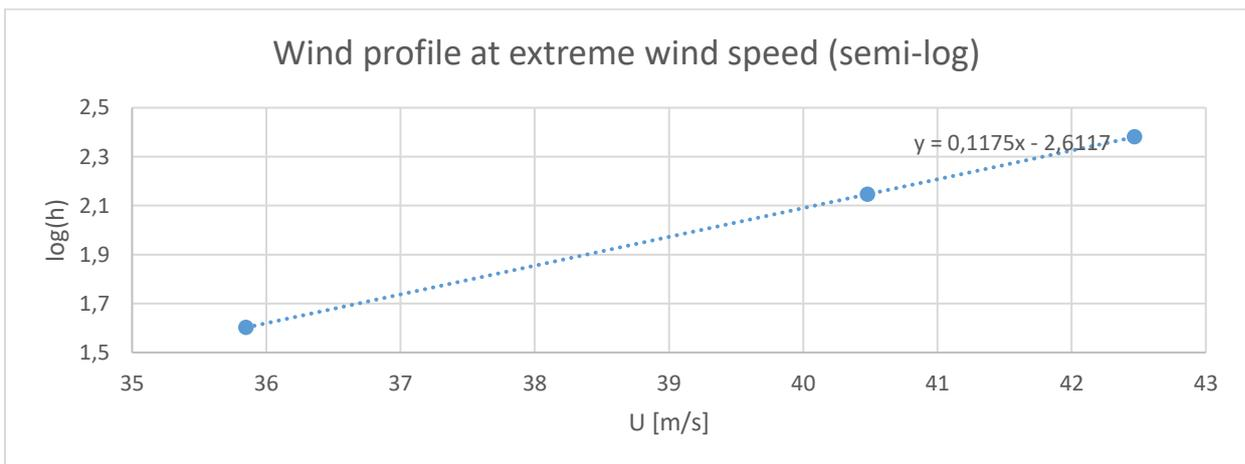
Figure 43. Fit on extreme wind speed to obtain roughness length at high wind speeds.
