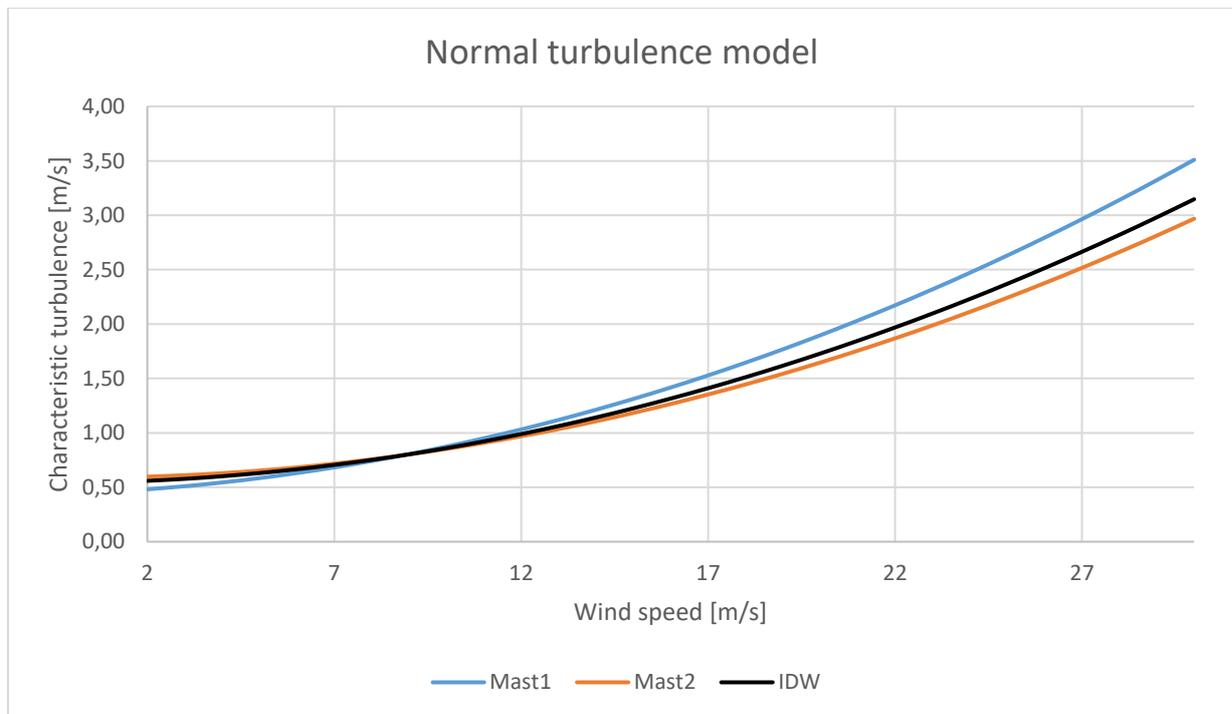
Figure 39. Characteristic turbulence at the two masts along with the inverse distance weighted (IDW) model recommended at the site.
