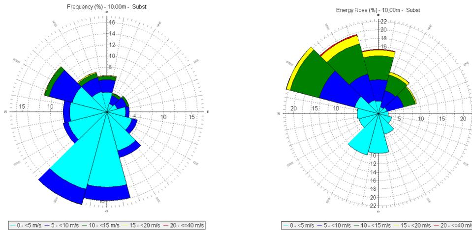
Figure 20. Wind direction frequency (on the left) and energy (on the right) distribution, Nakkehoved 14 years (11/2007-11/2021)
