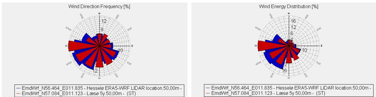
Figure 33. Left: directional distribution between EMD-WRF at Læsø (red) and EMD-WRF at Hesselø FLS (blue). Right: Energy rose of same two datasets.
