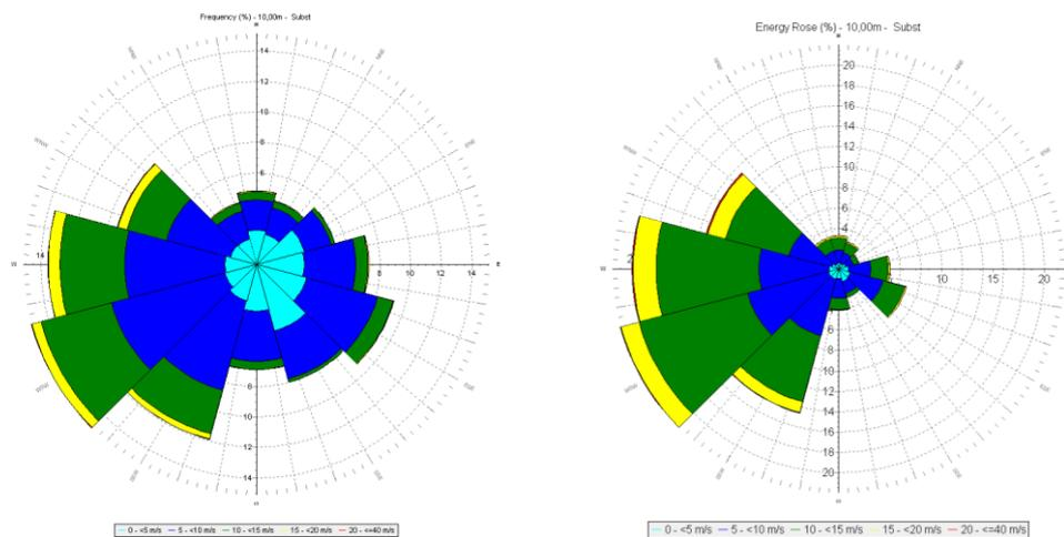
Figure 18. Wind direction frequency (on the left) and energy (on the right) distribution, Griben 19 years (11/2002-11/2021)
