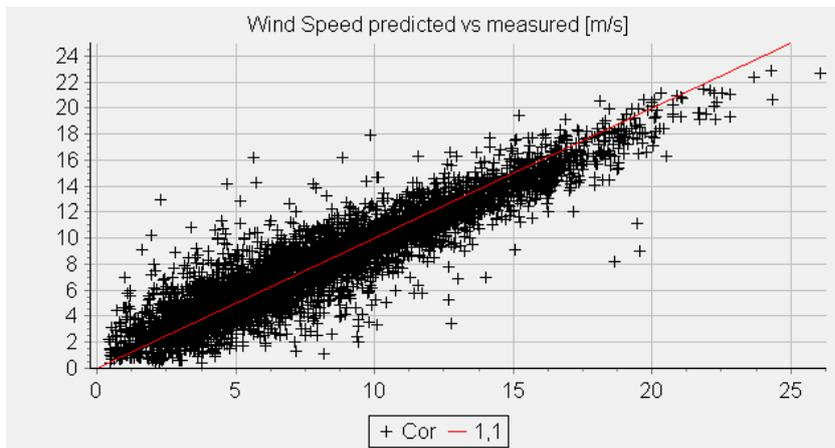
Figure 31. Linear fit of EMD-WRF 140 m to FLS 140 m data.
