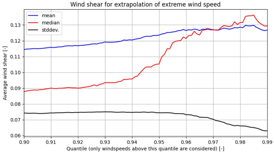
Figure 41. Wind shear extrapolation of extreme wind speed at Hesselø FLS.
