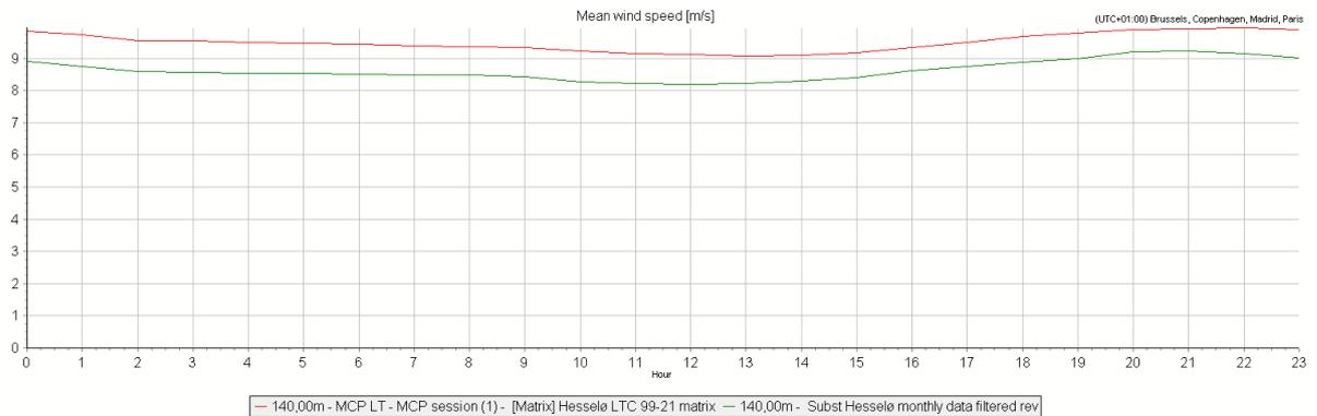
Figure 29. Diurnal wind speed, long-term corrected (red) and observed (green).
