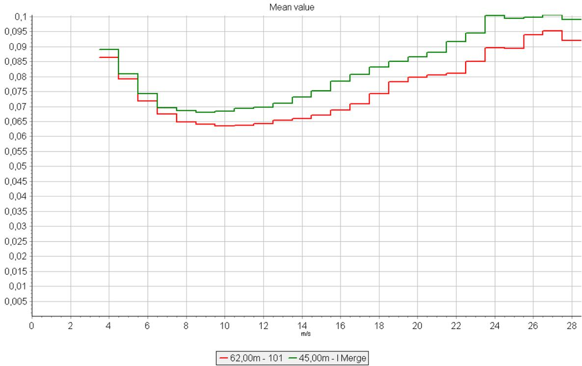
Figure 8. Turbulence intensity measured at Læsø mast (4 years) at 62 and 45 m per wind speed bin
