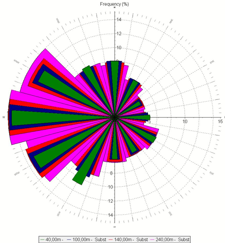
Figure 4. Directional distribution at selected heights of LIDAR measurements.
