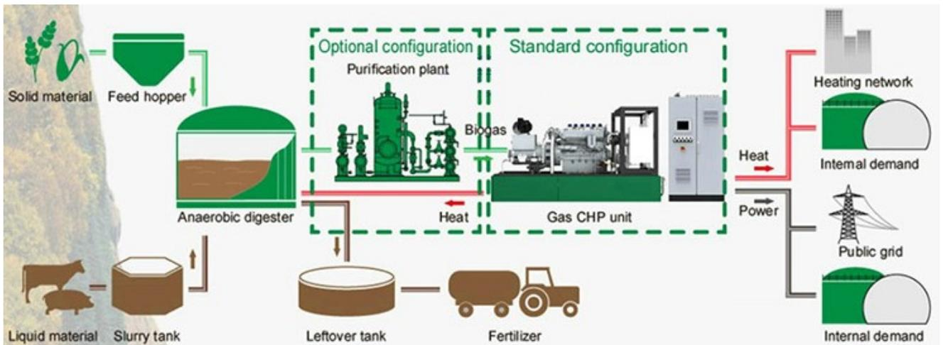
Figure 88: Biogas CHP working diagram (ref. 5).
