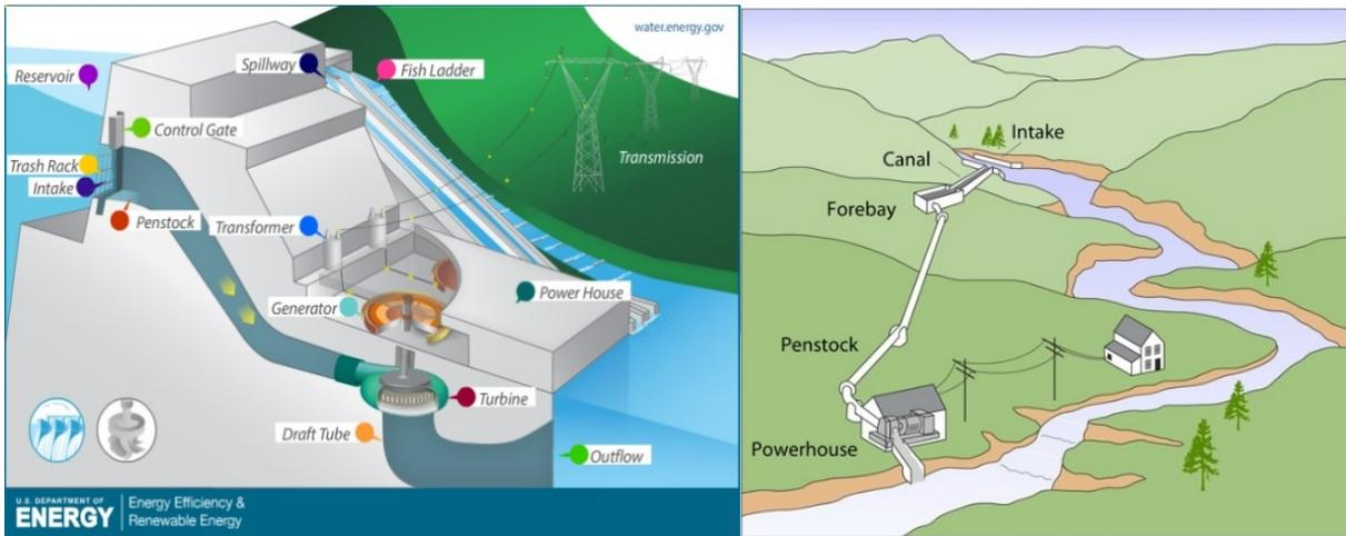
Figure 30: Reservoir and run-of-river hydropower plants (ref. 14)
