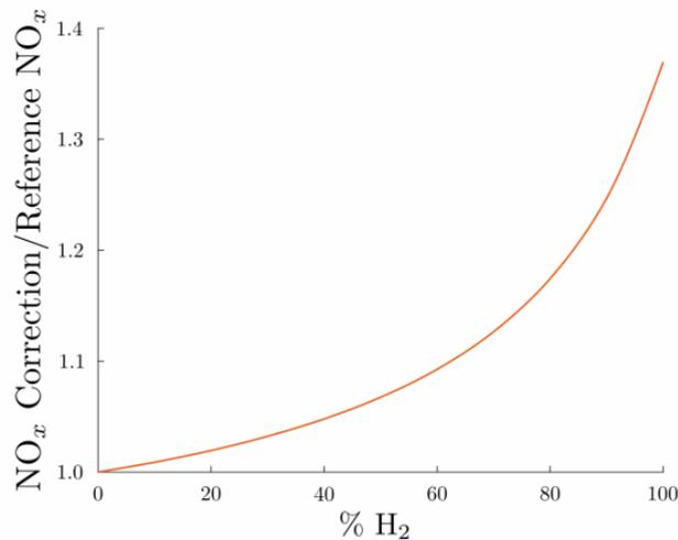
Figure 21. Increase of NO<sub>x</sub> emission correspond to the H<sub>2</sub> co-firing ratio according to [Ref. 9]
