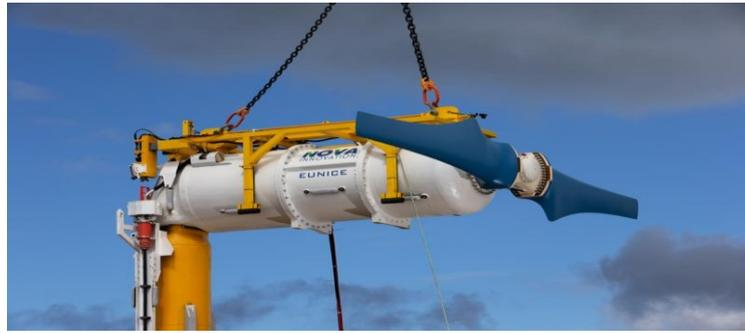
Figure 67: 500 kW direct drive turbine [16]
