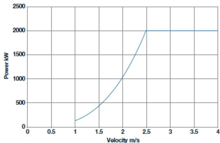
Figure 65: Sample power curve for tidal stream turbine.[9]
