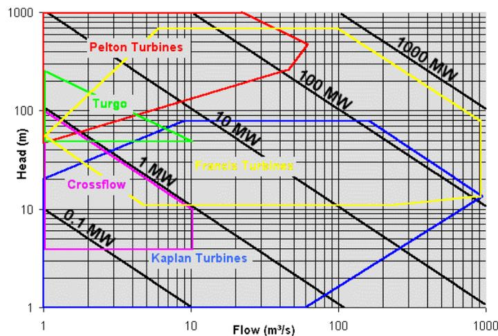
Figure 32: Hydropower turbine application chart (ref. 2)
