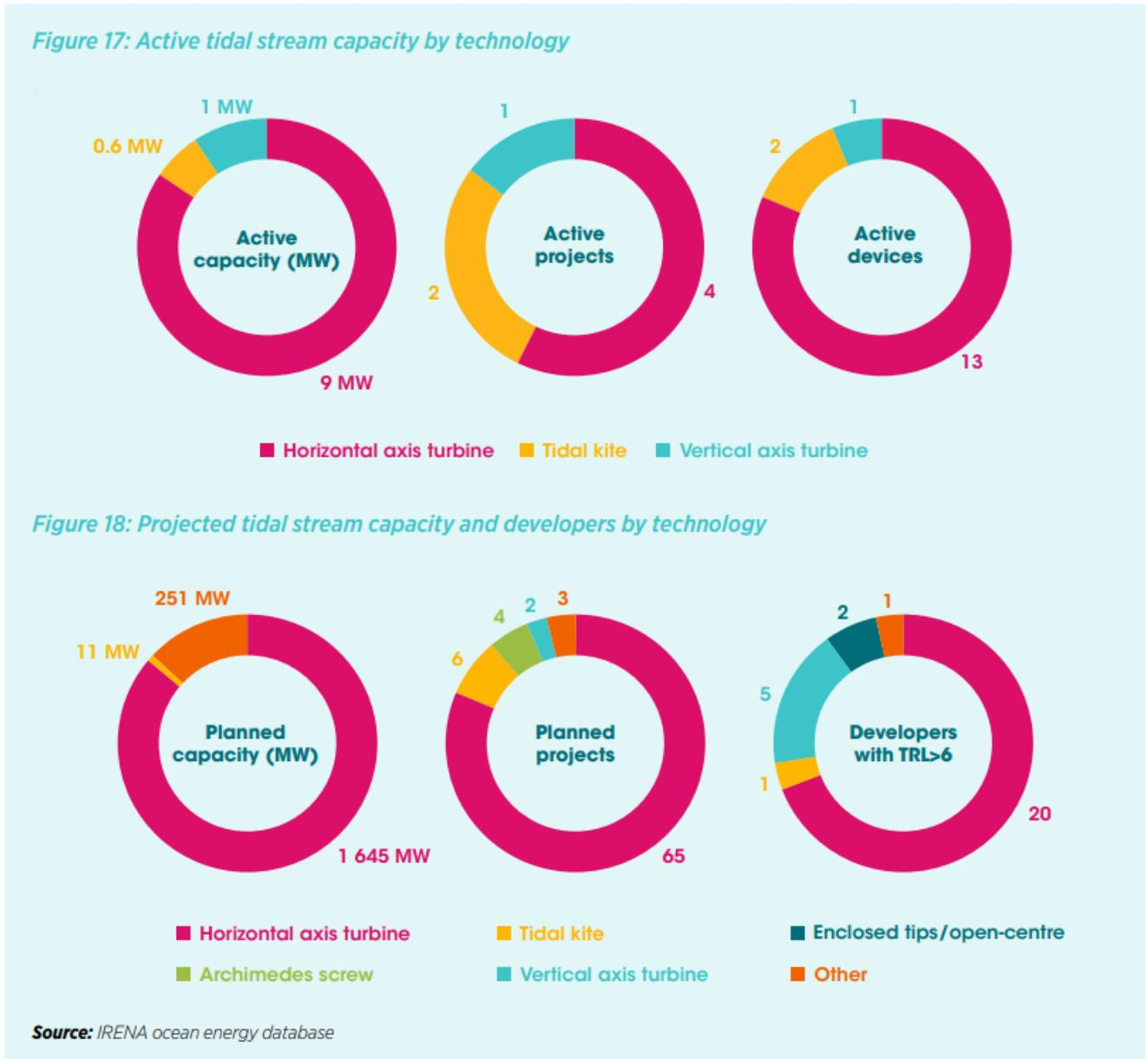
Figure 61: Active and project tidal stream capacity and technology [26]
