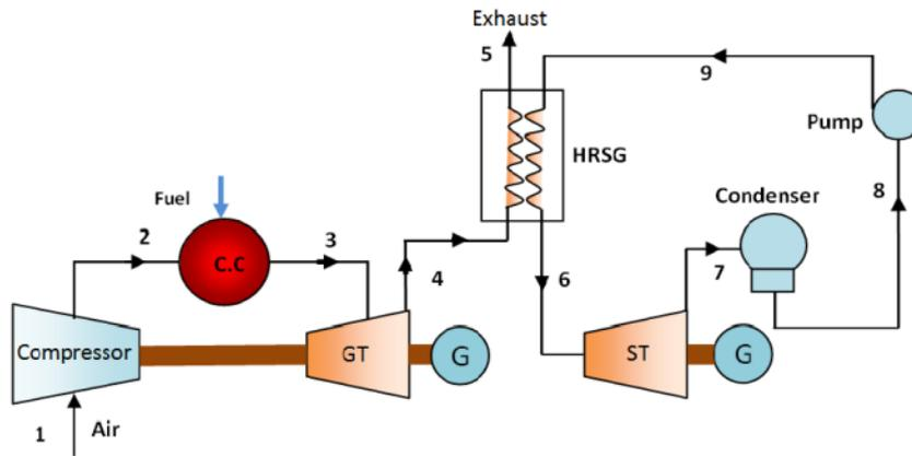
Figure 166: Process diagram of a CCGT (ref. 1)
