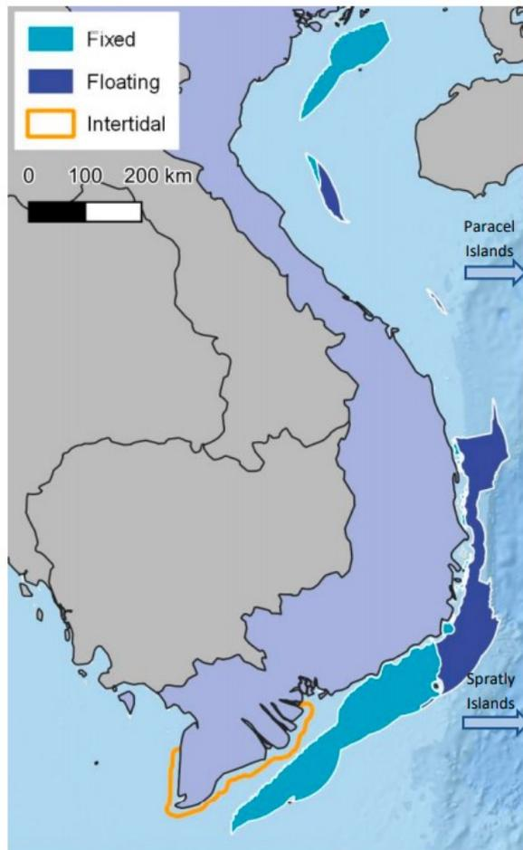
*Figure 51. Potential sites for offshore wind turbines (Ref. 35). The potential for offshore wind is mainly along the coast of mainland Viet Nam and the Paracel and Spratly Islands are therefore not included in the map.*
