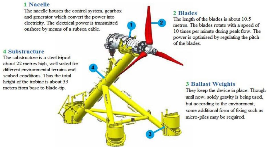
Figure 62: Early gravity based substructure design [8]
