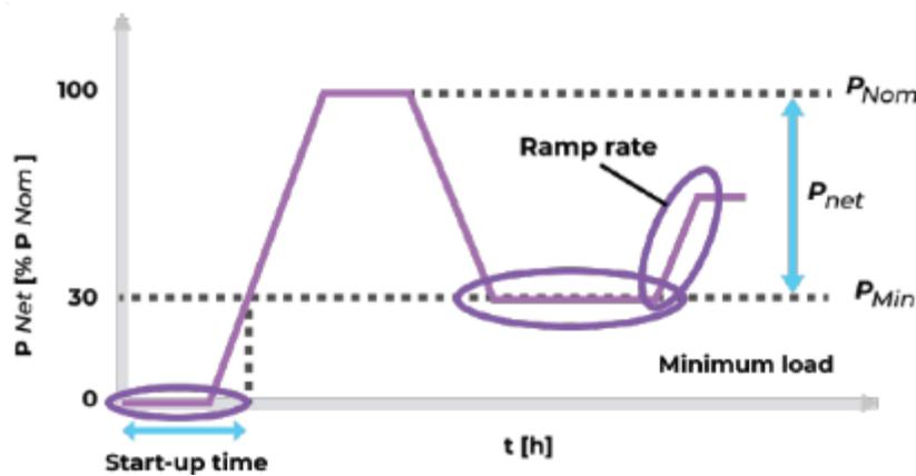
Figure 3: Key flexibility parameters of a power plant [3].
