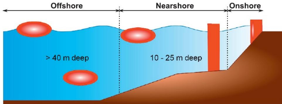
Figure 72: Location of wave energy converters [3]
