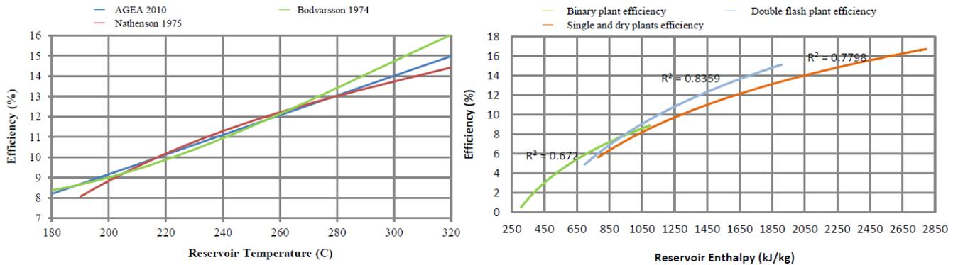
Figure 92: Geothermal plant efficiency as a function of temperature and enthalpy (ref. 5)
