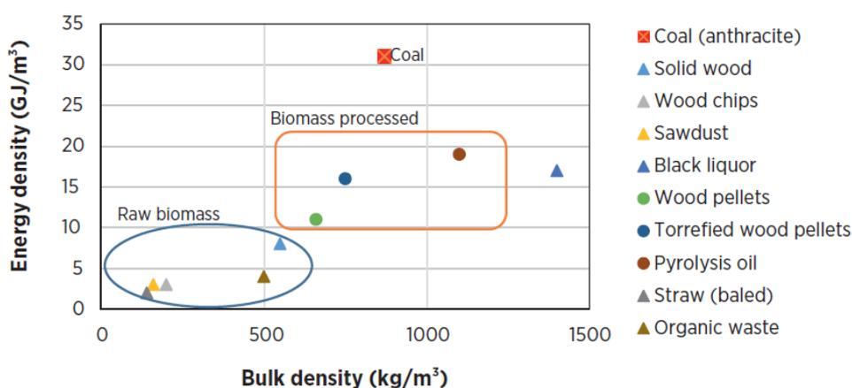
Figure 83: Energy density of biomass and coal (ref. 11).
