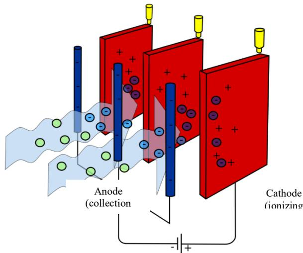
Figure 4: Principle behind electrostatic precipitator (ref.4).
