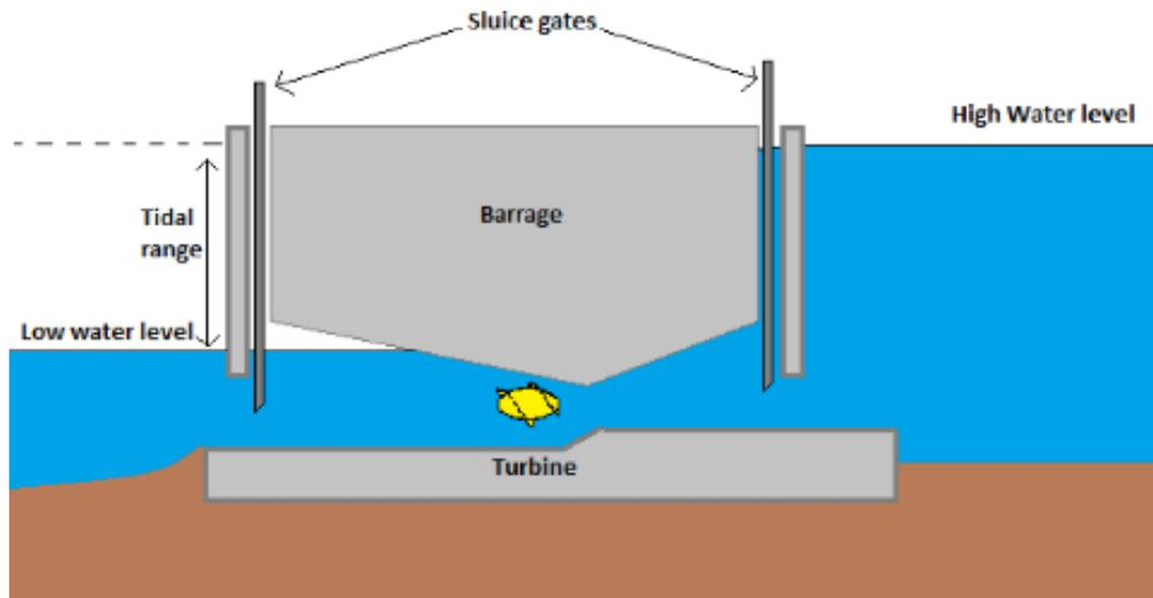
Figure 58: Schematic of tidal impoundment type plant.[4]
