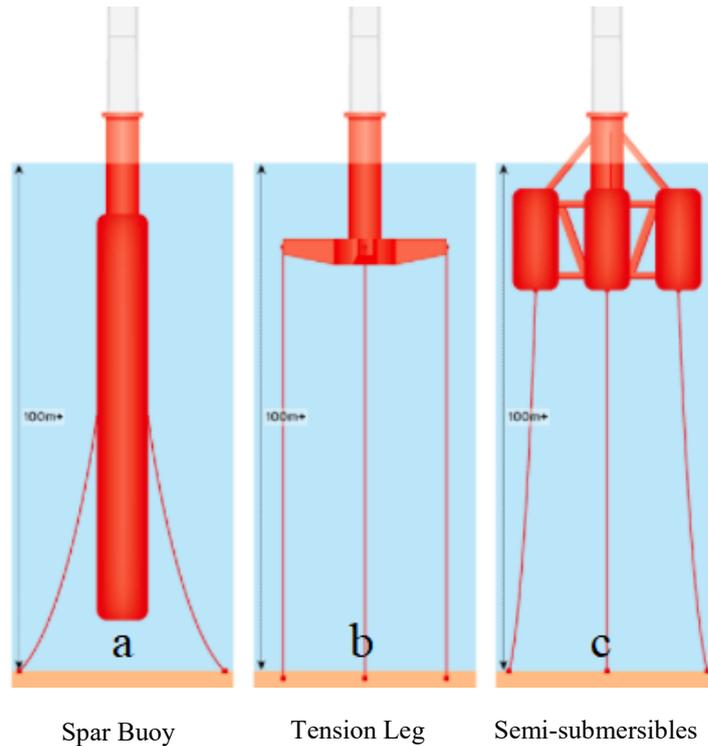
Figure 53. Different floating offshore foundations (Ref. 29).
