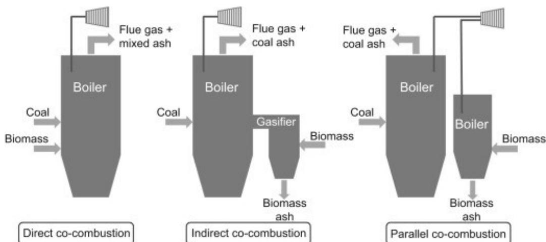
Figure 82: Different biomass co-firing configurations (ref. 15)
