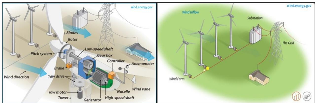
Figure 46: General turbine technology and electrical system (ref. 48)
