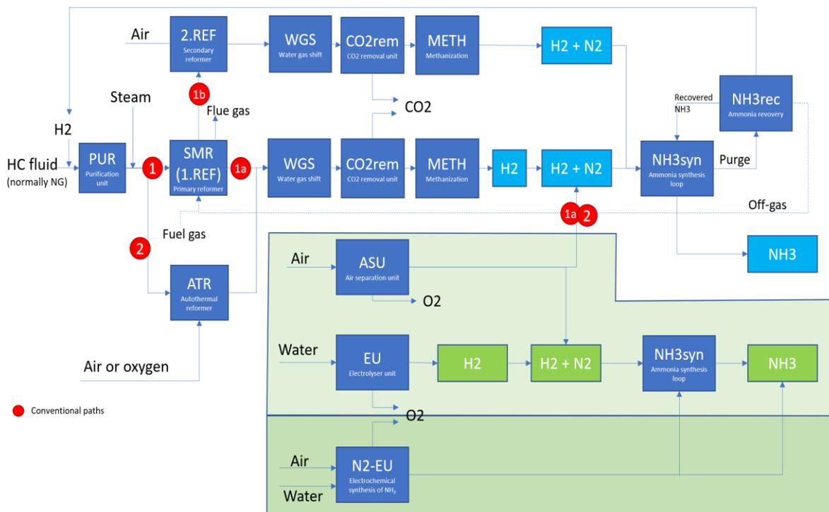
Figure 40: Different pathways for production of NH<sub>3</sub>. The light green area is the green NH<sub>3</sub> production part that is covered within this Technology Catalogue. The darker green area marks a potential future route (electrochemical). The white background shows the three conventional parts, i.e. 1a) SMR+ASU, 1b) SMR+2.REF and 2) ATR+ASU
