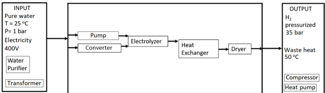
Figure 39: A sketch of an electrolysis system for AEC and PEMEC.
