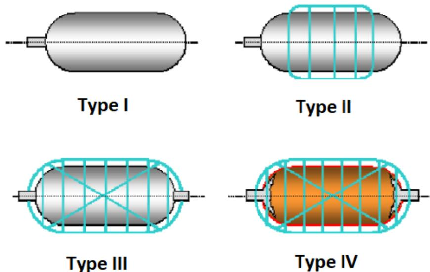
*Figure 14: Schematic of different hydrogen pressure tank types [18]. The blue lines represent fibers used for wrapping, made of different materials depending on the tank type. More details in the text below.*
