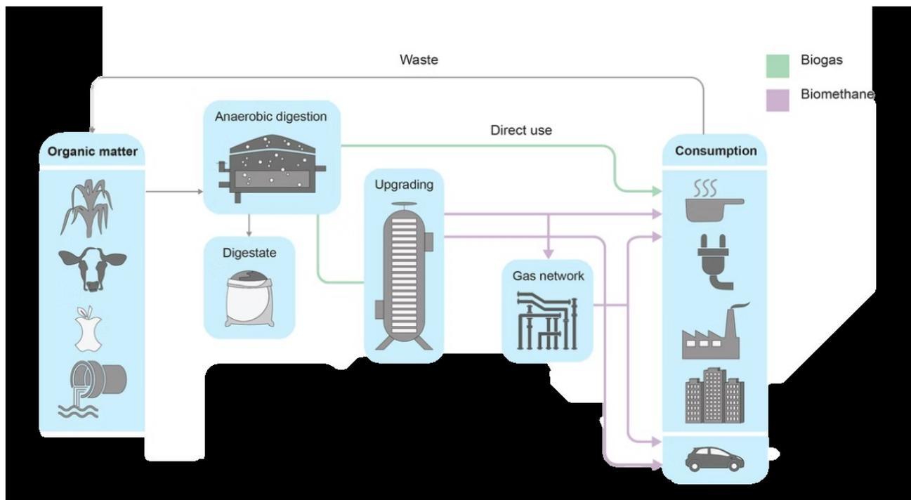
Figure 68: Biogas may either be used directly as an energy source or be upgraded through an upgrading plant to be fed into the gas network or be directly applied for consumptions needing gas with high energy content. Illustration from IEA [8]
