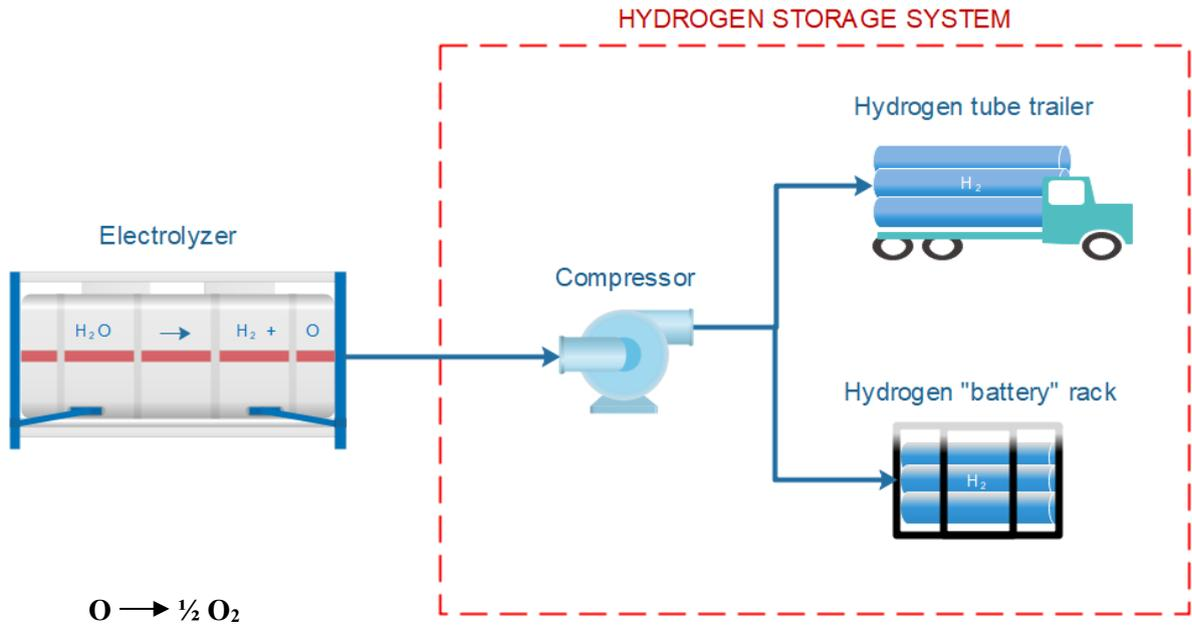
Figure 15: Typical pressurized tank storage system
