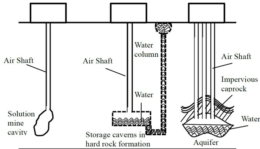
Figure 21: Various Geological Formations for Underground Storage [5]
