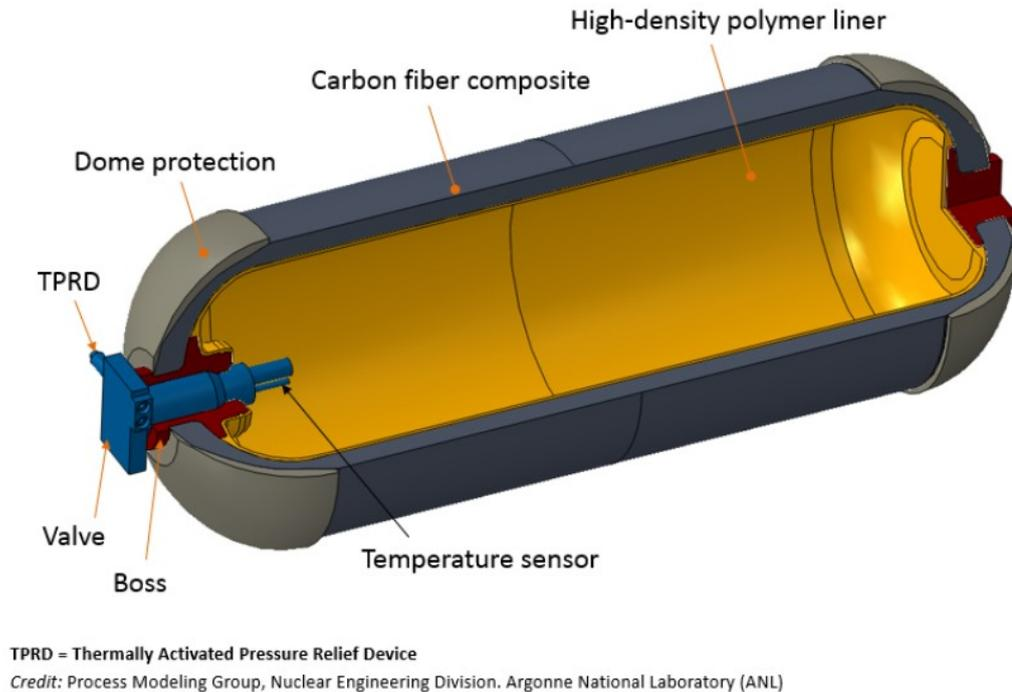
Figure 18: Components of a Type IV hydrogen pressure tank [36]
