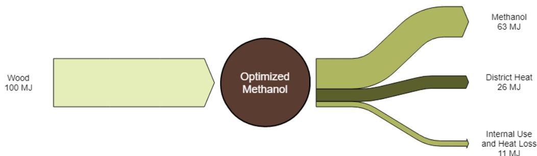
Figure 64: Optimized Biomass to Methanol Plant
