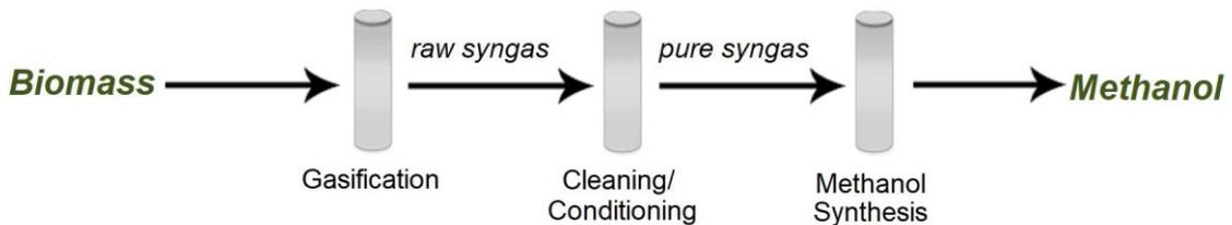
Figure 61: Biomass to Methanol Process
