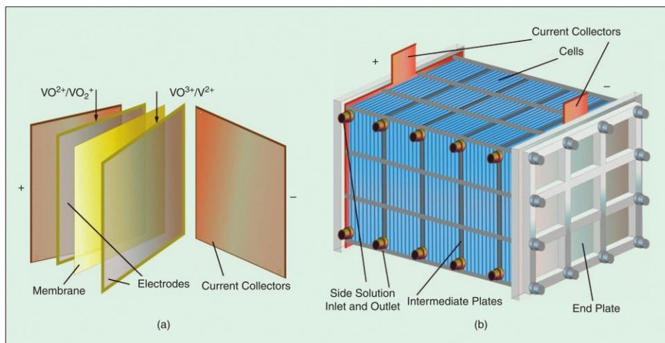
Figure 12: a) Reaction cell. B) Typical stack [2].
