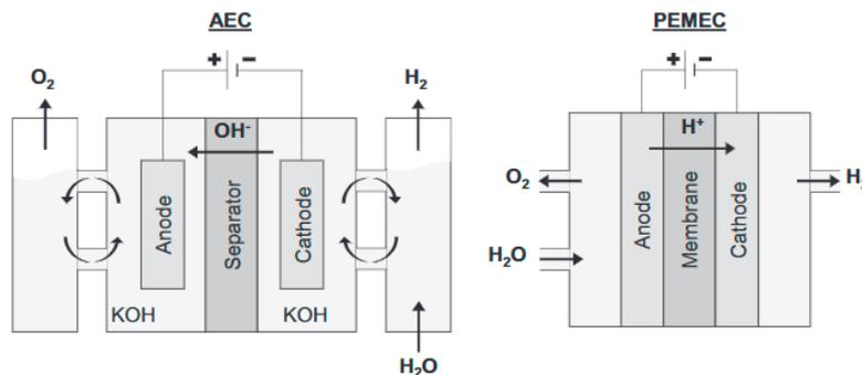
Figure 36: Operating principle of AEC and PEMEC [1].
