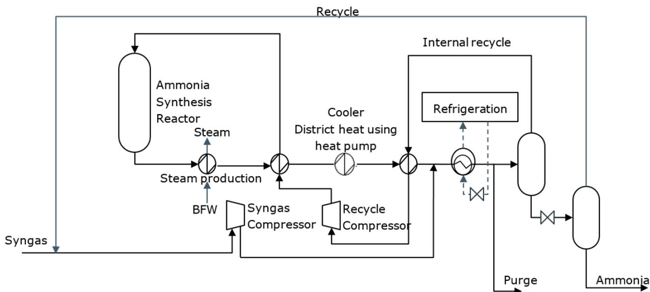
Figure 47: Ammonia synthesis loop and downstream purification
