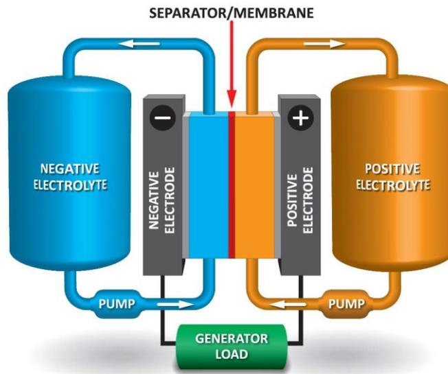
Figure 11: Schematic of flow battery [1].
