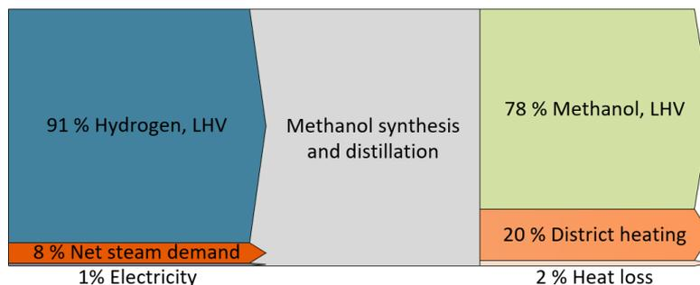
Figure 58: Energy balance of a methanol plant. “District heating” is low temperature heat that can be used for heating or low temperature industrial purposes.
