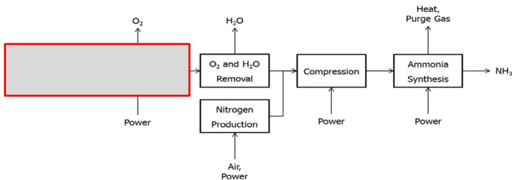
Figure 42: Green ammonia plant. Any impurities of O<sub>2</sub> in the H<sub>2</sub> product is removed by reacting it with H<sub>2</sub> over a DeOX (de-oxygenation unit).
