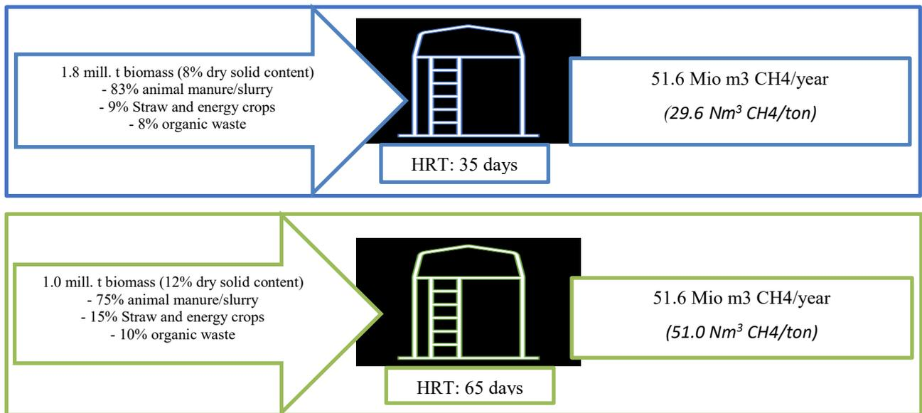
Figure 67: Biogas output in two different biogas plants – own illustration based on [19]
