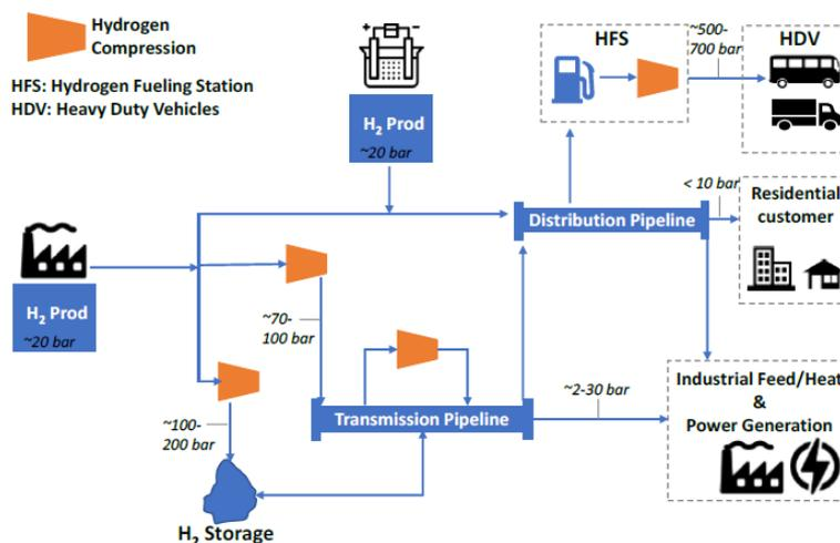
Figure 19. Possible future H<sub>2</sub> pipeline system [7].
