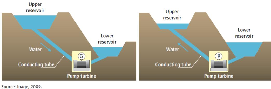
Figure 2: Pumped storage hydropower plants [2]
