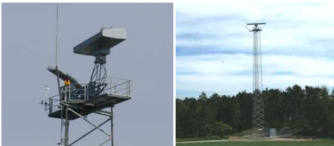
Figure 4-4 To the left is a Scanter 4000 radar, which is the type established in Thyborøn. To the right is a Scanter 2001 radar, which is established in Hanstholm and Oksbøl.
