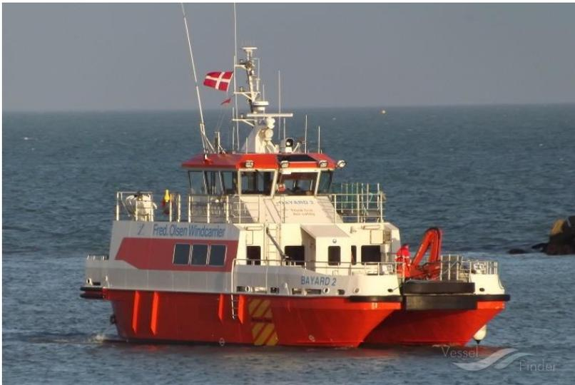
**Figure 3-13 Example CTV from the Lillgrund OWF; M/V Bringer is a 20 m multipurpose service vessel, designed for supporting offshore wind farms. The vessel has a capacity of 12 Pax + Crew.**
