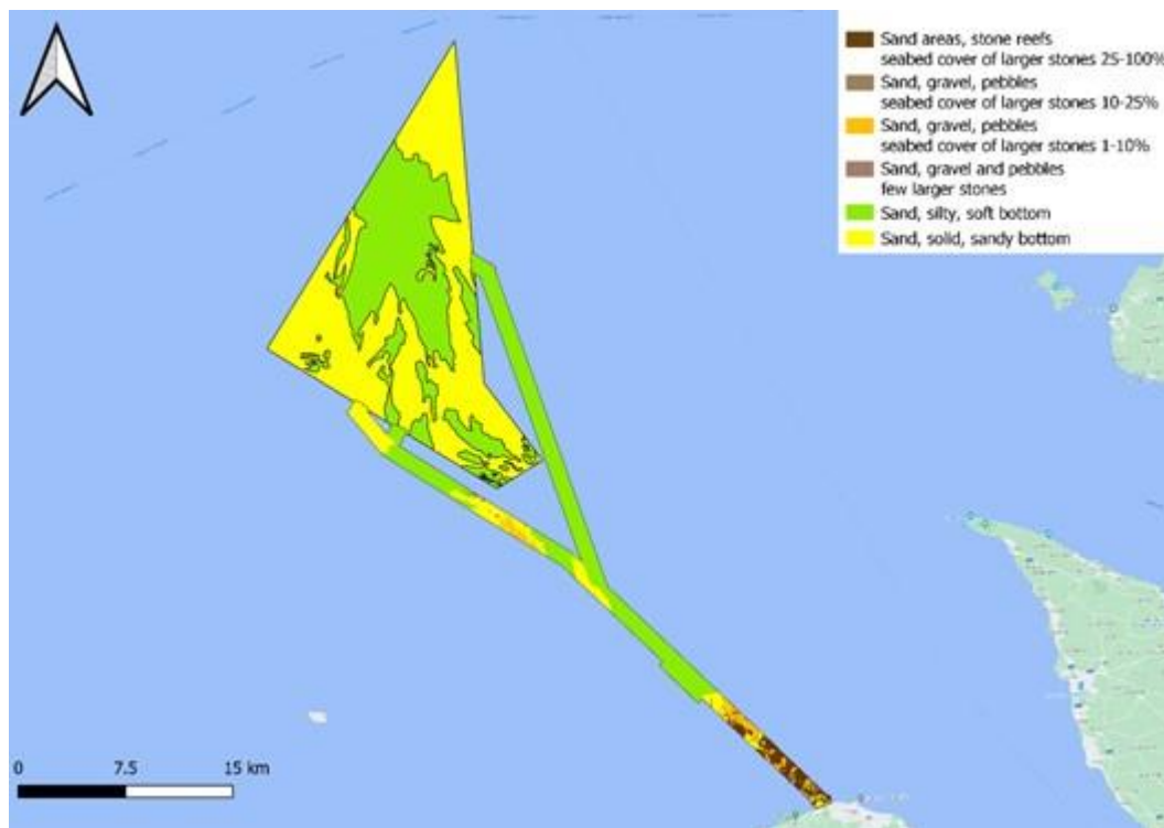
Figure 3.1 Seabed characteristic of the Hesselø Offshore Wind farm planned project area including the cable corridor to land.
