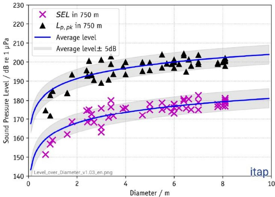
Figure 5.1: Relationship between measured SPL and SEL levels at 750 m distance, and pile size up to the largest pile diameter where data is available (Bellmann, et al., August 2020).
