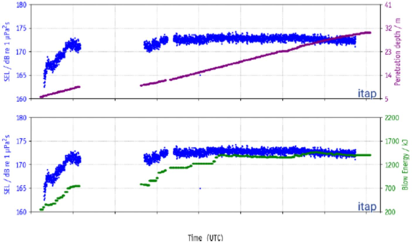
Figure 5.3: Relationship between SEL versus penetration depths and blow energy [Bellmann, et al., August 2020].
