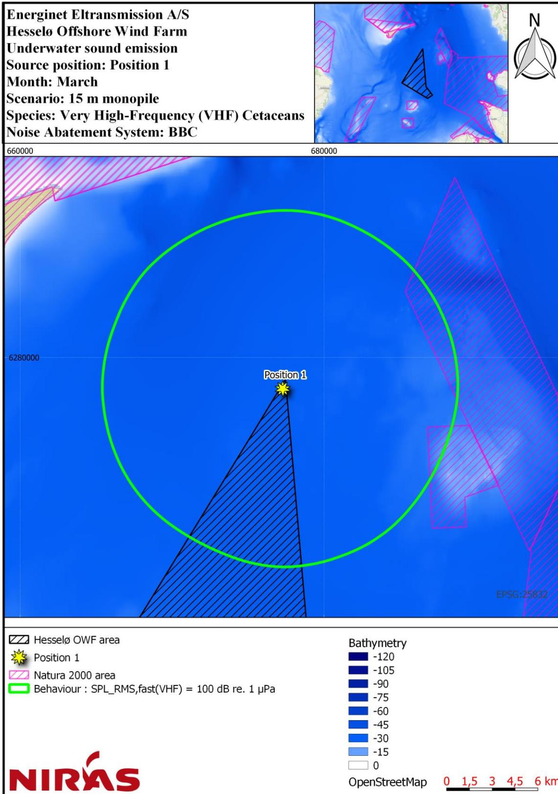
Figure 6.5: Noise contour map for position 1, showing impact distances for behaviour with VHF-weighting and BBC NAS on a 15 m monopile.
