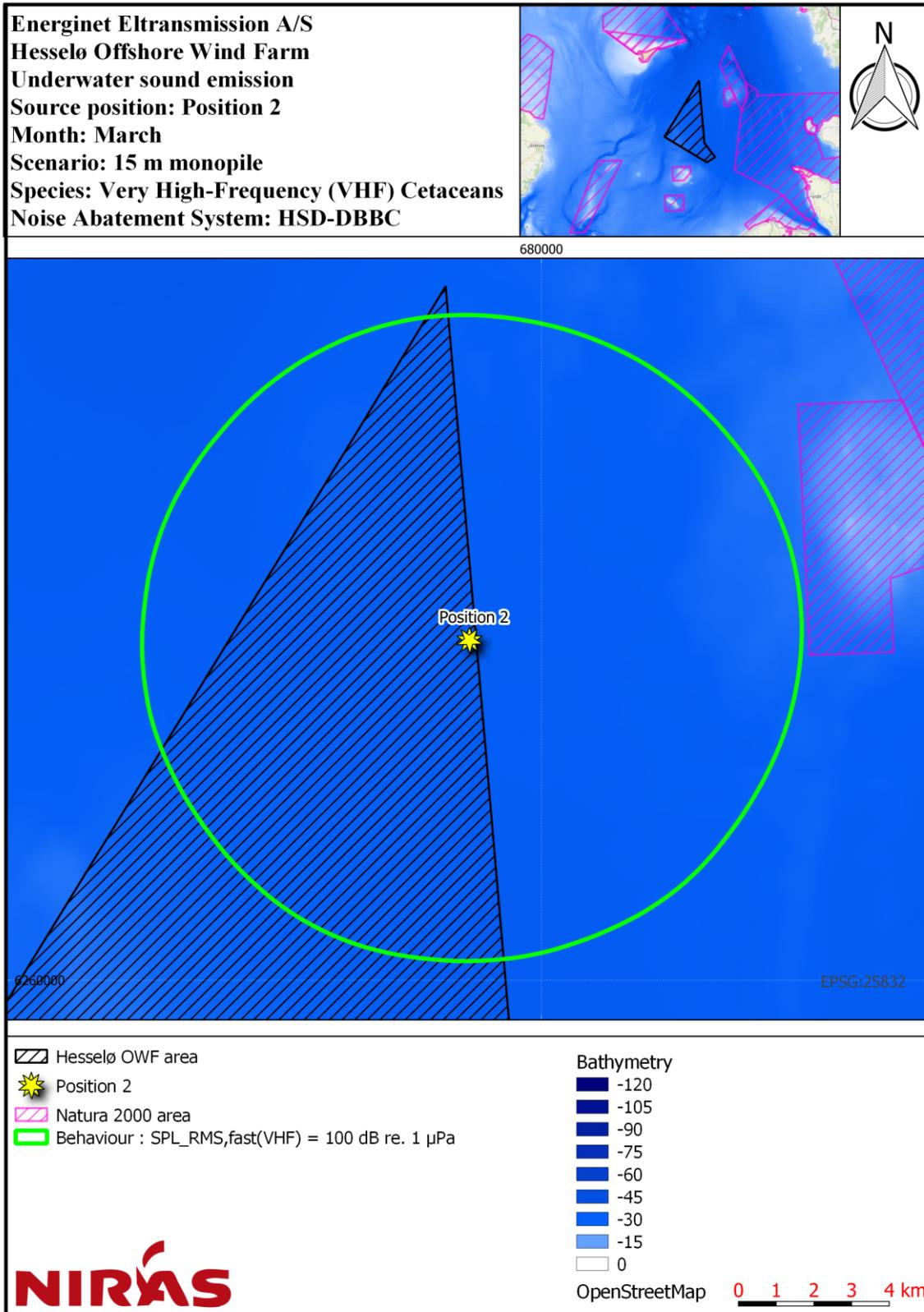
Figure 6.2: Noise contour map for position 2, showing impact distances for behaviour with VHF-weighting and HSD-DBBC NAS on a 15 m monopile.
