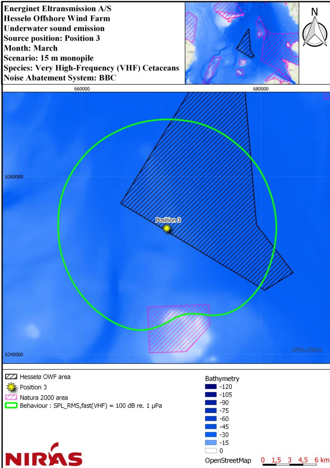
Figure 6.7: Noise contour map for position 3, showing impact distances for behaviour with VHF-weighting and BBC NAS on a 15 m monopile.
