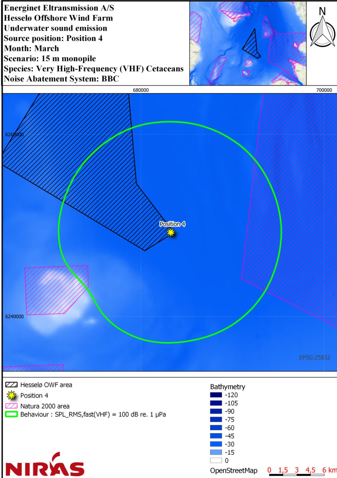
Figure 6.8: Noise contour map for position 4, showing impact distances for behaviour with VHF-weighting and BBC NAS on a 15 m monopile.
