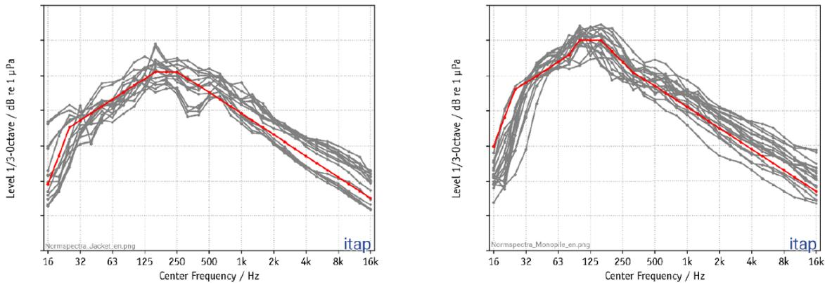
Figure 5.4: Measured pile driving frequency spectrum (grey lines) at 750m, with the averaged spectrum shown as the red line [Bellmann, et al., August 2020]. The spectrum ranges from 110-180 dB.
