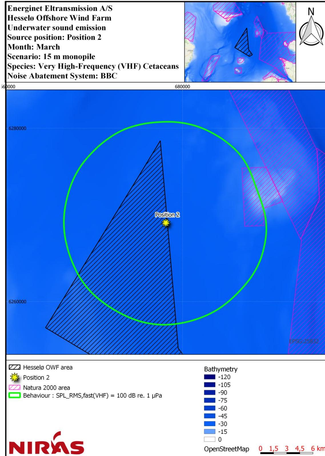
Figure 6.6: Noise contour map for position 2, showing impact distances for behaviour with VHF-weighting and BBC NAS on a 15 m monopile.
