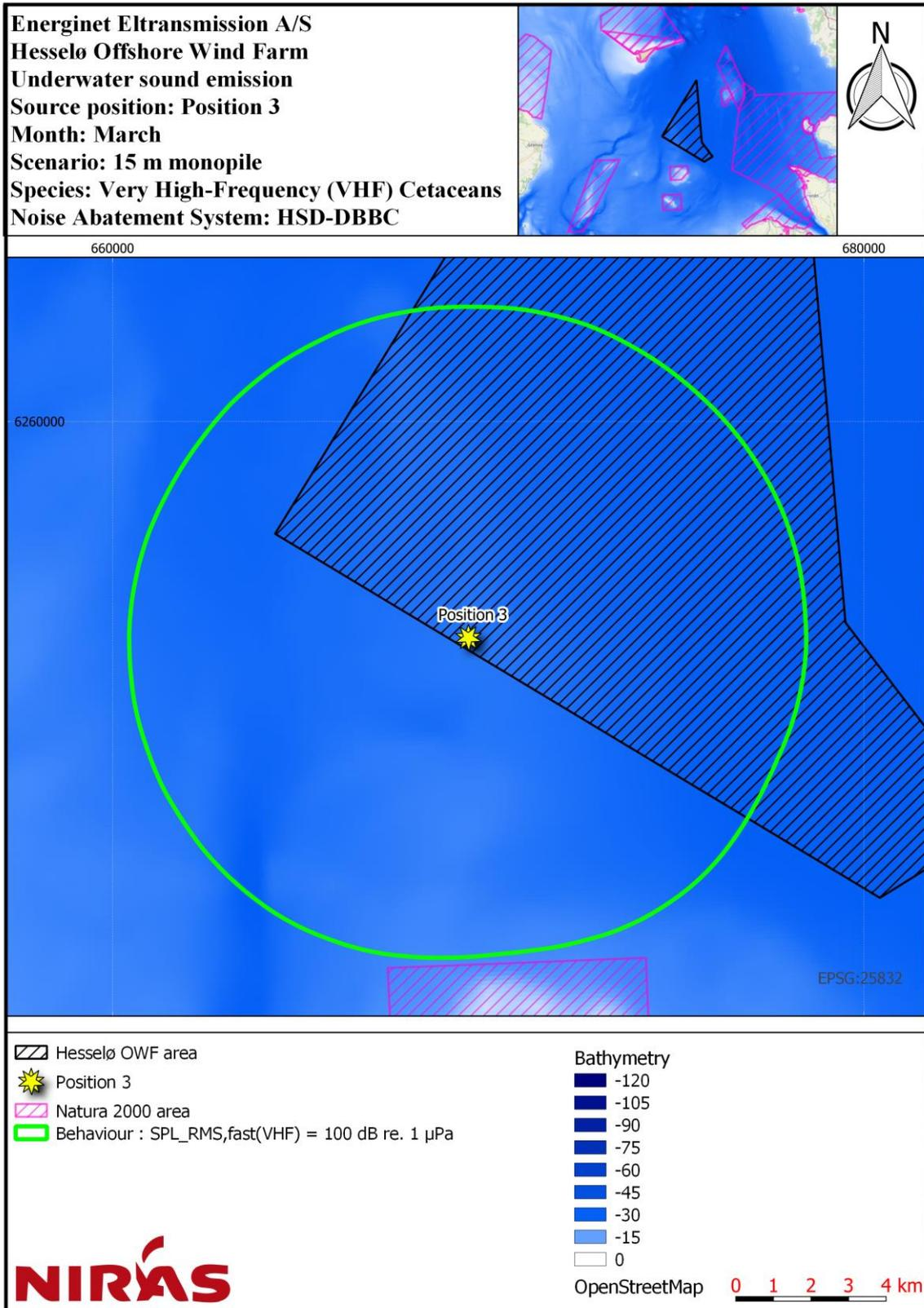
Figure 6.3: Noise contour map for position 3, showing impact distances for behaviour with VHF-weighting and HSD-DBBC NAS on a 15 m monopile.
