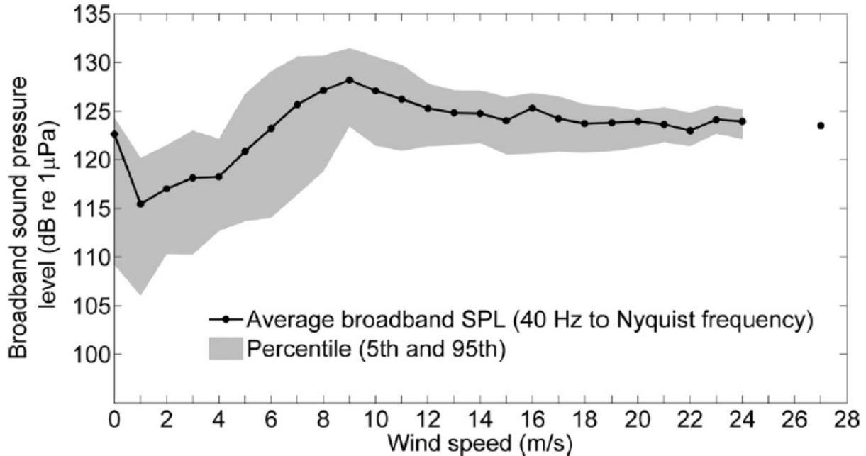
Figure 7.2: Measured broadband noise level from a Siemens SWT 3.6-107 turbine operating at different wind speeds. Bandwidth of the recordings was 40 Hz to 3.5 kHz (Nyquist frequency). From Pangerc et al. [2016].
