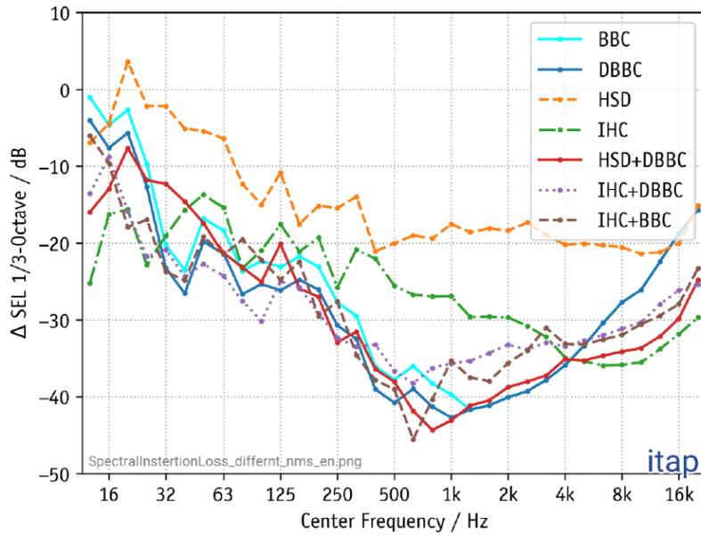
Figure 5.6: Frequency dependent noise reduction for different NAS, [Bellmann, et al., August 2020].
