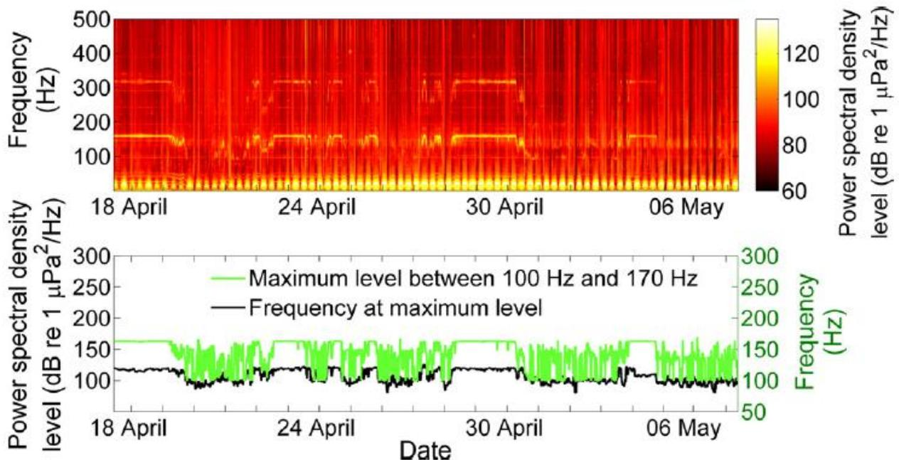
Figure 7.1: Measurement of underwater noise 50 m from a Siemens SWT 3.6-107 wind turbine over a 3-week period. From Pangerc et al. [2016]. The regularly fluctuating pattern at frequencies below 30 Hz is an artefact caused by fluctuating levels of flow noise due to the tide and is thus unrelated to the turbine.
