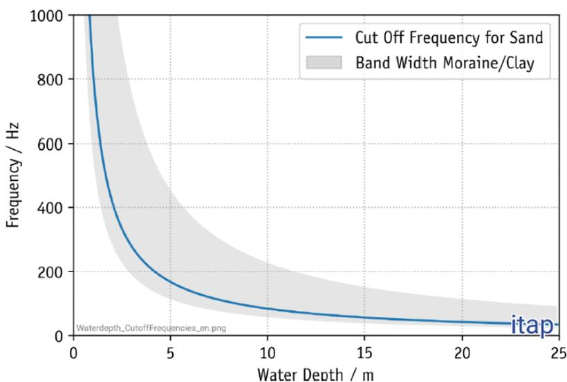
Figure 5.2: Cut off frequency and its dependency on sediment type and water depth [Bellmann, et al., August 2020].
