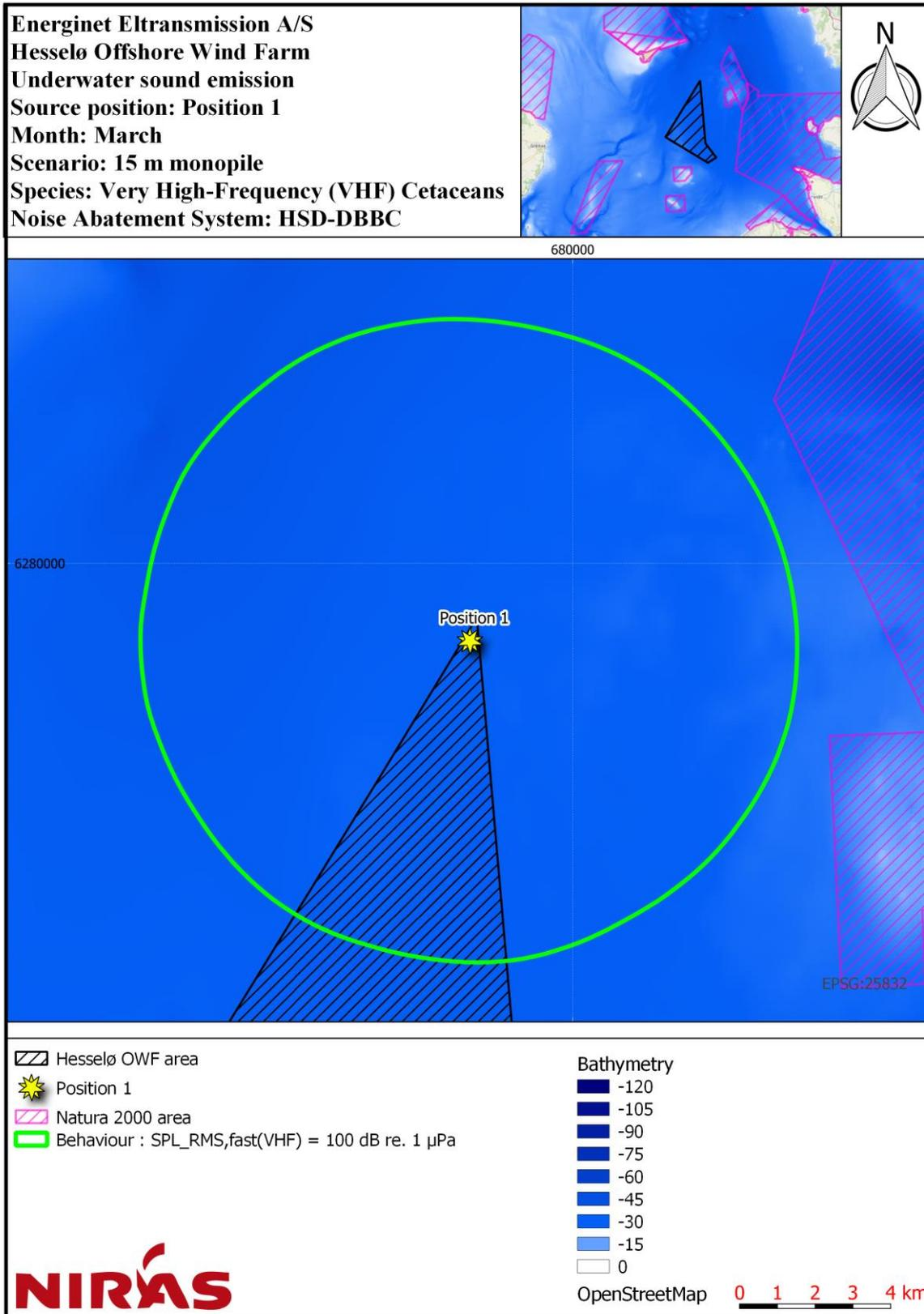
Figure 6.1: Noise contour map for position 1, showing impact distances for behaviour with VHF-weighting and HSD-DBBC NAS on a 15 m monopile.
