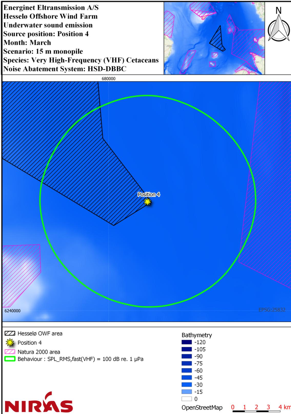
Figure 6.4: Noise contour map for position 4, showing impact distances for behaviour with VHF-weighting and HSD-DBBC NAS on a 15 m monopile.
