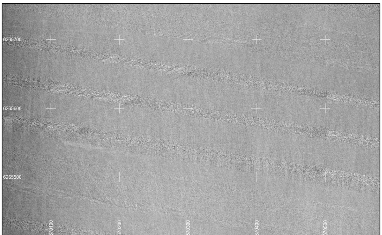
Figure 5.1: HOWF site backscatter, highlighting subtle nadir striping on flat seafloor.
