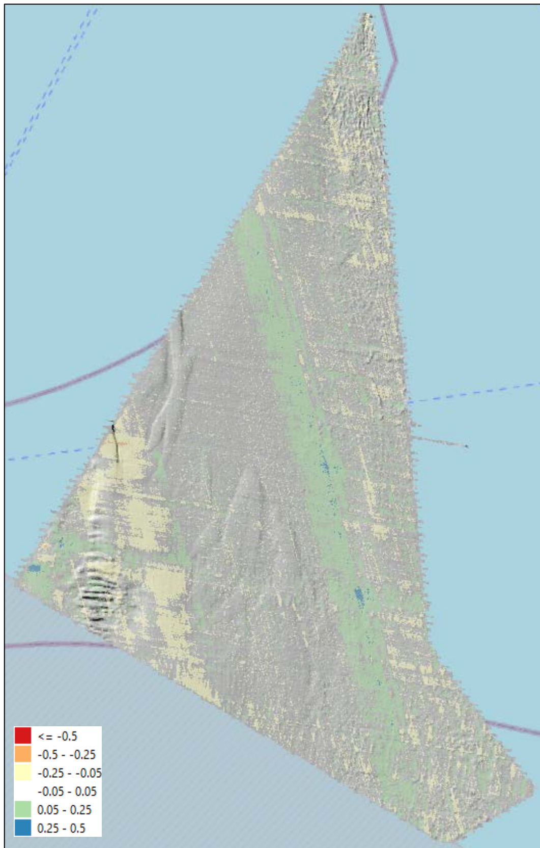
Figure 5.4: General overview of bathymetry differences between WPA and WPB. Positive values refer to areas where seabed elevation was interpreted as being higher for WPB than for WPA
