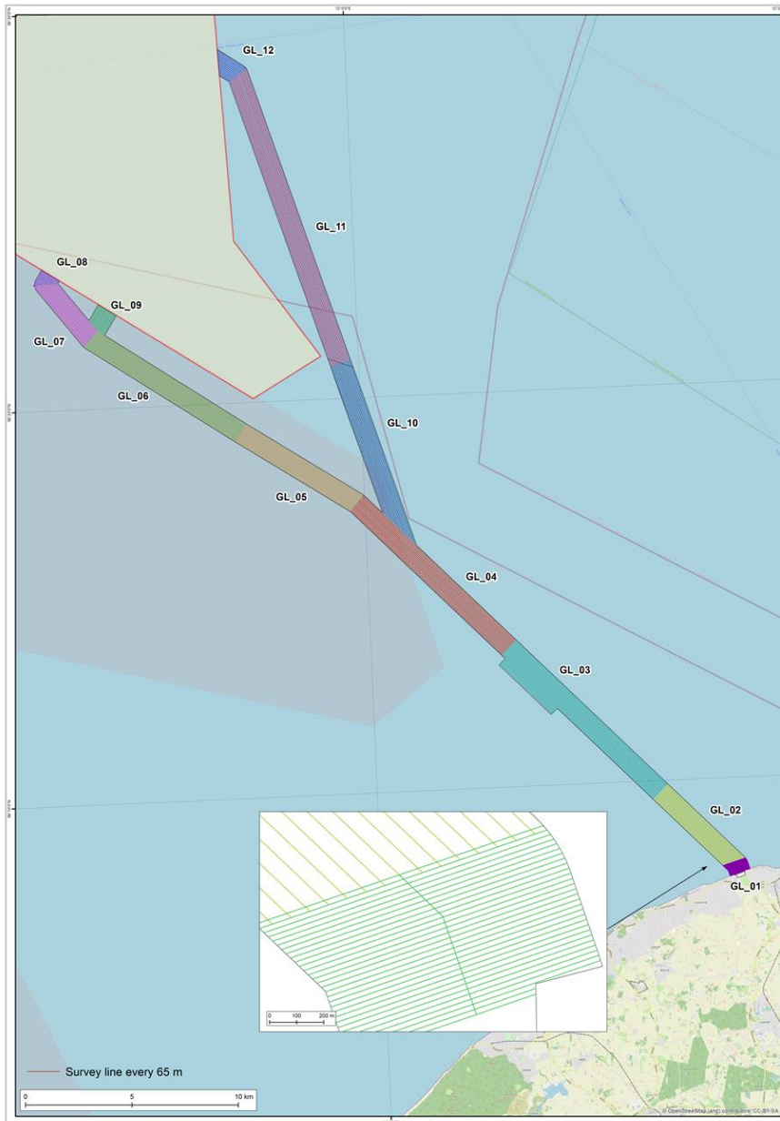
Figure 3-3 Survey area showing the sub-division into 12 sections with inserts showing planned line direction..
