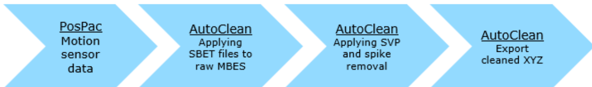
Figure 5-2 Workflow for the MBES processing in AutoClean.
