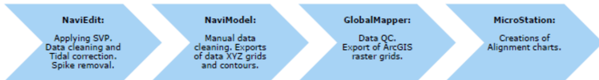
Figure 5-1 Workflow for the MBES processing in NaviEdit.
