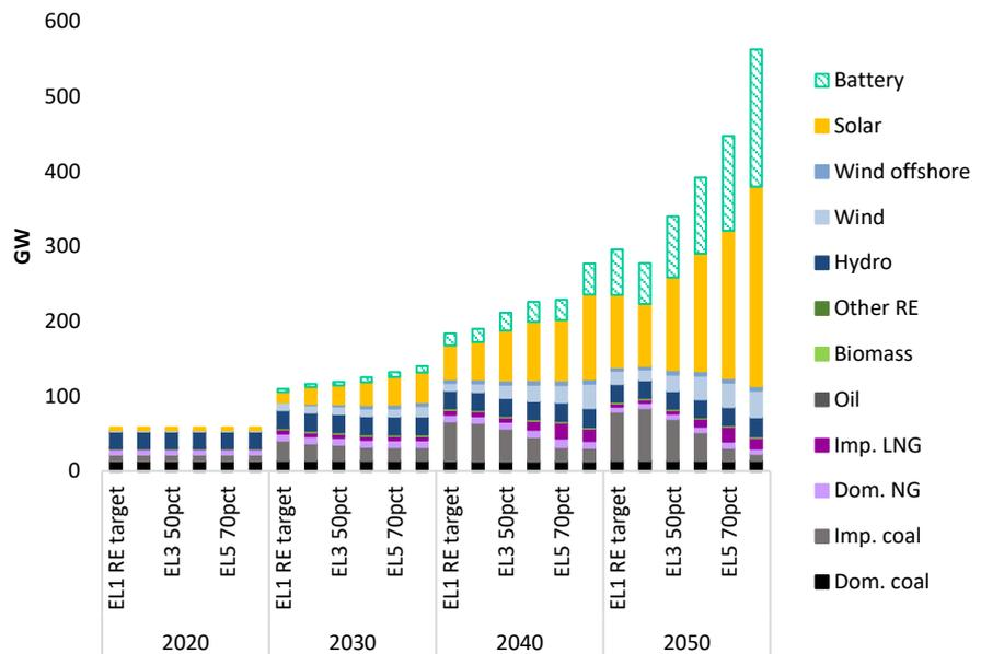
Figure 57: Generation capacity for the six CO<sub>2</sub> emission limit (EL) scenarios.
