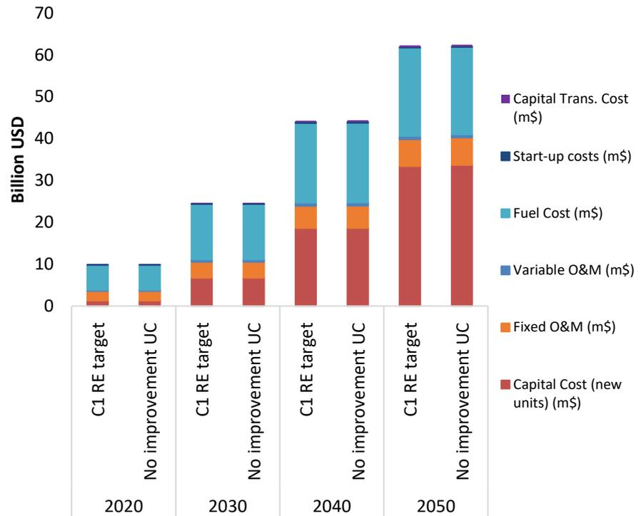
Figure 73: Comparing total system cost of the No improvement UC and C1 RE target scenarios.
