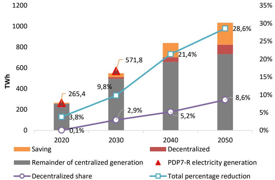
Figure 38: Effects of EE measures and industrial CHPs in C3-REEE scenario with respect to C1-RE scenario. “Decentralized” consists of approximately 80% industrial CHPs and 20% decentralised solar PVs.
