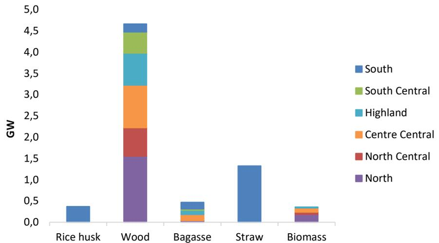
Figure 15: Resource limits on biomass-fired power generation capacity implemented in the Balmorel model.
