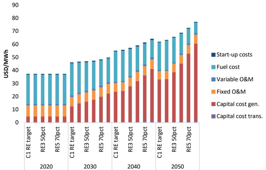
Figure 55: Total system cost per MWh in C1 RE target and the five RE share scenarios.
