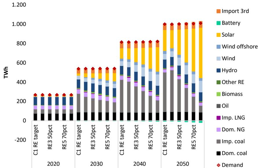
Figure 51: Annual electricity generation, import from 3<sup>rd</sup> countries and power demand (including transmission and distribution losses) in C1 RE target and the five RE share scenarios. Negative values for batteries represent the loss in the batteries.
