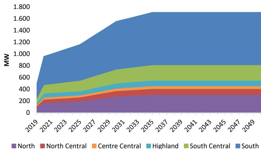
Figure 16: Resource limits on MSW-fired power plant generation capacity implemented in the Balmorel model.
