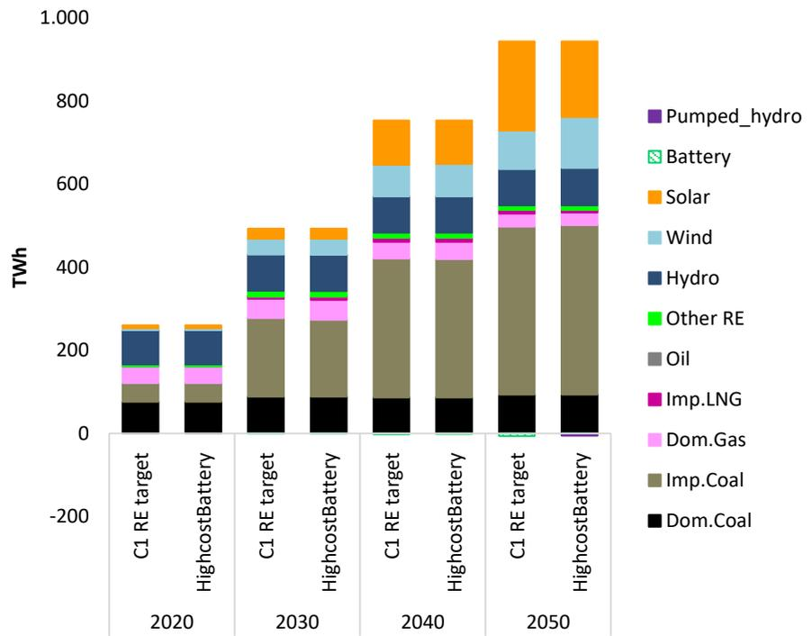
Figure 75: Comparing energy generation by power source type in the High cost battery and C1 RE target scenarios.
