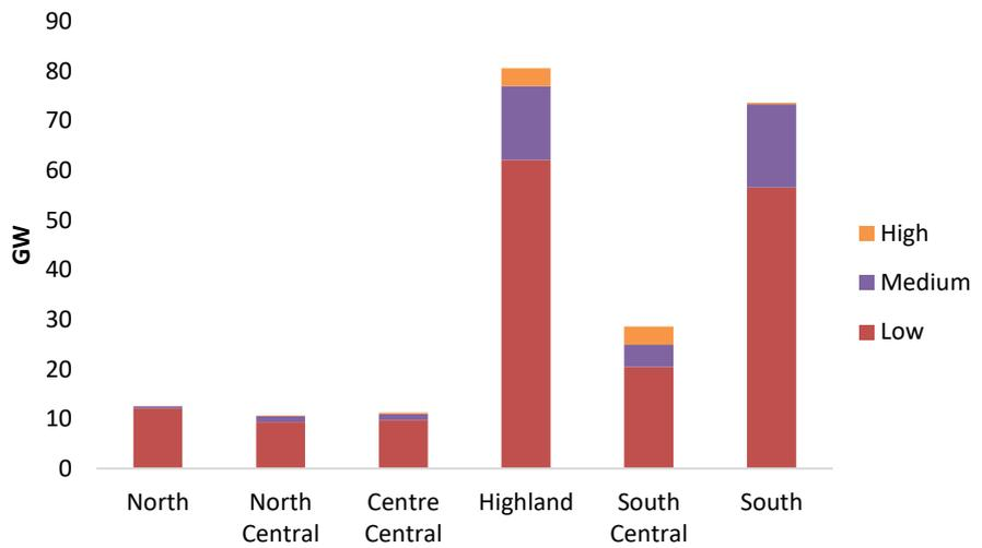
Figure 17: Resource limits on wind generation capacity per region and wind speed class implemented in the Balmorel model. Low: 4.5-5.5 m/s, Medium: 5.5-6 m/s, High: over 6 m/s (all at 80 m height).
