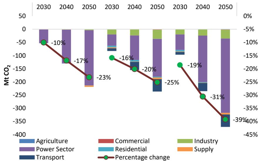
Figure 42: CO<sub>2</sub> emission reduction by sector in *C3 Energy efficiency* scenario (left) and *C4 Combination* scenario (right) with respect to *C1 RE target* scenario.
