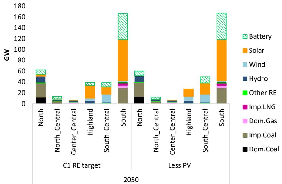
Figure 81: Comparing Installed capacity by power source types and regions in the *Less PV* and *C1 RE target* scenarios in 2050.
