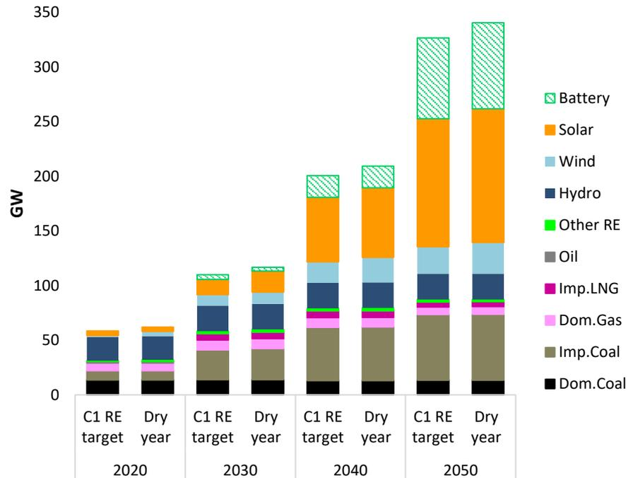
Figure 83: Comparing Installed capacity by power source type in the Dry year and C1 RE target scenarios.
