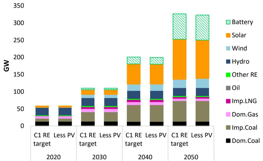
Figure 80: Comparing Installed capacity by power source type in the Less PV and C1 RE target scenarios.
