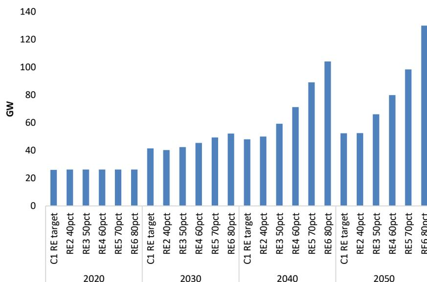
Figure 56: Transmission capacity in C1 RE target and the five RE share scenarios. The figure shows the sum of the capacity of the seven transmission lines.
