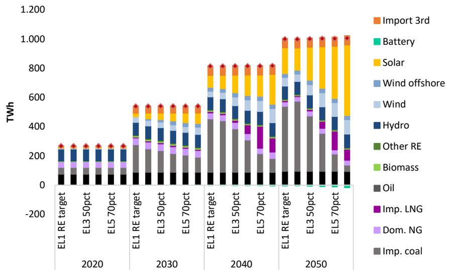
Figure 58: Annual electricity generation, import from 3<sup>rd</sup> countries and power demand (including transmission and distribution losses) in the six CO<sub>2</sub> emission limit scenarios. Note: The negative generation from batteries is the net loss.
