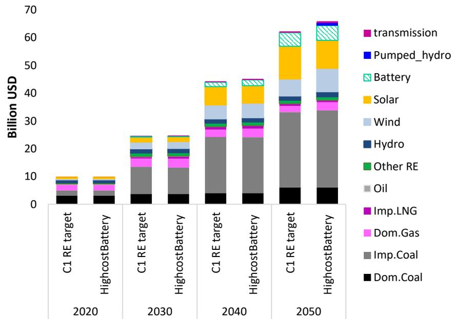
Figure 78: Comparing total system cost of High cost Battery and C1 RE target scenarios by types of source in 2050.
