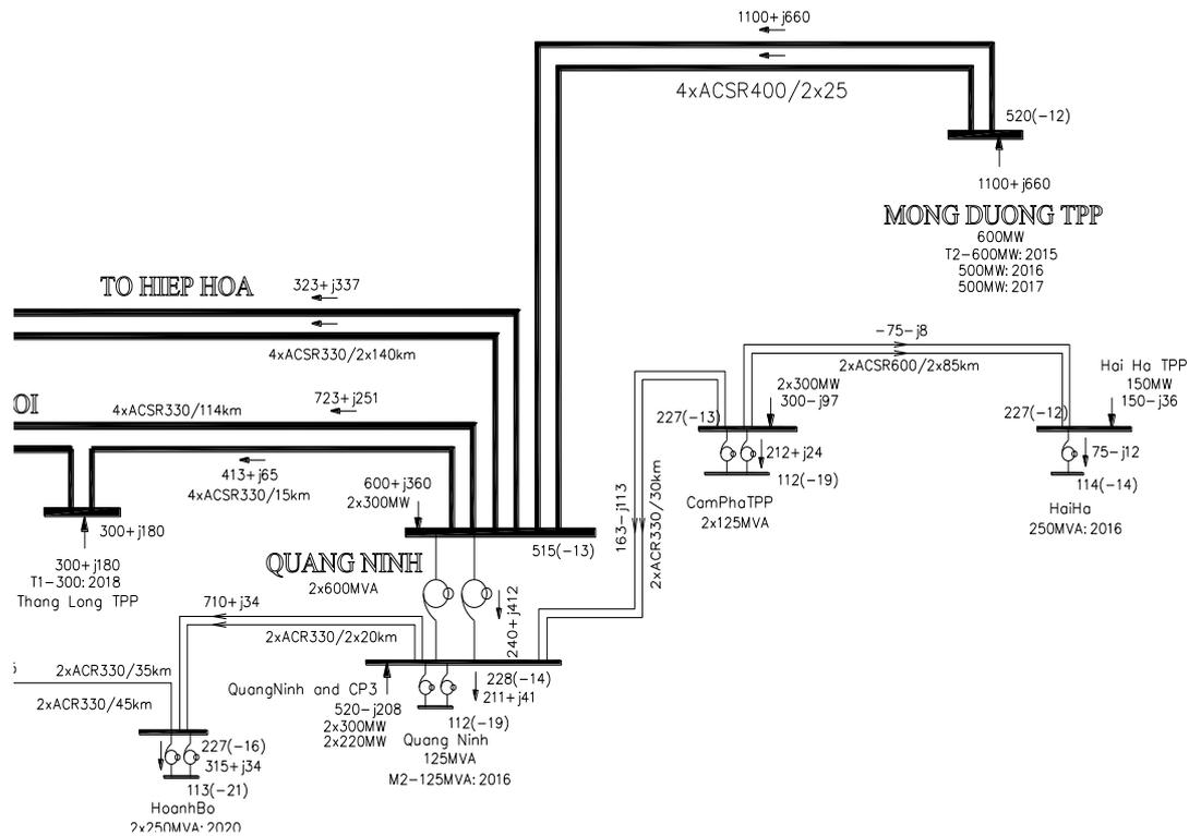
Figure 6: The 500kV and 220kV power grid of Quang Ninh province in year 2020.
