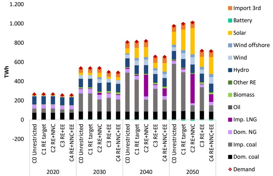
Figure 44: Annual electricity generation, import from 3<sup>rd</sup> countries and power demand (including transmission and distribution losses) in the five core scenarios. Negative values for batteries represent the loss in the batteries.
