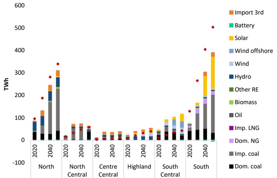
Figure 45: Annual electricity generation, import from 3<sup>rd</sup> countries and power demand (including transmission and distribution losses) per region for the C1 RE Target scenario. Negative values for batteries represent the loss in the batteries.
