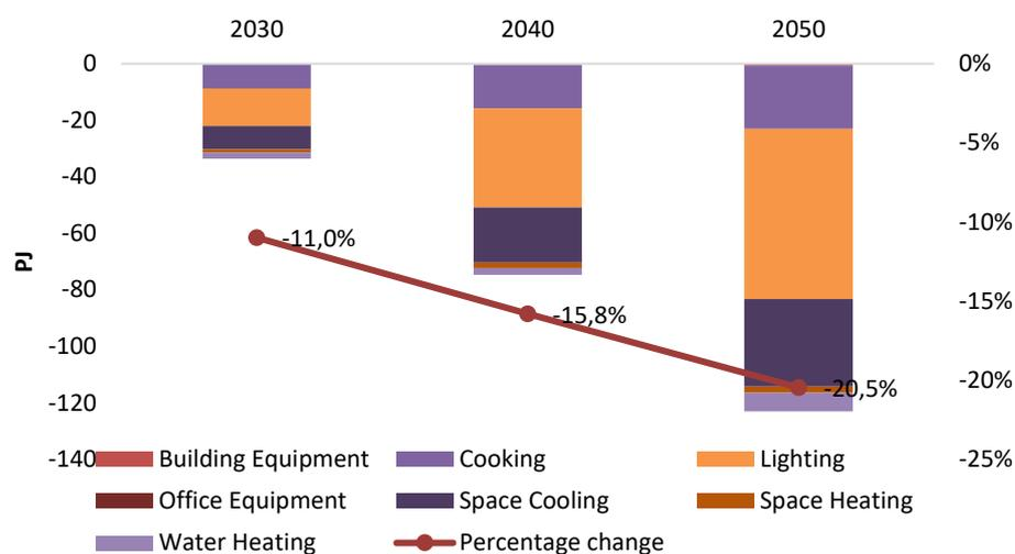
Figure 37: Energy saving potential by commercial end-use in C3 Energy efficiency scenario with respect to C1 RE target scenario.
