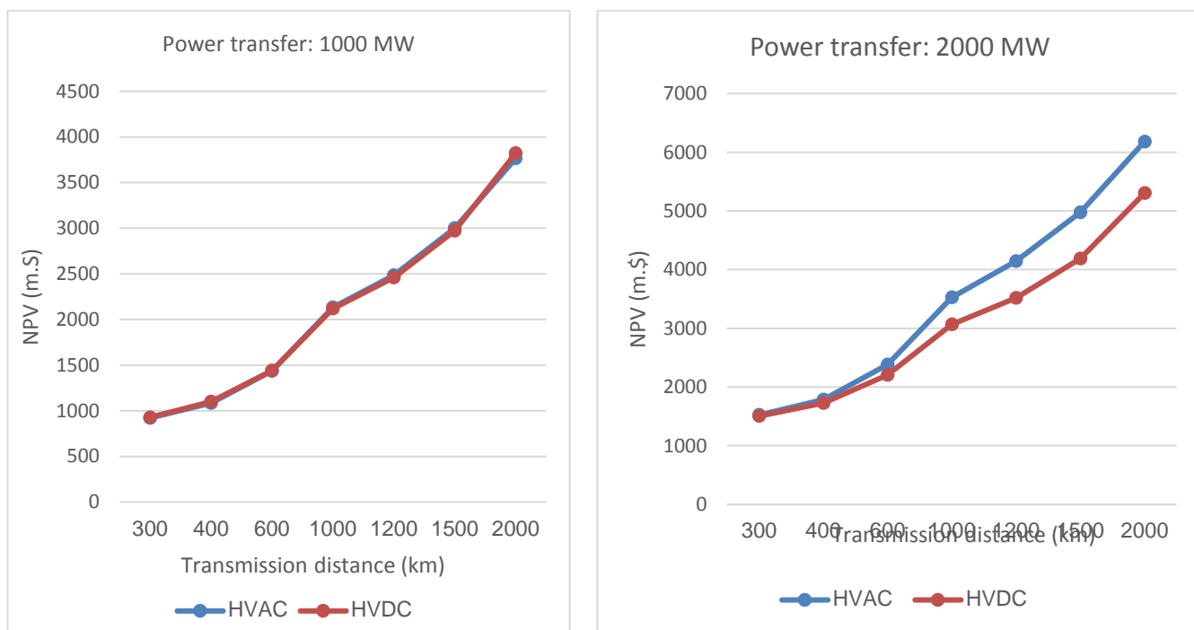
Figure 2-38 Net present value of HVAC and HVDC transmission alternatives in the power transfer scenario of 1000 and 2000 MW
