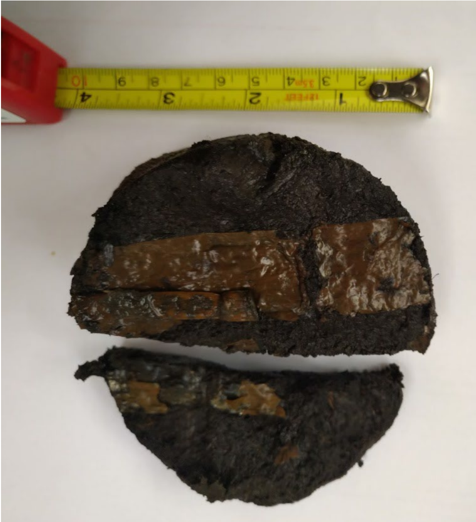
Figure 22. Photo of peat sample from core 282-VC-OWF-B1-007 (2.25-2.37 m under the seabed) showing well-preserved fragments of Phragmites reed.
