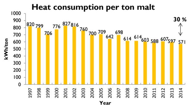
Figure 3. Development in heat consumption per ton malt.
