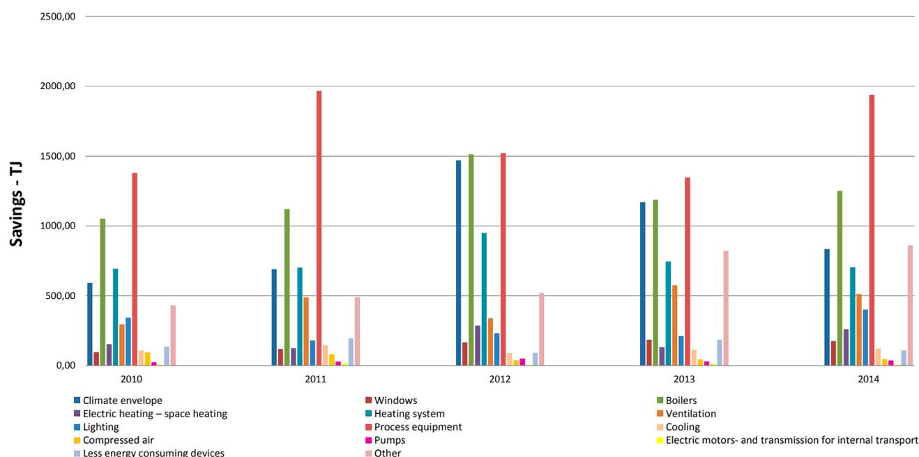
Figure 7. Development of savings found in different technologies
