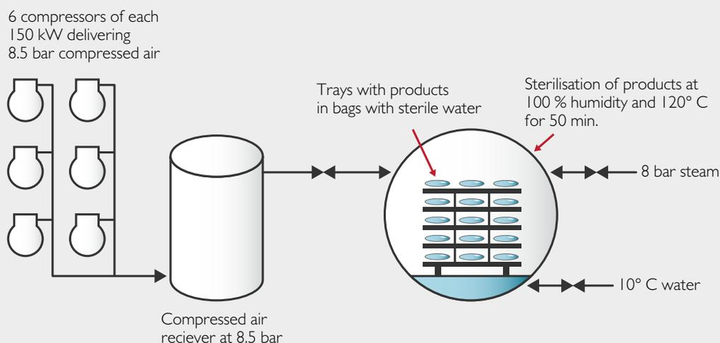
Figure 12. Autoclave for sterilisation of healthcare products
