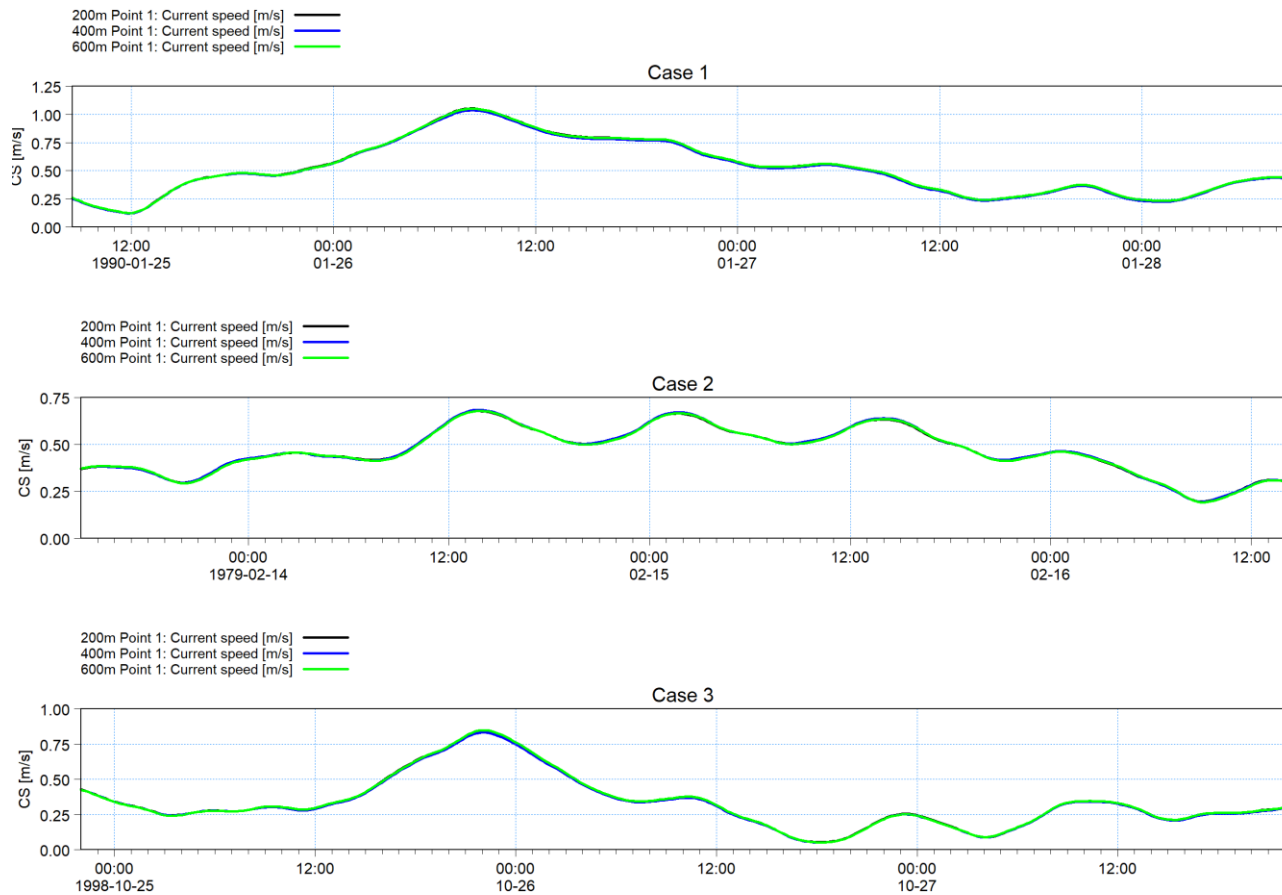
Figure 5.9 Comparison of current speeds for the different mesh resolutions at EINS-1 (Shallowest) Top: Case 01; Middle: Case 02, and Bottom: Case 03.
