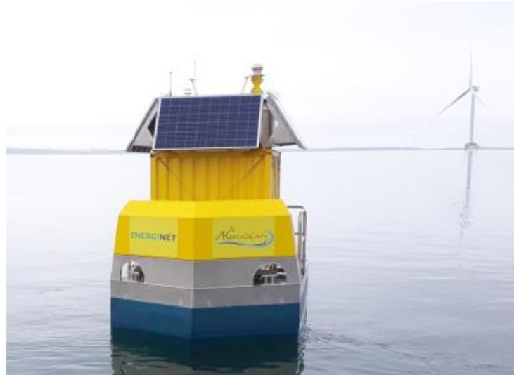
Figure 53. Picture from WINDSEA buoy and the LiDAR Thor, source: [39]
