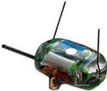
Figure 4. 2. The Wildlife Computers' SPLASH10-F-333 tag intended for cetaceans. Note the three different antennas.
