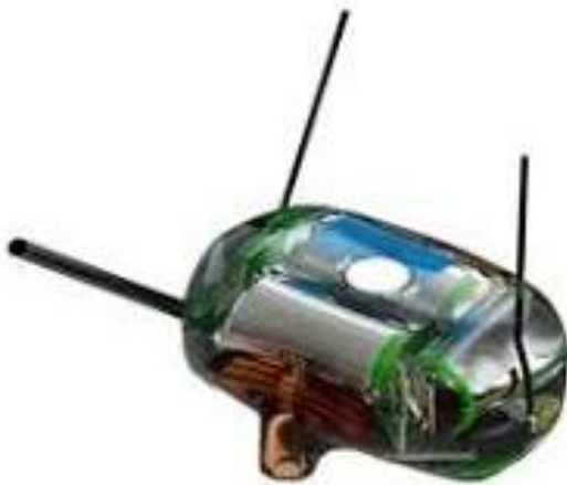
Figure 3. 7. The Wildlife Computers' SPLASH10-F-333 tag intended for cetaceans. Note the three different antennas.
