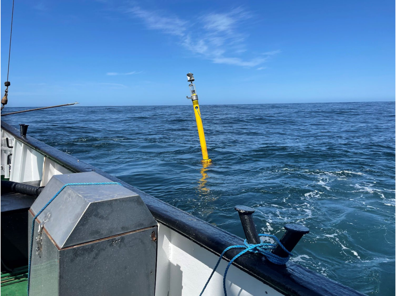
Figure 4.2. Bat Passive acoustic monitoring (PAM) station in the pre-investigation area. The recorder sits inside the metal 'casserole' beneath the light and reflector top piece, with the microphone mounted at the end of the protruding arm. The buoy shown had lost its yellow St. Andrews cross top mark, which was replaced during service.
