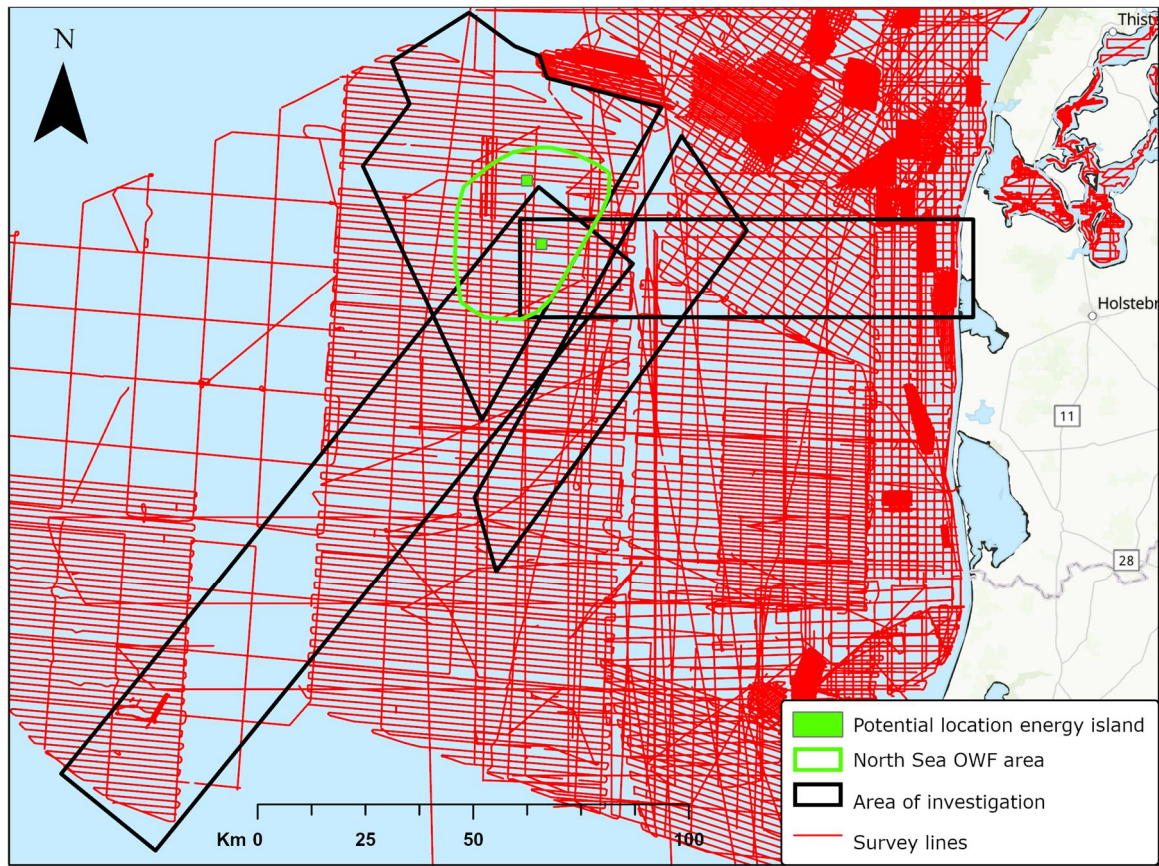
Figure 3-2: Overview of reported shallow seismic/geophysical survey lines in the area based on the Marta database.
