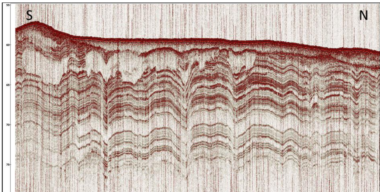
Figure 61 Raw Innomar data showing vertical striping Sparker interference.
