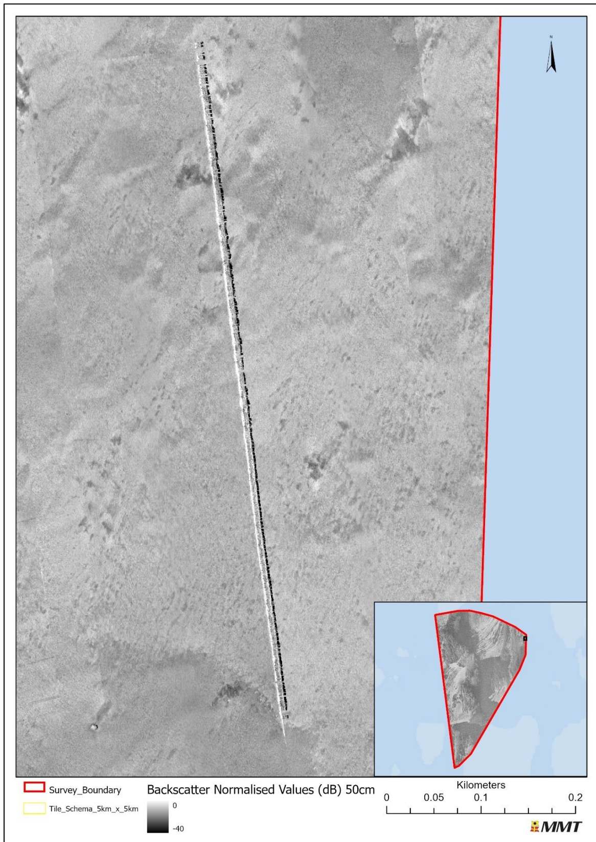
Figure 35 700m stretch of M/V Relume outer-beam noise visible in the backscatter dataset.
