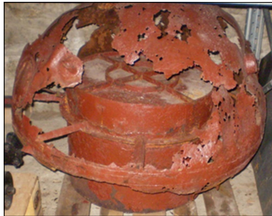
EMC Mine showing corrosion of buoyant casing, revealing main charge
