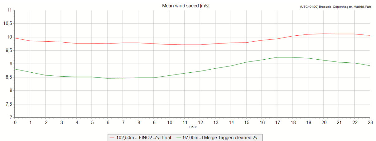
Figure 68. Daily variation of wind speed measured at FINO2 (7 years – 102.5 m) and Taggen (2 years – 97 m)
