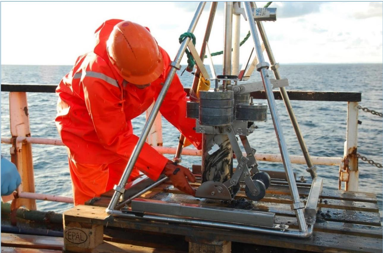
Figure 3-9. HAPS core sampler.
