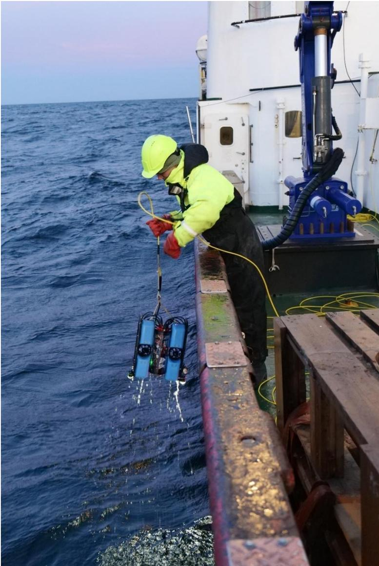
Figure 3-8. ROV being pulled out of the water.
