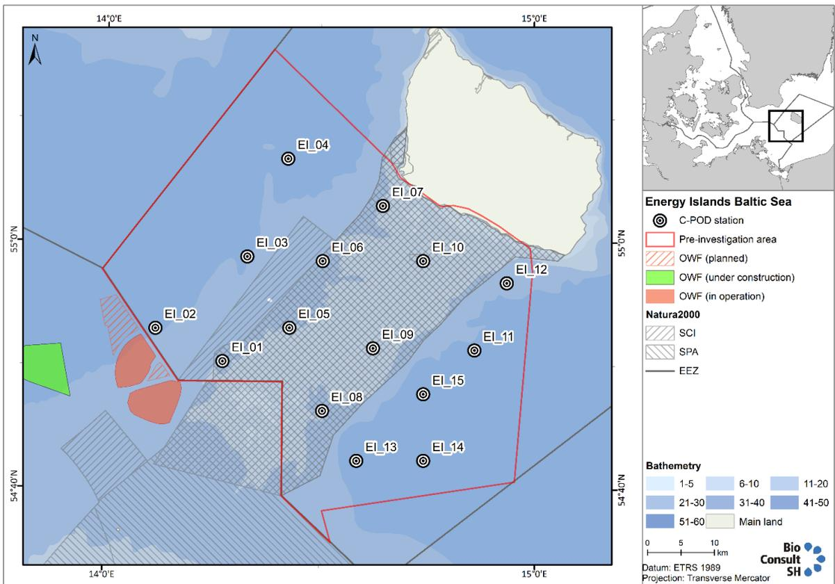
**Figure 3-3. Location of C-POD stations used for the passive acoustic monitoring survey in relation to the pre-investigation area of EIB.**
