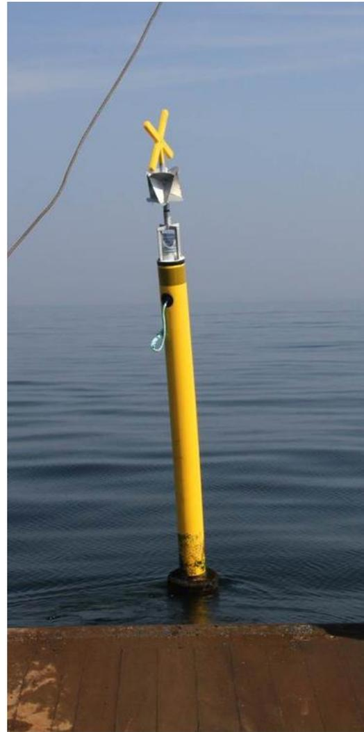
**Figure 3-5. C-POD mooring system with spar buoys.**
