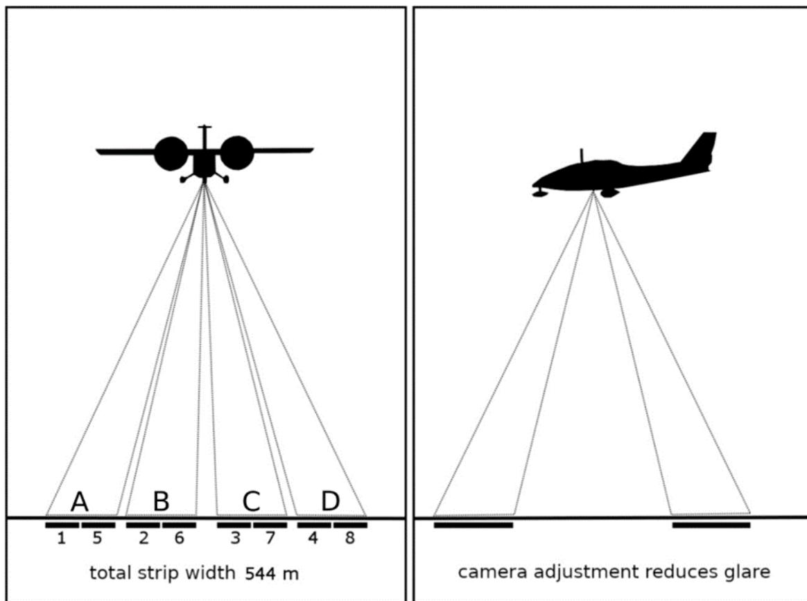
**Figure 3-2. The HiDef Camera-System. The four cameras (A to D) cover an effective strip width of 544 m of the sea surface at a flight altitude of 549 m (left: frontal view; right: side view). The numbering indicates the camera images as they are used in the evaluation (the images from each camera are divided into two halves).**
