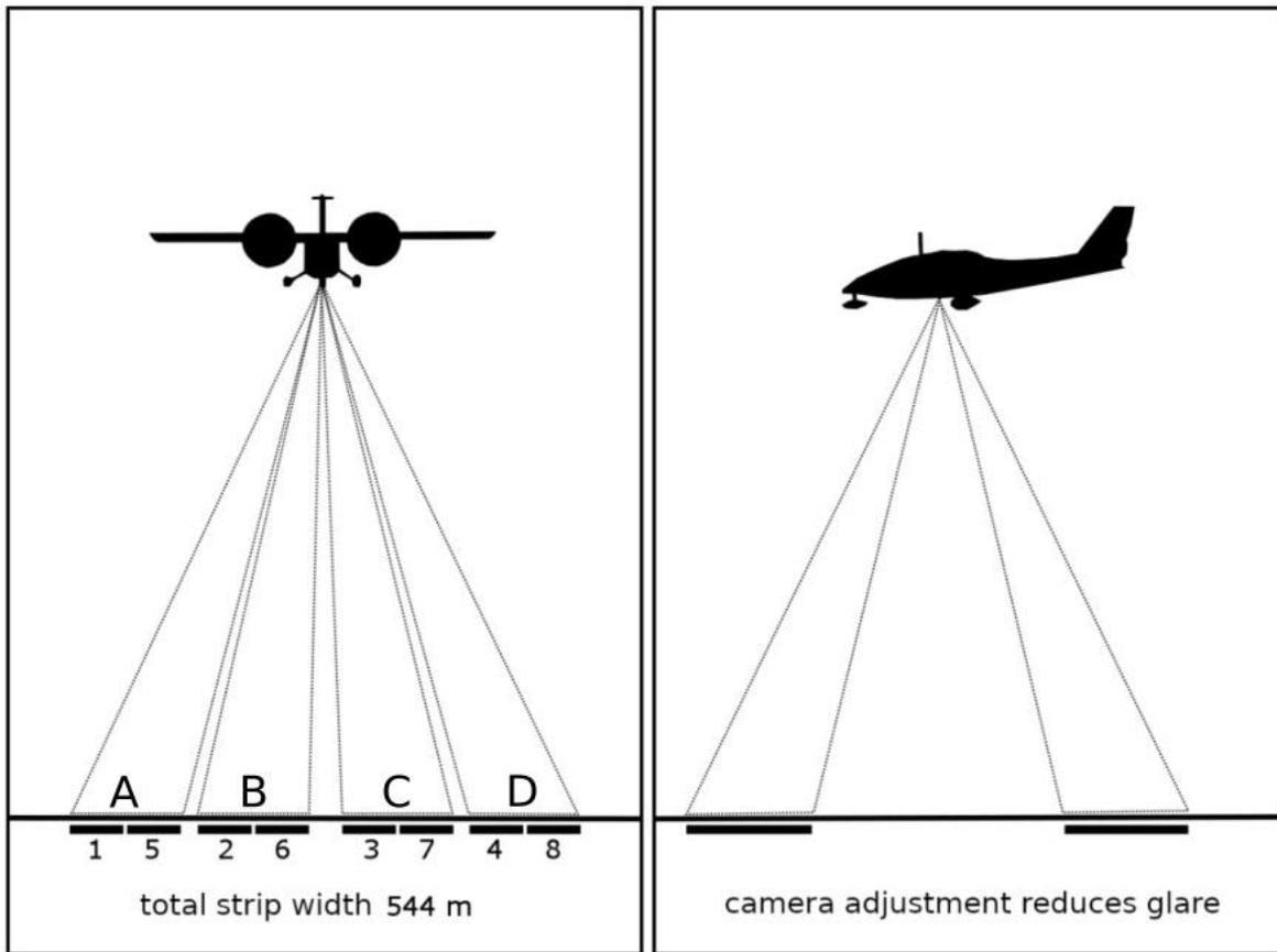
**Figure 4. The HiDef Camera-System. The four cameras (A to D) cover an effective strip width of 544 m of the sea surface at a flight altitude of 549 m (left: frontal view; right: side view). The numbering indicates the camera images as they are used in the evaluation (the images from each camera are divided into two halves).**
