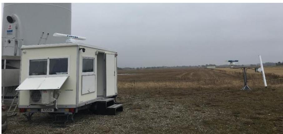
**Figure 2 Example setup of a bird radar station: Two radar units per station were used for this study. A horizontal radar is mounted on the roof of a caravan and is used to determine the flight direction of seasonally migrating bird species. A mobile vertical radar standing next to the trailer also collects data to determine flight altitude and migration intensity.**
