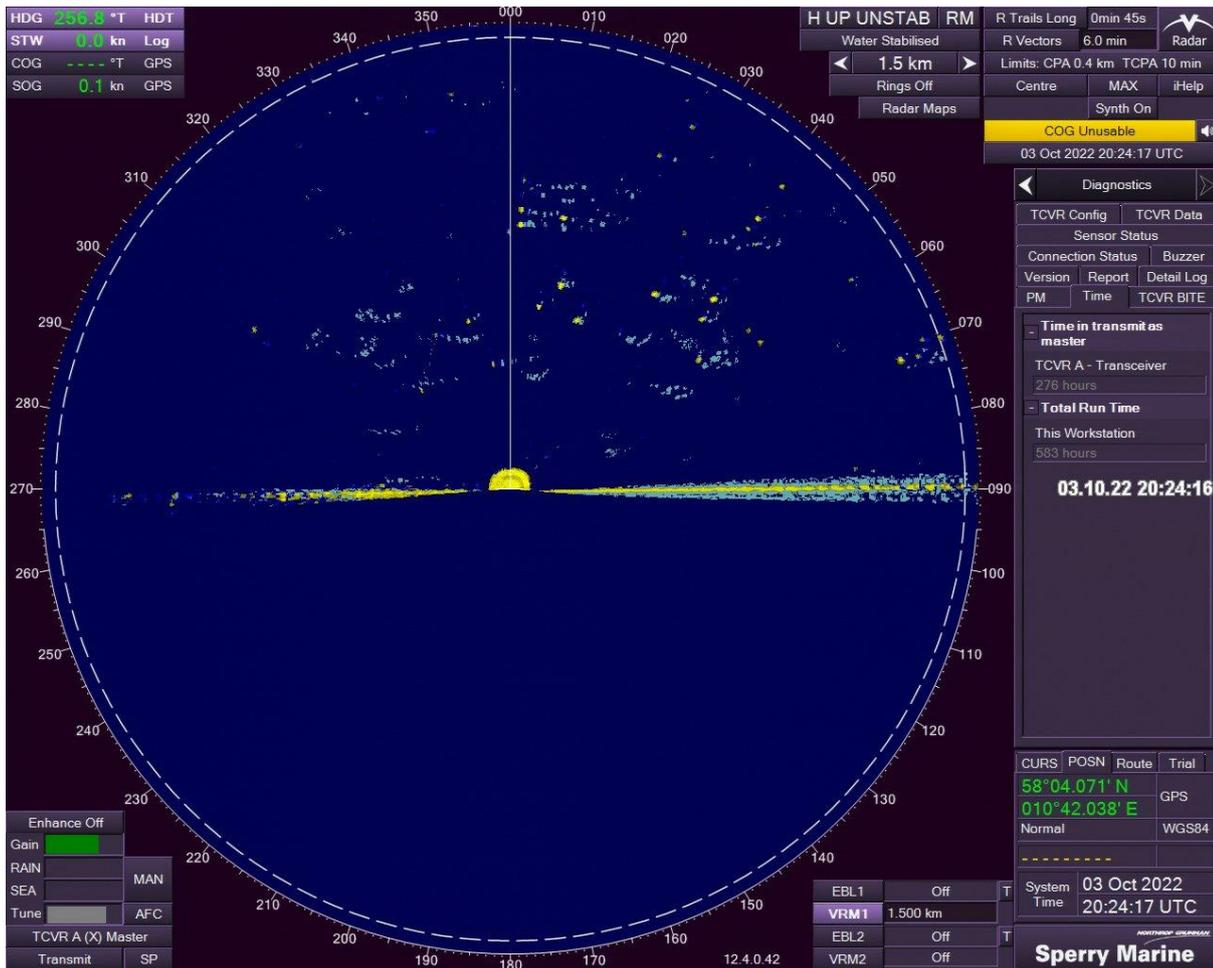
**Figure 5. Example of a screenshot from vertical radar. Bird signals can be recognized by the blue tracks in the wake of the current yellow signal.**
