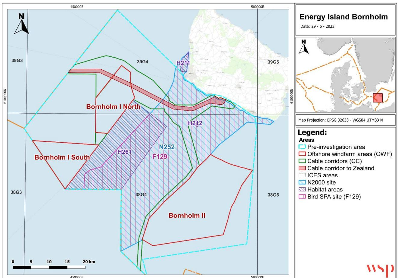
Figure 4-1 The pre-investigation area of ENOE OWF with offshore cable corridors and relevant habitat and N2000 sites.
