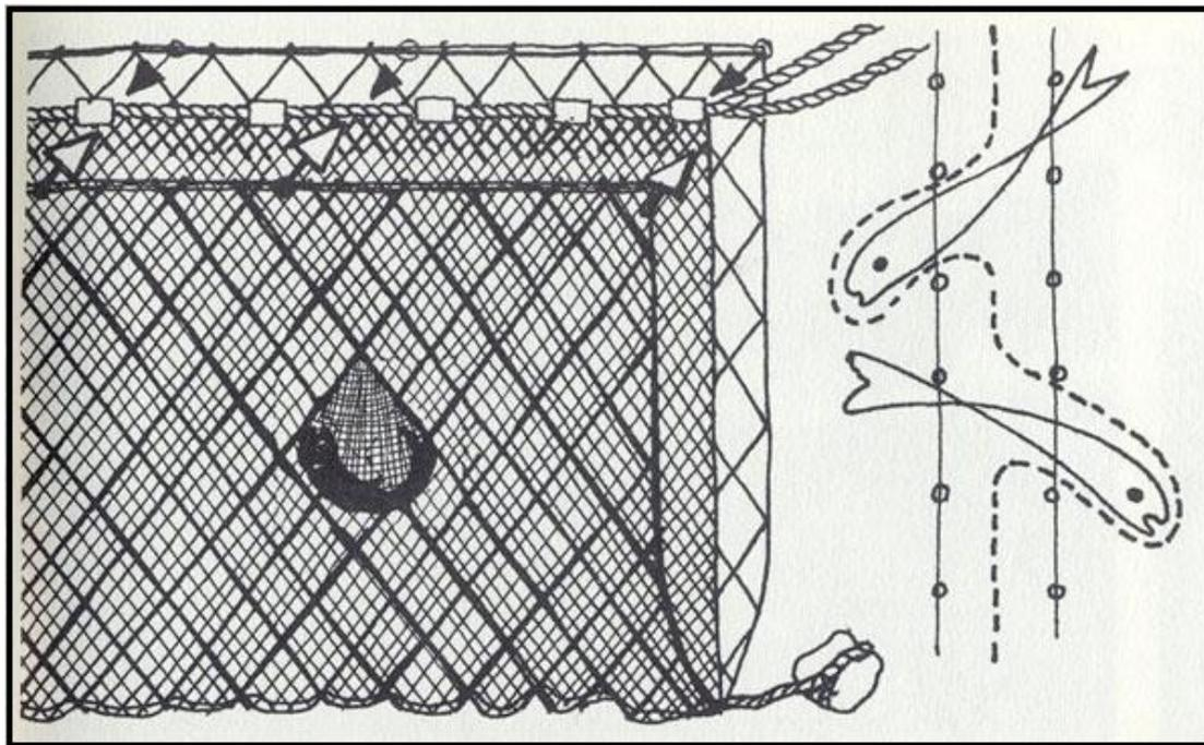
Figure 3-3 Trammel net with three layers of netting. The net layers catch the fish inside a “bag” instead of catching it by the gills (Garmer, 2023).
