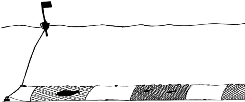
Figure 3-4 Multimesh gillnets with various mesh sizes specialized for catching a wide range of fish sizes.
