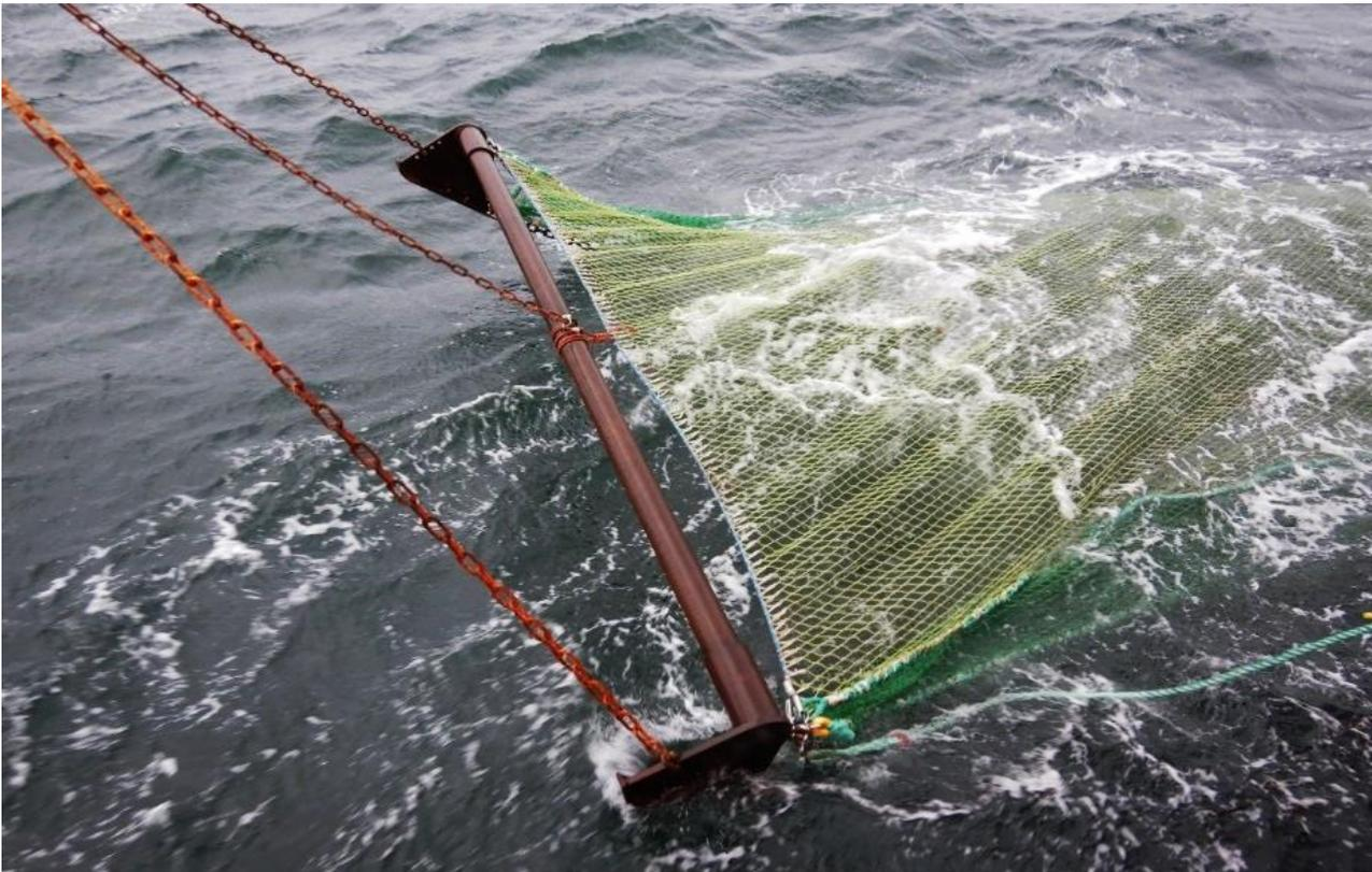
Figure 3-2 Beam trawl utilized for the fish survey of the pre-investigation area of ENOE OWF.
