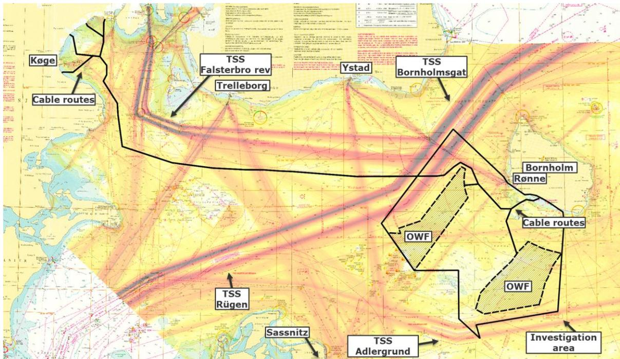
**Figure 2-4 Ship traffic density plot for all types of ships, based on AIS data from a one-year period (January 2019 to December 2019).**
