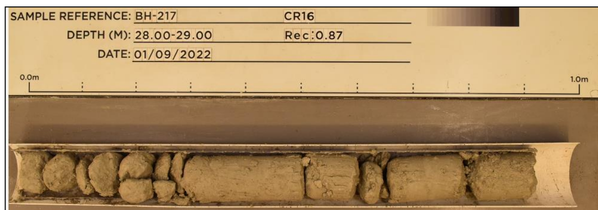
Figure 8-45. Example of drilling induced fractures causing the RQD value to be low.
