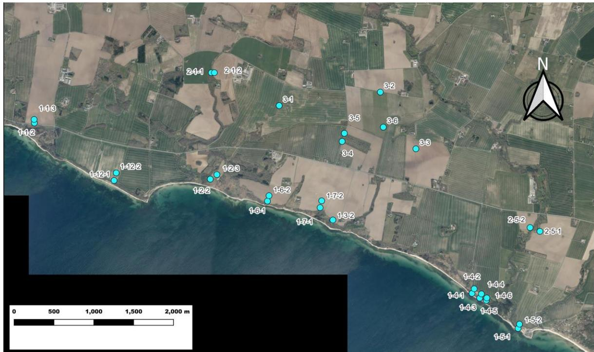
Figure 6.1 Location of boreholes with Recent, Fill and Lateglacial deposits; the boreholes are marked with blue dots
