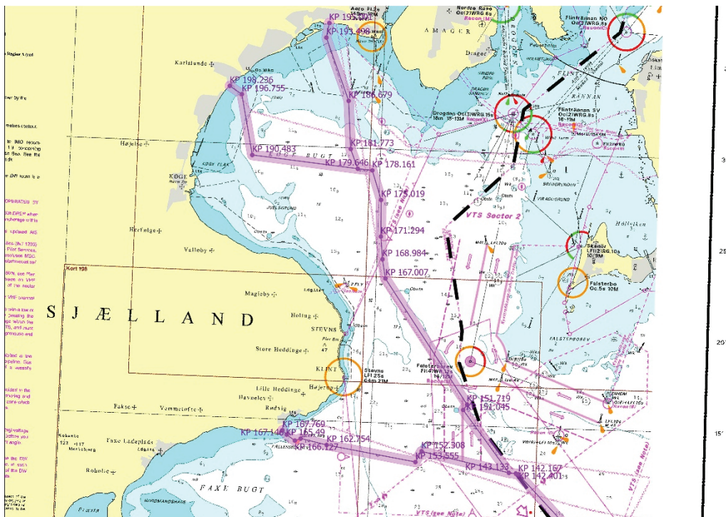
Figure 7-2. Overview of the cable route and survey corridor for part 3 from Danish EEZ to Landfall: PURPLE LINE: Cable Route. POINTS: Route Positions with KP values. PURPLE POLYGON: Survey corridor. EEZ boundary: Dashed BLACK LINE
