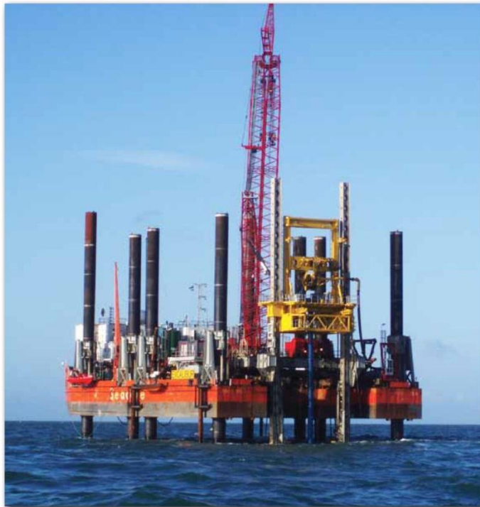
Seacore FUGRO SEACORE Excalibur jackup barge
