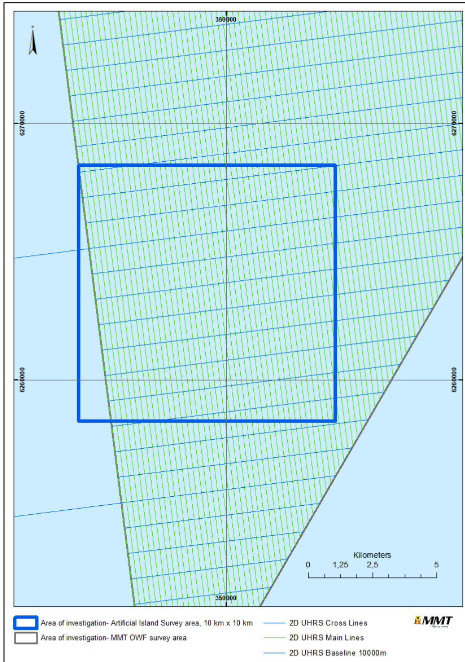
Figure 3 Line plan – 2D UHRS main and cross lines (Including geophysical data) within the Artificial Island survey area.
