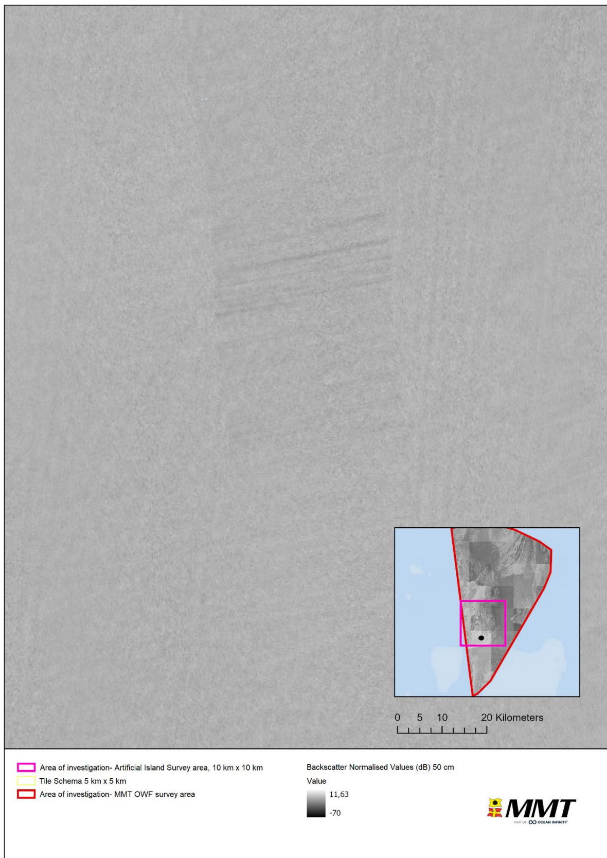
Figure 32 Outer beam busts visible in the Relume data, within the Artificial Island survey area.
