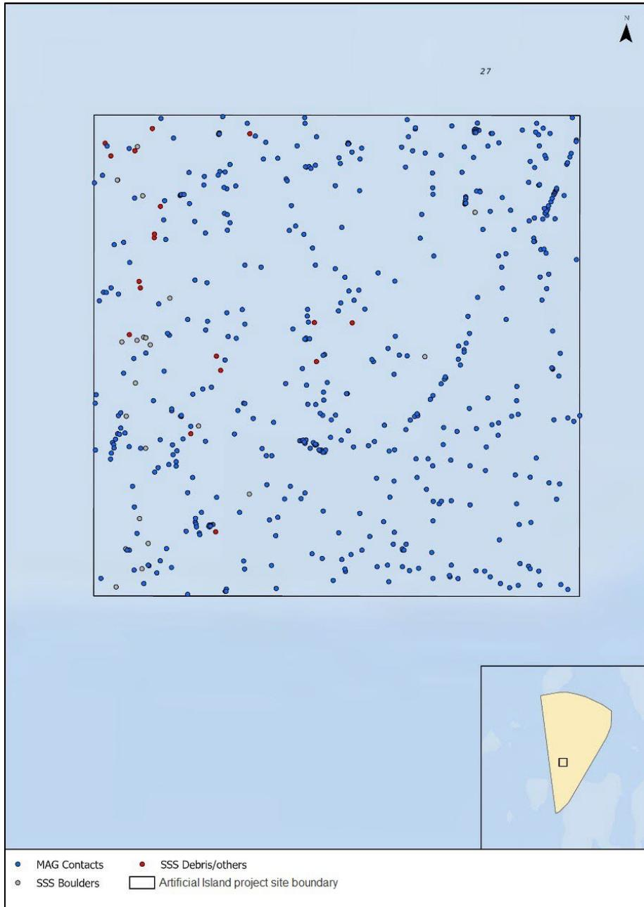
Figure 30 Distribution of contacts and anomalies within the Artificial Island project site.
