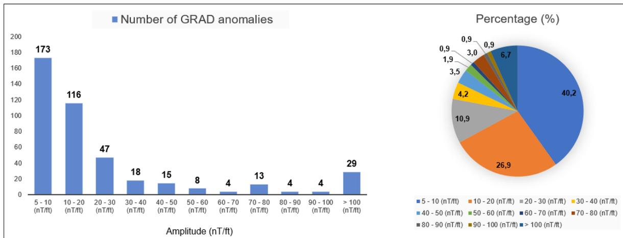
Figure 31 Histogram and pie chart illustrating the number and percentage of magnetic anomalies classified according to amplitude (nT/ft).
