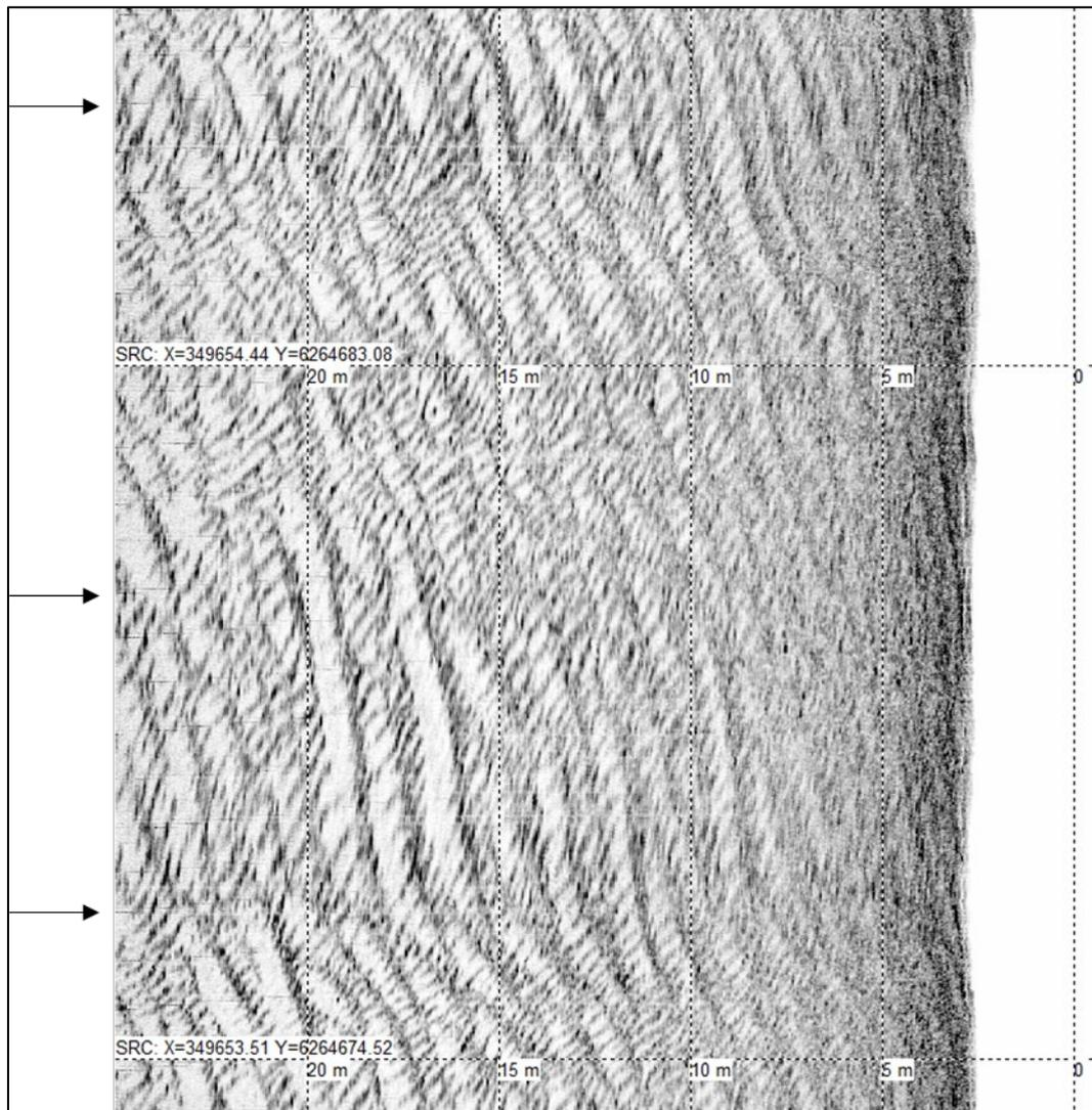
Figure 22 Example of mild electrical noise (horizontal dashed lines across the record) in SSS data on the outer range of the port channel. The image shows line 1660, in waterfall view. Horizontal scale lines at 5 m intervals, in waterfall view.
