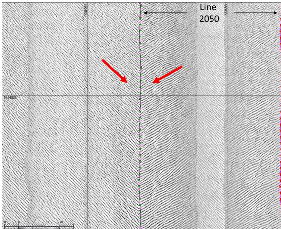
Figure 29 Change in ripple orientation observed in adjacent lines acquired on different days. The left side of the image acquired after waiting on weather and line 2050 acquired 2 weeks later.
