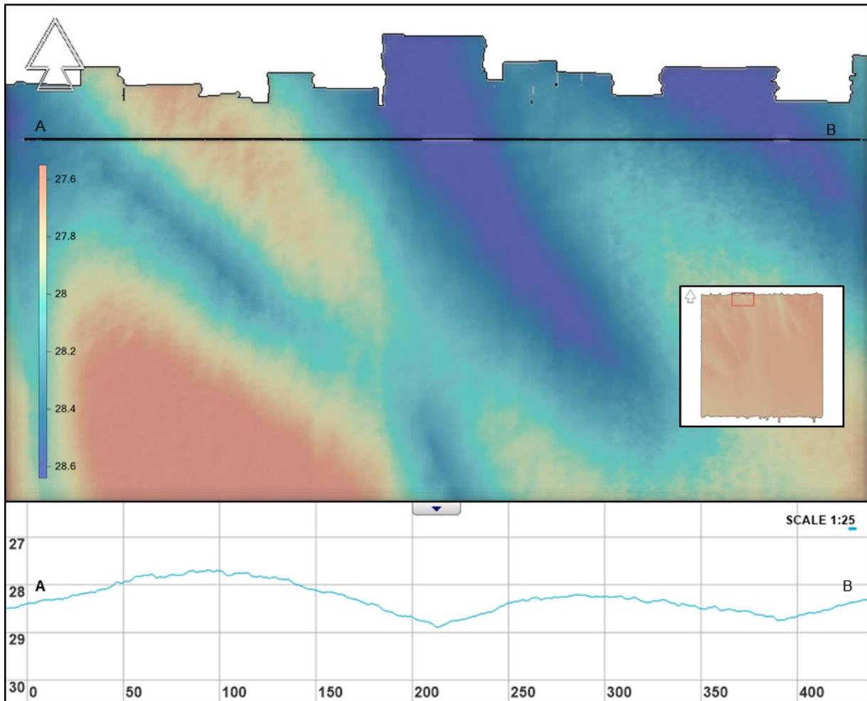
Figure 25 MBES image showing the maximum depth of the Artificial Island project site and surrounding seabed. NaviModel depth convention is positive down, vertical exaggeration of profile is 25. Red box in inset map highlights figure location.
