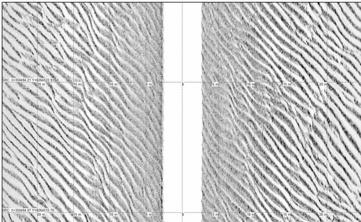
*Figure 18 Example of good high frequency SSS data, showing ripples. The data is from line 2500 in waterfall view. Horizontal scale lines at 5 m intervals.*
