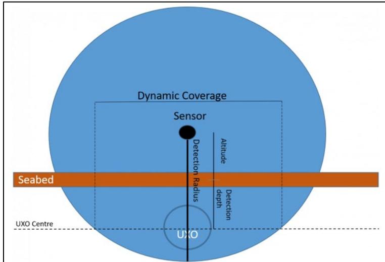
Figure 11 Dynamic Coverage parameters.
