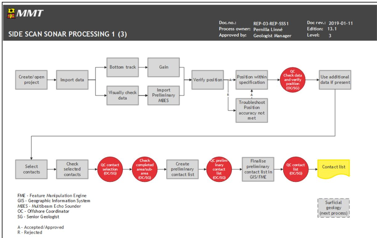
Figure 8 Workflow side scan sonar processing (1 of 2).
