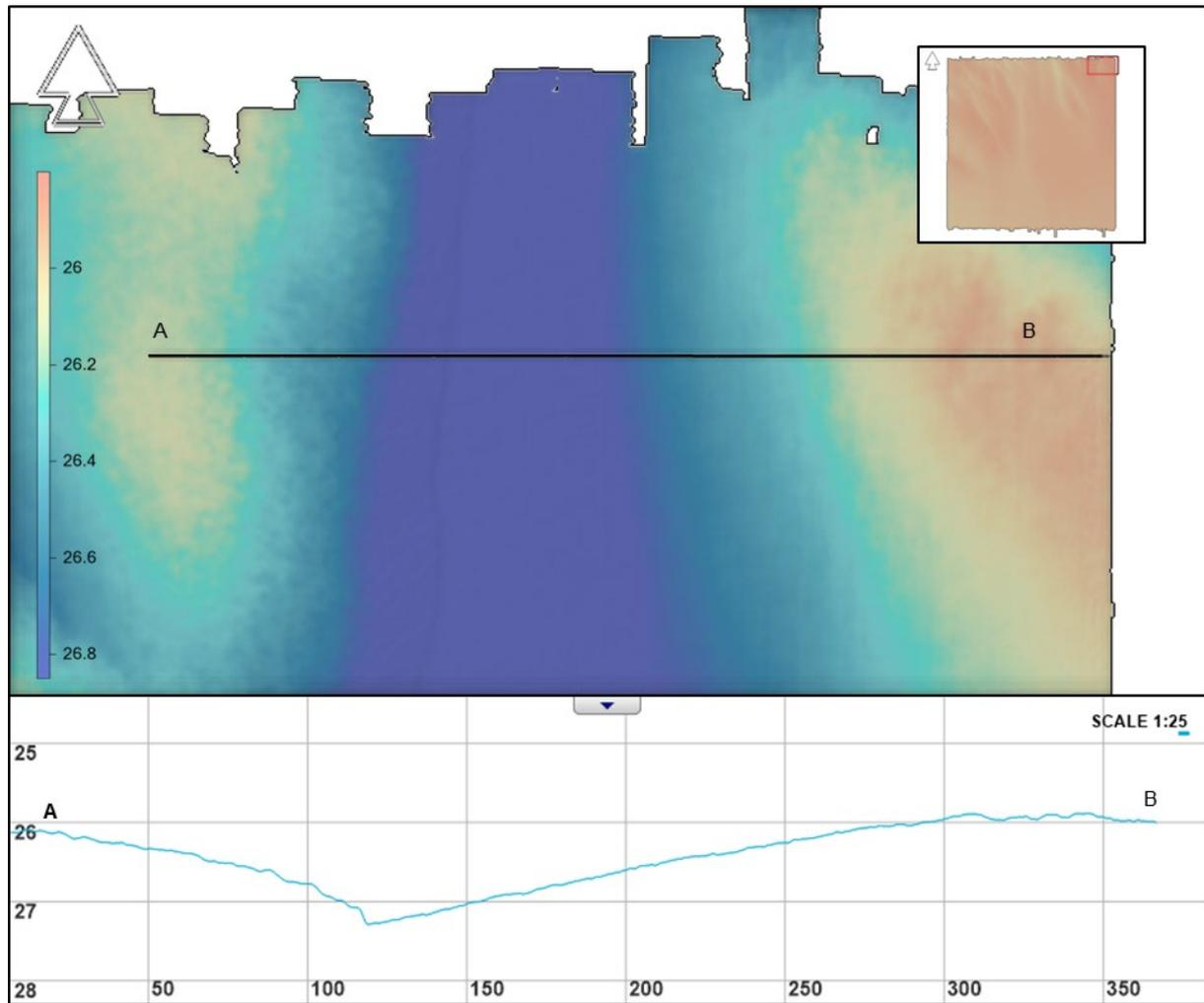
Figure 26 MBES Image showing 300m wide, 1.5m deep channel and shallowest depth of the Artificial Island project site. NaviModel depth convention is positive down, vertical exaggeration of profile is 25. Red box in inset map highlights figure location.
