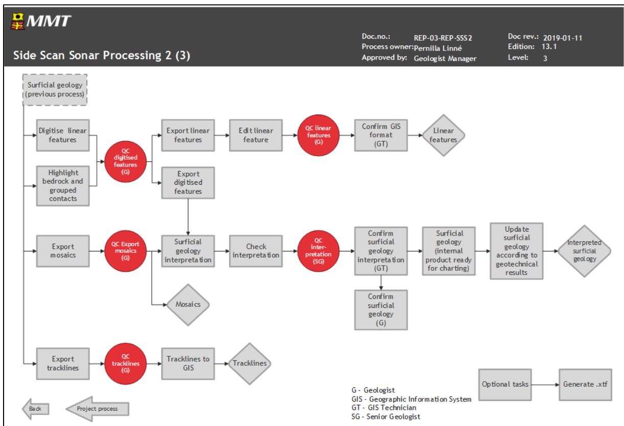
Figure 9 Workflow side scan sonar processing (2 of 2).
