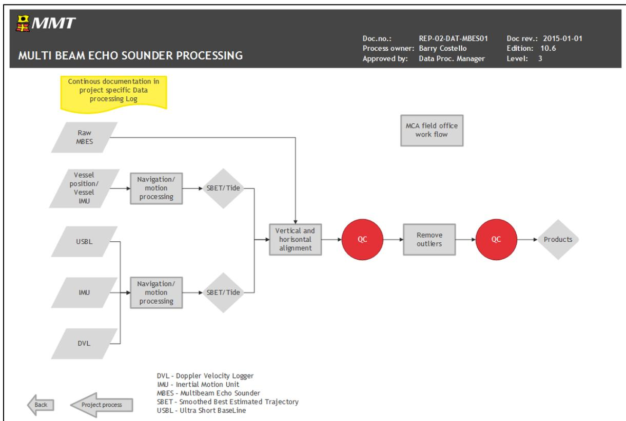
Figure 5 Workflow MBES processing.
