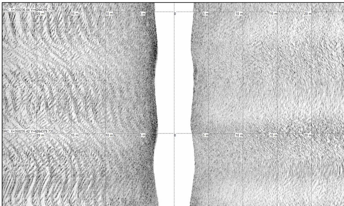
Figure 20 Moderate pitch and roll effects in an area of ripples.
