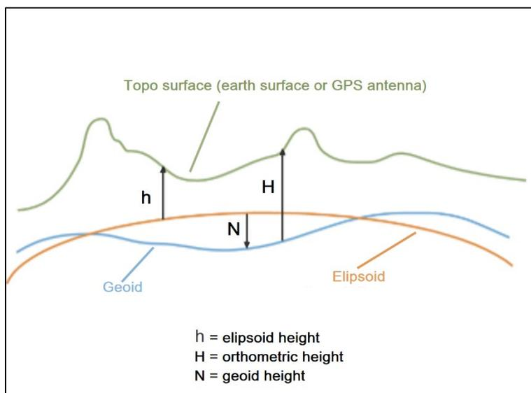
Figure 3 Overview of the relation between different vertical references.
