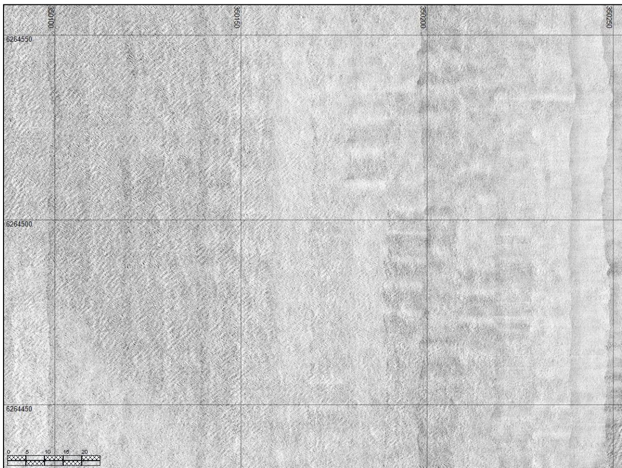
Figure 21 Example of striping in SSS data from moderate pitch and roll effects, in mosaic plan view.
