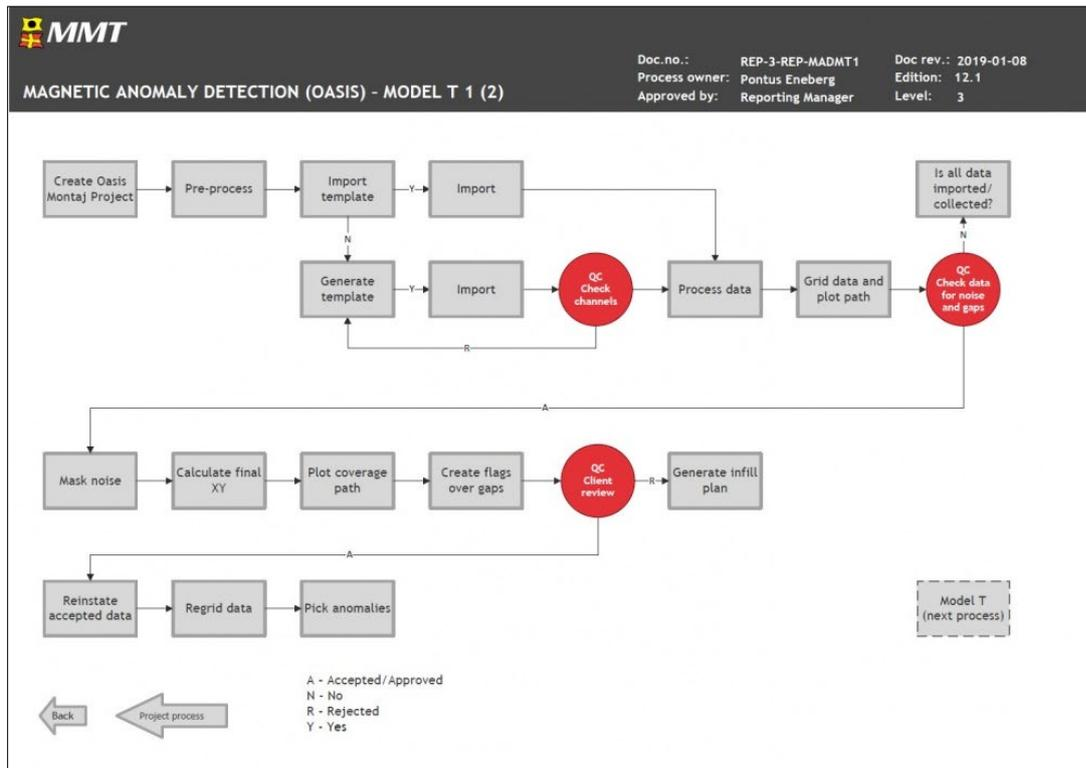
Figure 12 Workflow GRAD processing (1 of 2).
