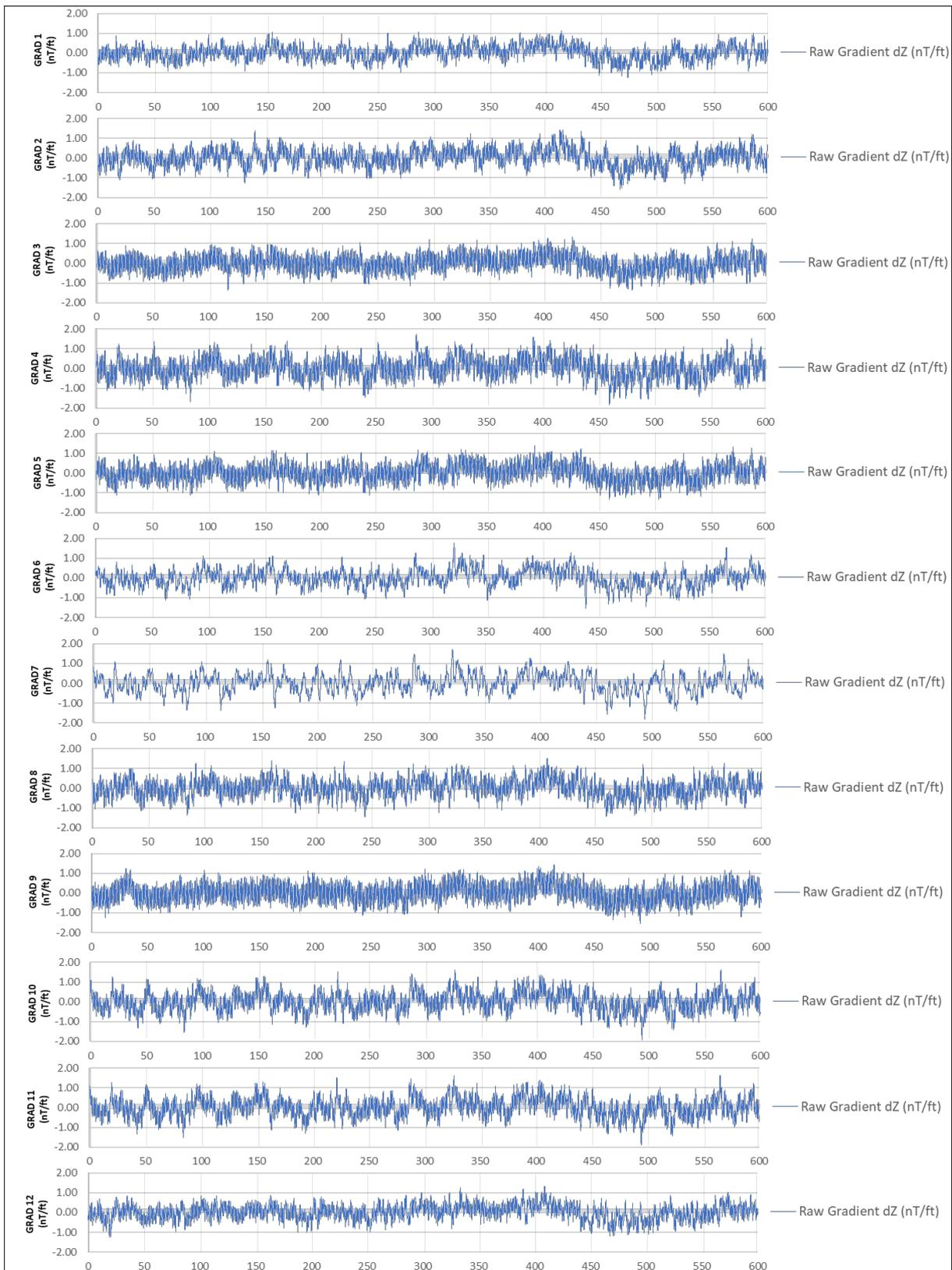
Figure 23 Gradiometer profile of line showing background noise levels below 2.5nT/ft PtoP. All twelve gradiometer pins shown.
