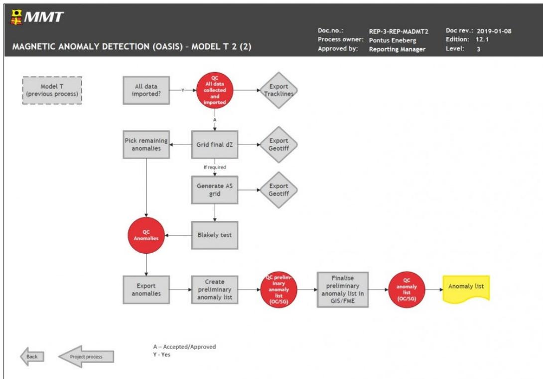
Figure 13 Workflow GRAD processing (2 of 2).
