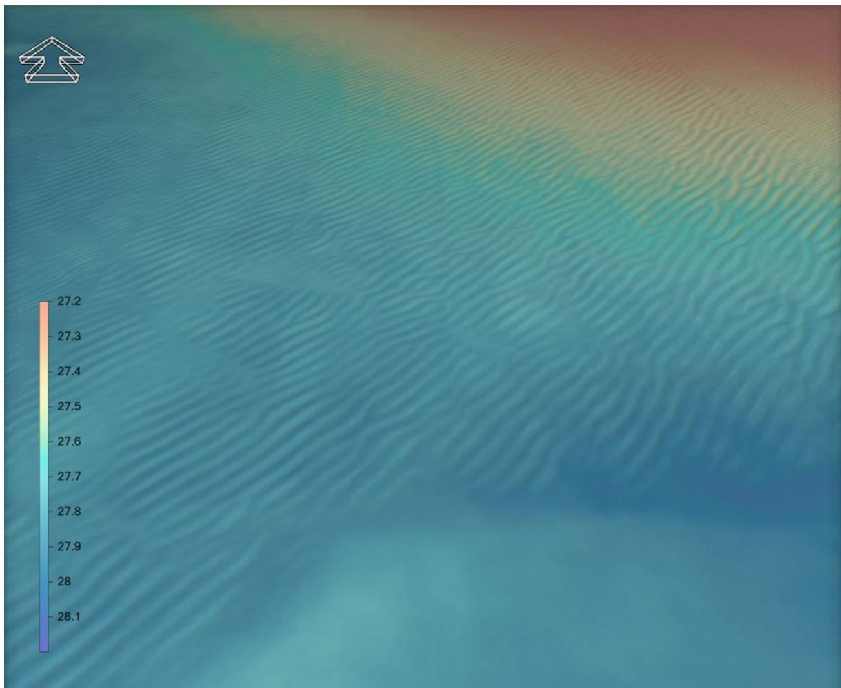
*Figure 17 3D image of an area of ripples within the Artificial Island project site.*
