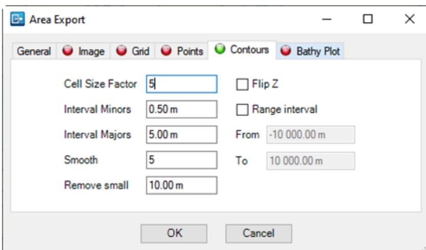
Figure 6 Artificial Island project site contour export parameters.
