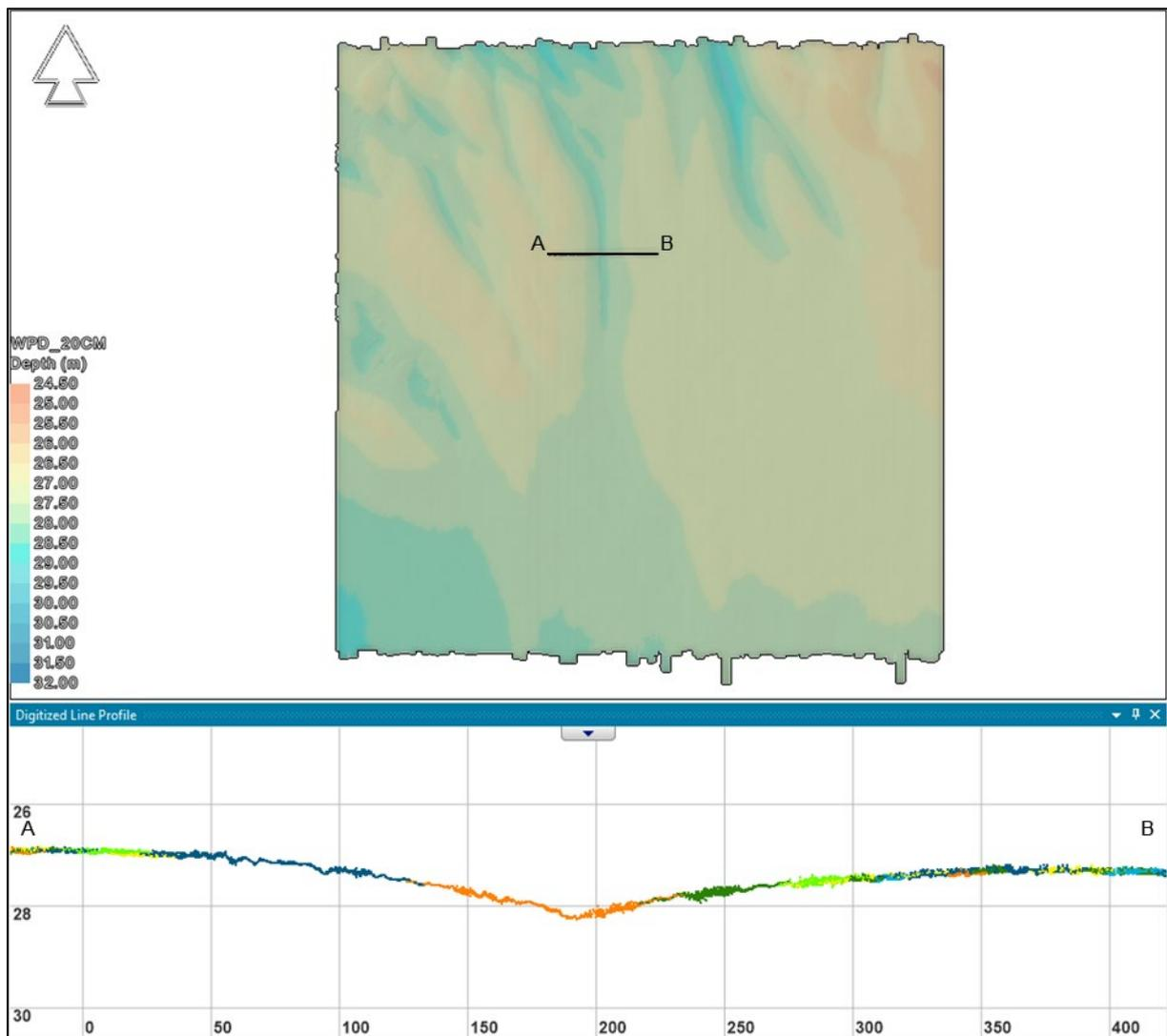
Figure 15 Profile showing vertical alignment of soundings in the Artificial Island project site.
