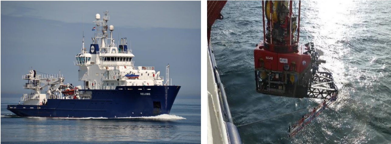
Figure 1.2 – DP Vessel Relume & Launch of ROV with Gradiometer Frame being extended.
