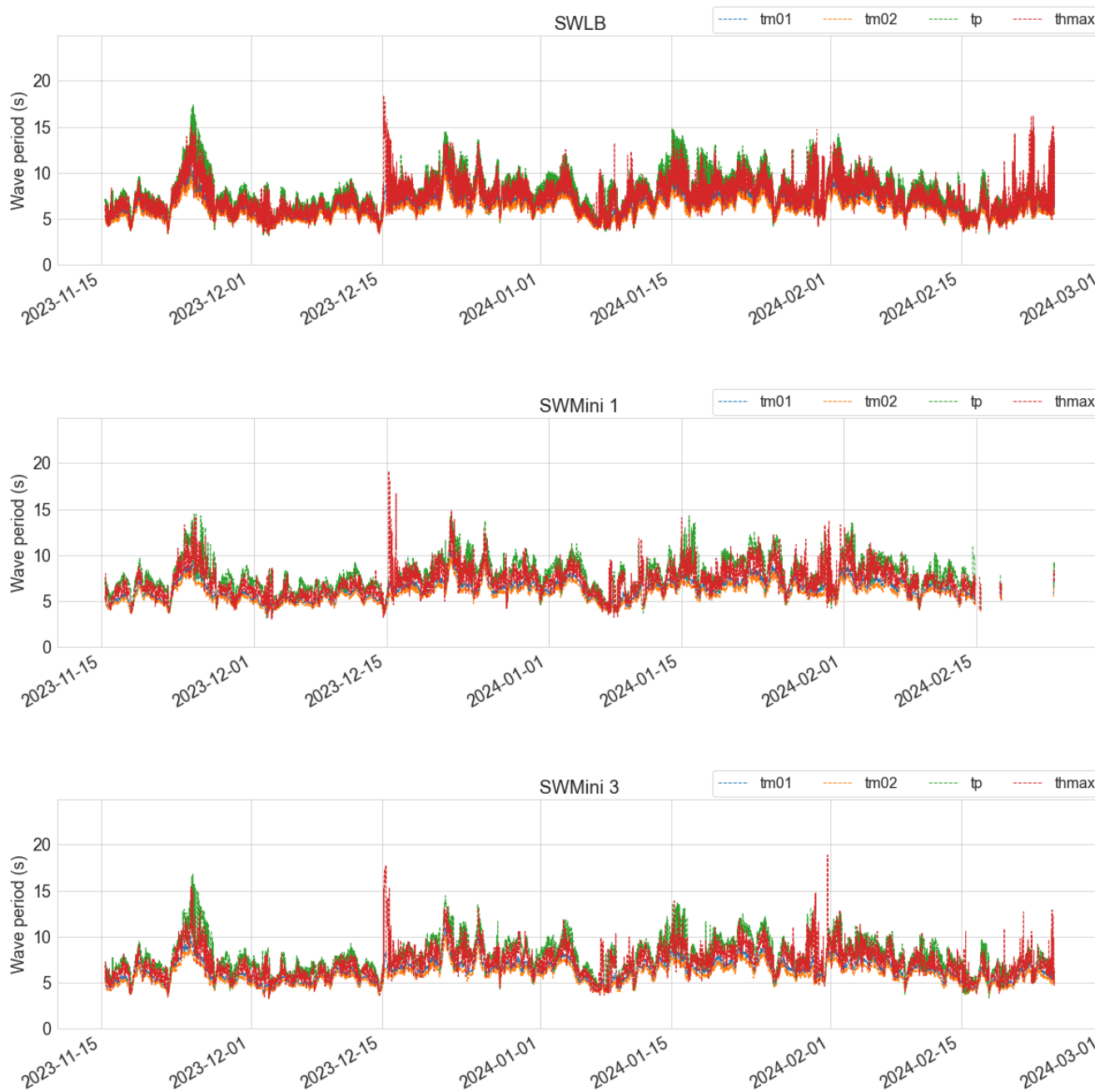
Figure B-28 Timeseries of wave periods from November 2023 until February 2024 measured by the SWLB (top), SWMini wave buoy 1 (middle), and SWMini 3 (bottom).
