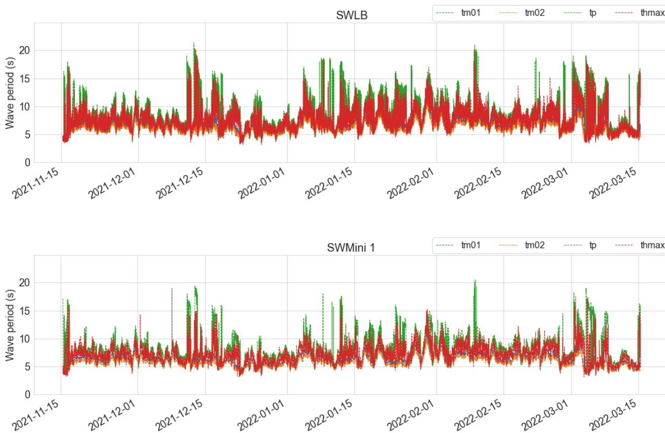
Figure B-22 Timeseries of wave periods from November 2021 until March 2022 measured by the SWLB (top) and SWMini wave buoy 1 (bottom).
