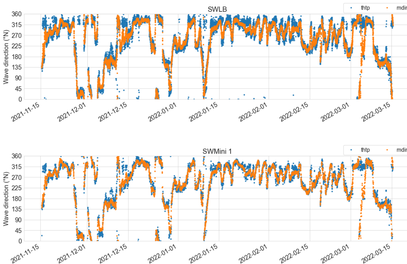
Figure B-15 Timeseries of wave directions from November 2021 until March 2022 measured by the SWLB (top) and SWMini wave buoy 1 (bottom). Please note that the y-axis for wave direction spans from 0° (bottom line) to 360° (top line).
