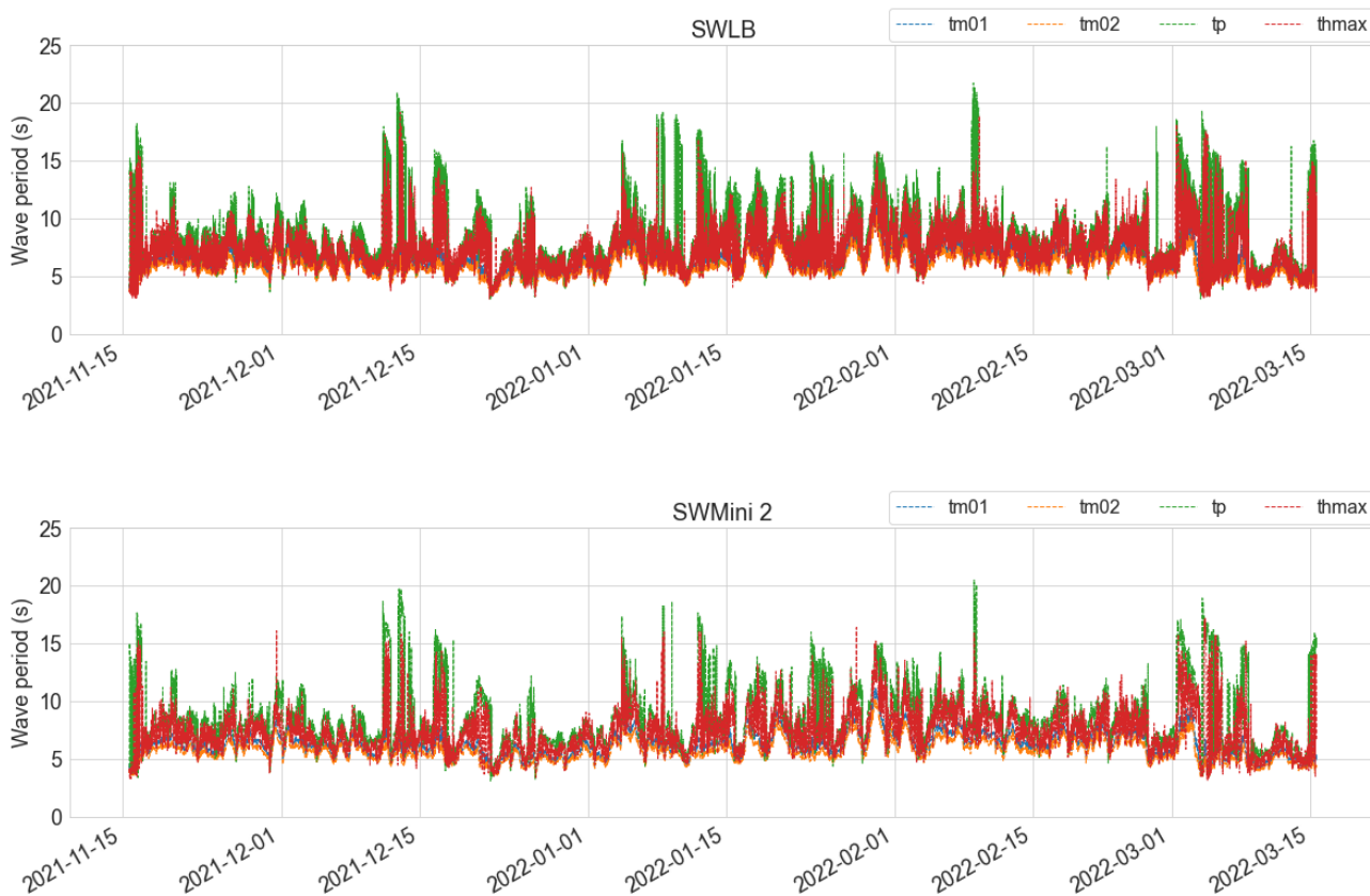
Figure B-22 Timeseries of wave periods from November 2021 until March 2022 measured by the SWLB (top) and SWMini wave buoy 2 (bottom).
