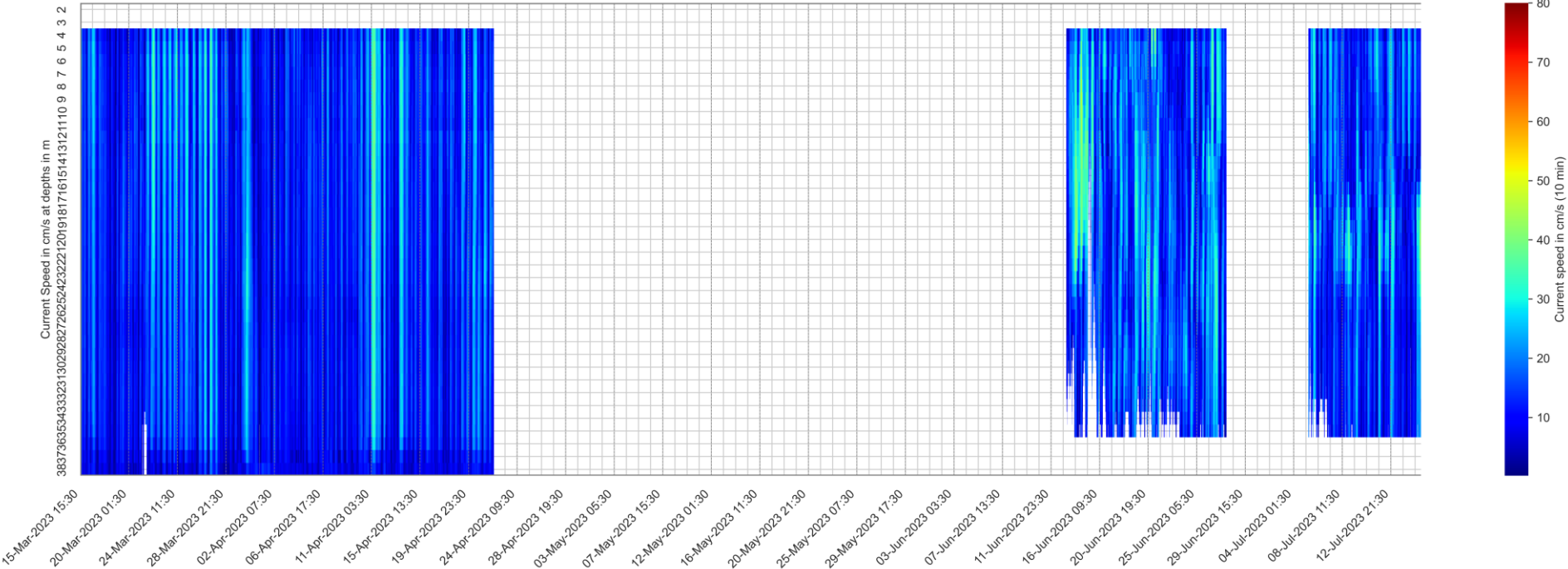
Figure B-47 Heatmap of SWLB (Aquadopp)-measured top-down current speed from March 2023 until July 2023.
