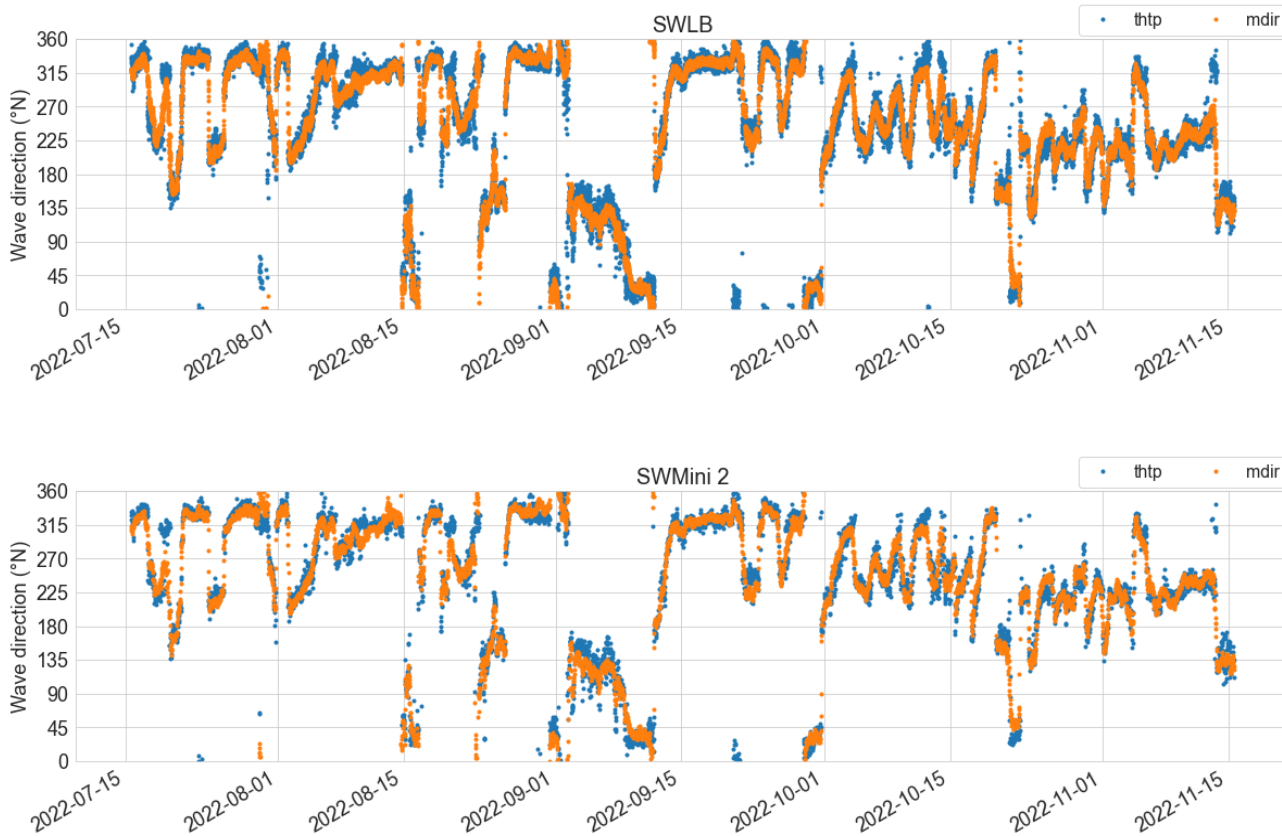
Figure B-17 Timeseries of wave directions from July 2022 until November 2022 measured by the SWLB (top) and SWMini wave buoy 2 (bottom). Please note that the y-axis for wave direction spans from 0° (bottom line) to 360° (top line).
