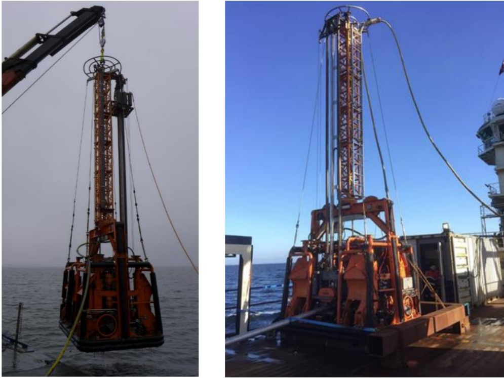
Figure 22: GeoCeptor - Combined Vibrocore and CPTU rig
