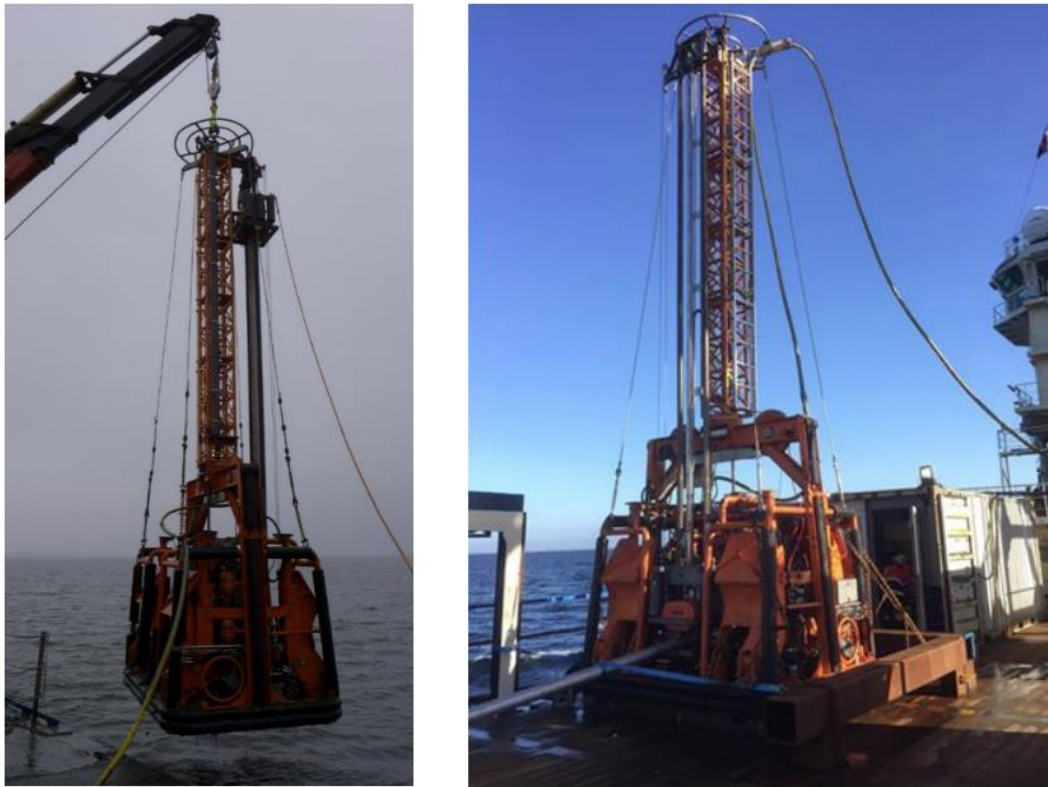
Figure 29: GeoCeptor - Combined Vibrocore and CPTU rig
