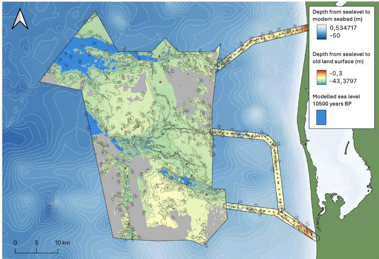
Figure 11 Modelled coastline at ~10500 years BP, showing inundation of the lower channel systems. Contour lines outside the OWF site and cable routes represent modern bathymetry below sea level. Red dots indicate the locations of vibrocores.
