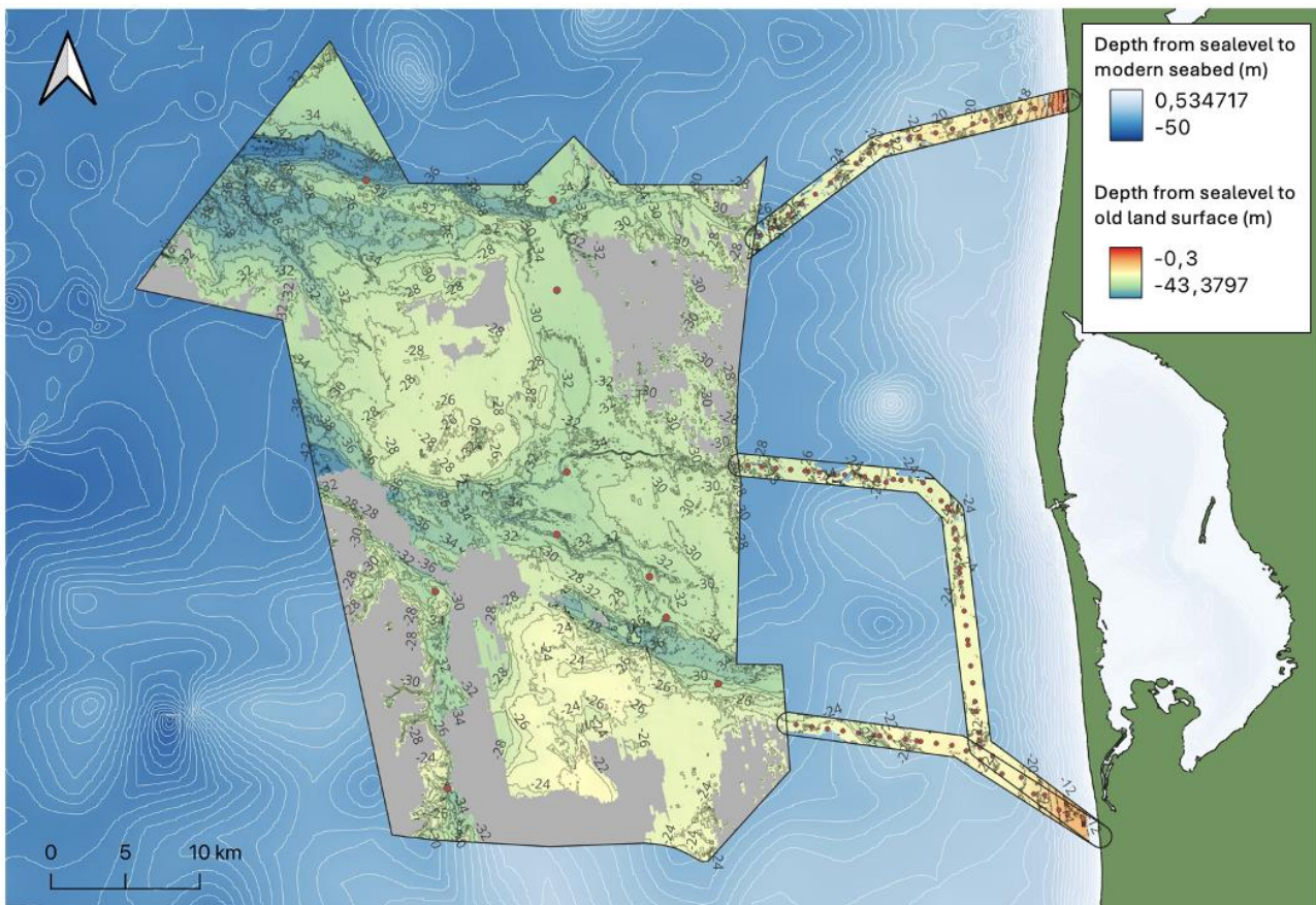
Figure 10 Modelled coastline at ~11000 years BP, showing no inundation of the area. Contour lines outside the OWF site and cable routes represent modern bathymetry below sea level. Red dots indicate the locations of OWF vibrocores.
