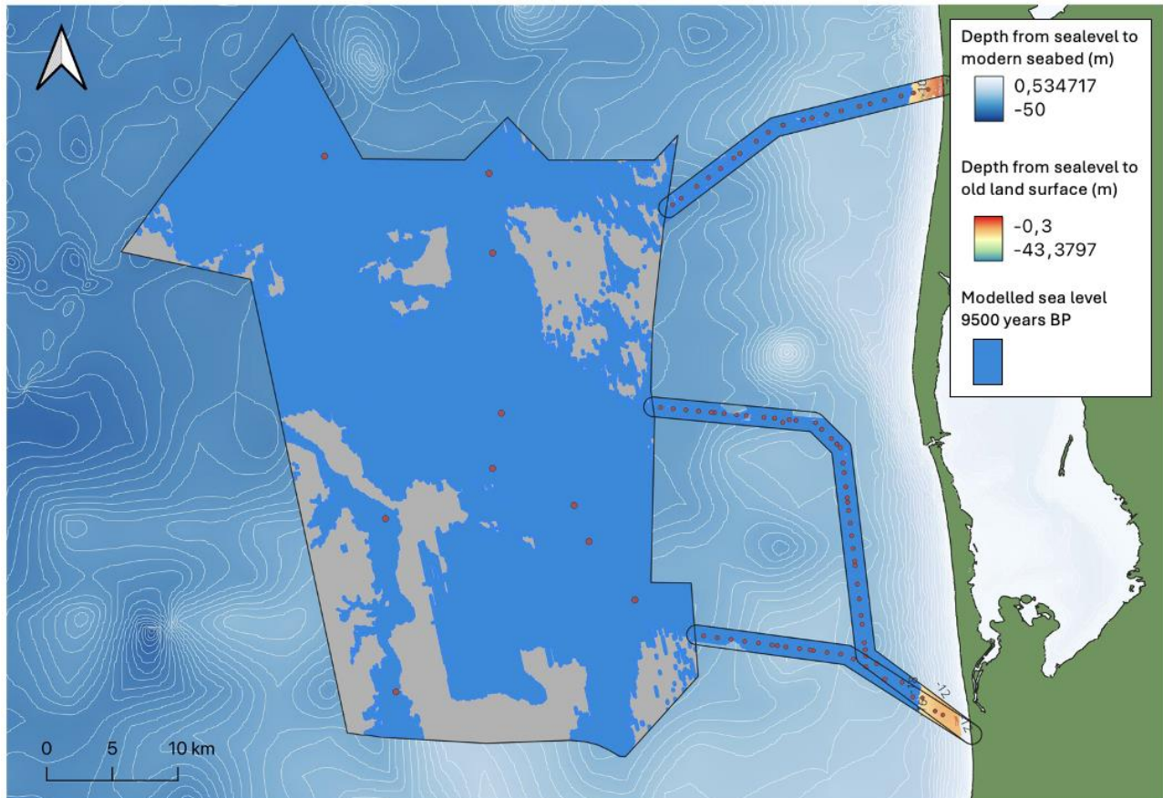
Figure 13 Modelled coastline at ~9500 years BP, showing inundation across both the OWF site and the cable routes. Only small area to the east in the northern and southern cable route remain a land surface. Contour lines outside the OWF site and cable routes represent modern bathymetry below sea level. Red dots indicate the locations of OWF vibrocores.
