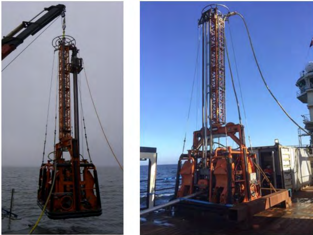
Figure 54: GeoCeptor - Combined Vibrocore and CPTU rig
