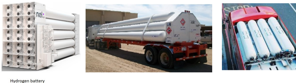
Figure 12: Hydrogen storage, transportation and fuel tank.
