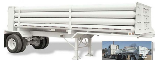
Figure 26: Trailer and storage is same vessel.
