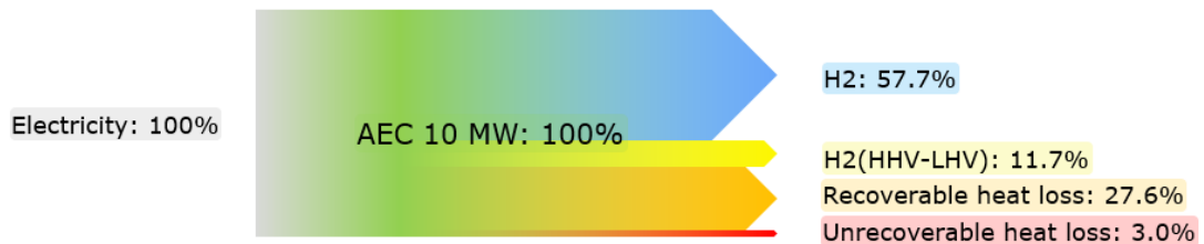
Figure 9: The energy inputs and outputs of an AEC (2020, 10 MW hydrogen plants).
