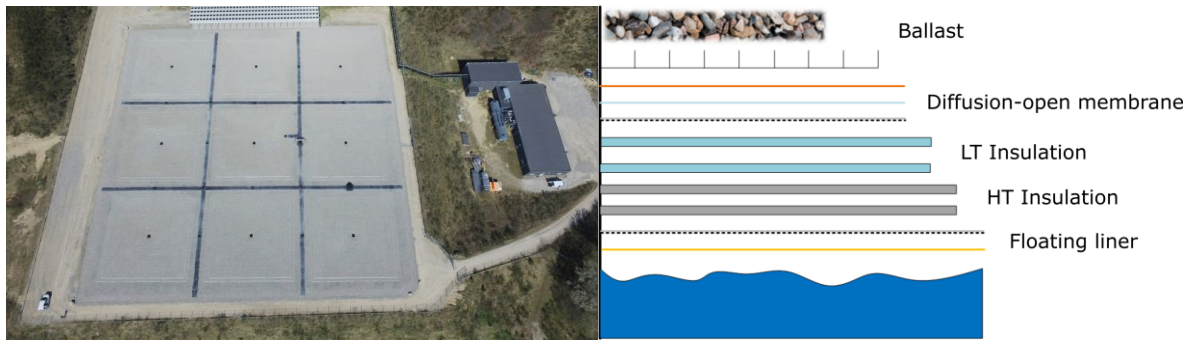
Figure 3: Illustrations of the lid in SUNSTORE 3 in Dronninglund. The lid construction is developed by Arcon-Sunmark and now implemented by Aalborg CSP [21].
