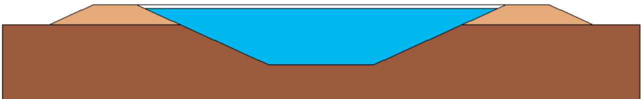
Figure 2: Principle sketch of a cross section of a PTES [15]. Blue color is water, brown color is undisturbed soil and sand color is excavated soil build into embankments around the excavation.
