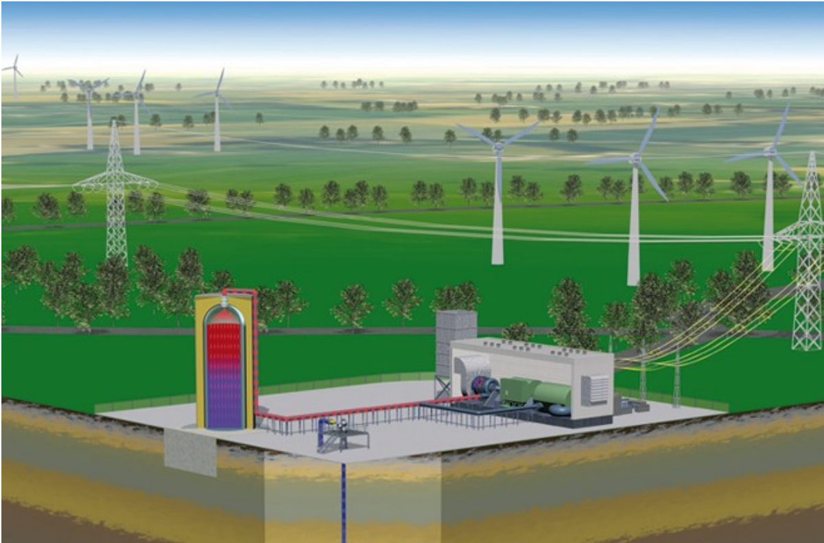
Figure 7: RWE's vision for an ACAES plant [15].
