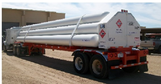
Hydrogen tube truck/trailer
