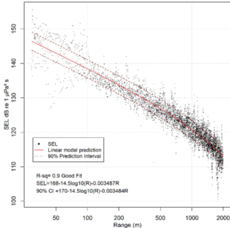
Figure 6.2: Sound Exposure Level measurements and curve fit for 360 tip sparker, during a sound source verification study in the North Sea (Pace, Robinson, Lumsden, & Martin, 2021).
