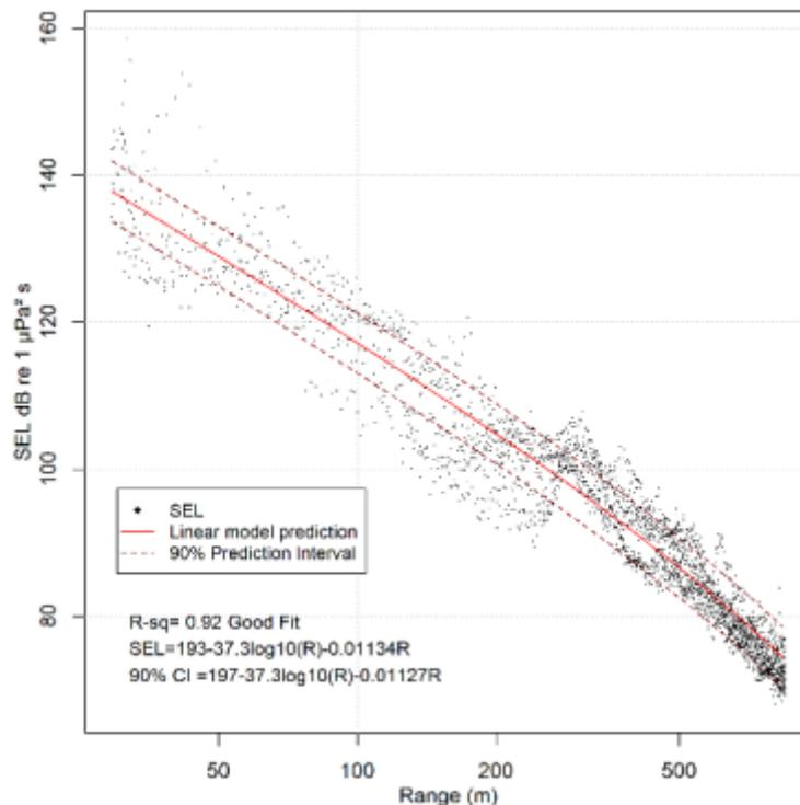
Figure 6.1: Sound Exposure Level measurements and curve fit for Innomar Medium 100, during a sound source verification study in the North Sea (Pace, Robinson, Lumsden, & Martin, 2021).
