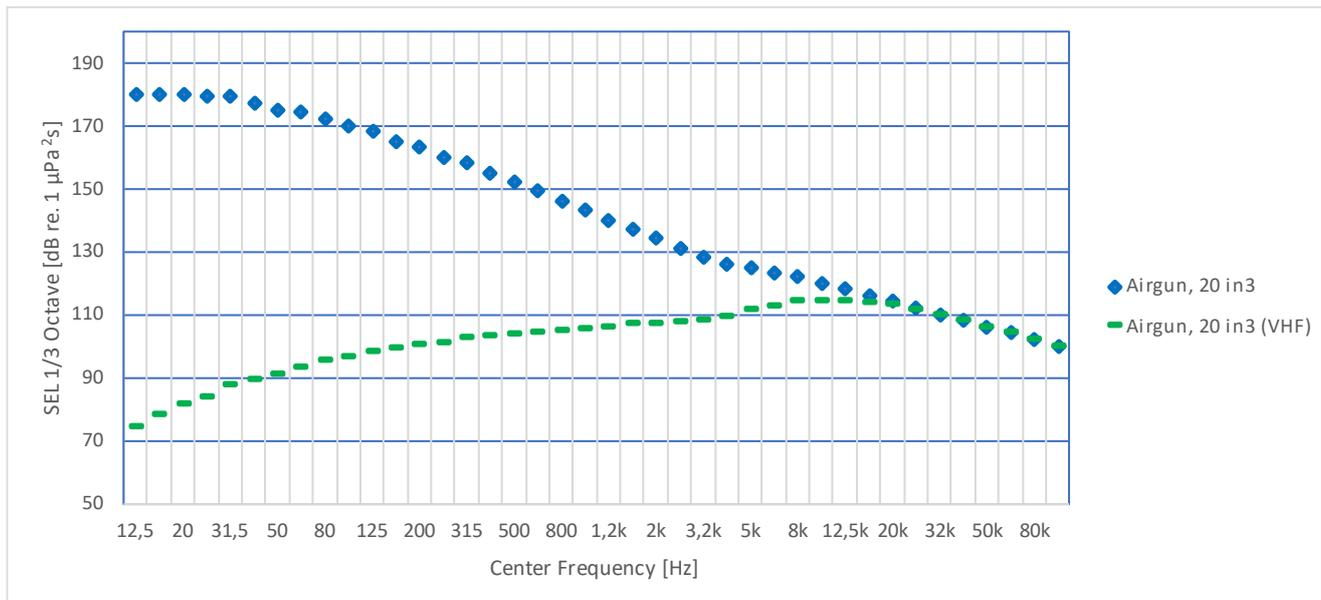
Figure 6.6: Equivalent omnidirectional point source model frequency spectrum for the Mini G 20 cu. inch airgun.
