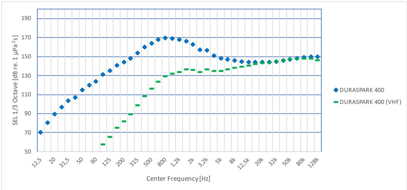
Figure 6.5: Equivalent omnidirectional point source model frequency spectrum for the Duraspark 400 sparker. The source model is calibrated to fit measurement results from (Pace, Robinson, Lumsden, & Martin, 2021), but adjusted in source level to represent information from client.
