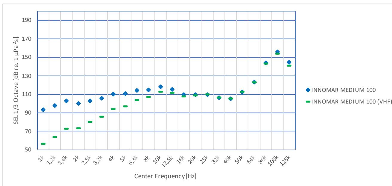
Figure 6.4: Equivalent omnidirectional point source model frequency spectrum for the Innomar Medium 100 parametric SBP. The source model is calibrated to fit measurement results from (Pace, Robinson, Lumsden, & Martin, 2021).
