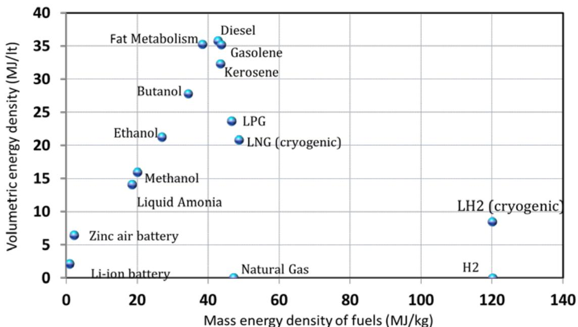
As shown, both weight and volume of batteries are very high, relative to the energy volumes they hold. Even with electric propulsion being inherently more energy efficient compared to combustion engines the lower energy density is a deal breaking barrier for widespread electric applications in modern commercial aviation.
