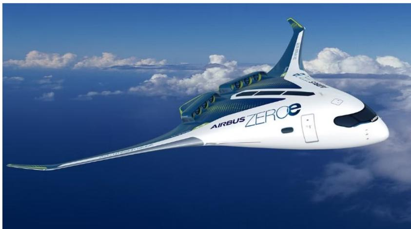
Making aircraft design more efficient (increasing the lift/drag ratio) is one way of meeting some the challenges of hydrogen concerning volume and range. Novel and radical aircraft design like Lockheed Martin's box-wing concept (Mehedi, Redonnet, & Hernadi, 2021), Boeing's transonic truss-braced concept (Boeing, 2023) or the Blended Wing Body (BWB) that
