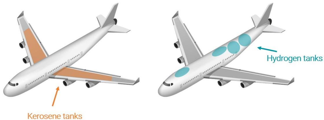
The need for fitting hydrogen tanks inside the fuselage in a CTW design (Conventional Tube-and-Wing Design) significantly increases the wetted area compared to volume for passenger and cargo, leading to increased parasitic drag, which will reduce the efficiency of the aircraft.
