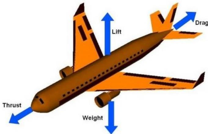
Each force has its own direction, opposing force, and factors that affect its effect. These forces balance the trajectory of the aircraft where lift opposes weight and thrust opposes drag. The four forces are explained in the table below.
