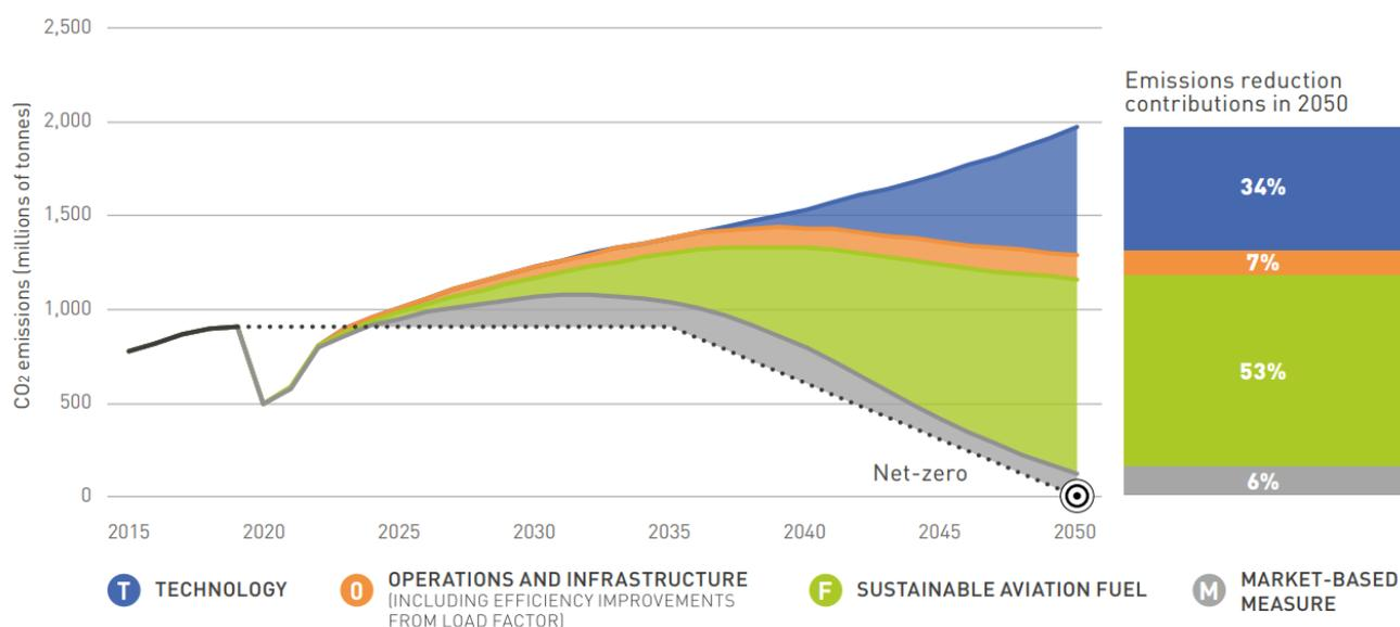
Figure 14 shows projected emissions in ATAGs Waypoint 2050 scenario 3, relying heavily on new technologies including electric aircraft up to 100 seats, zero emissions aircraft for 100-200 seat and hybrid electric powered unconventional larger aircraft. According to this scenario at substantial part of the necessary CO<sub>2</sub> emission reduction would even with extensive use of new technologies have to come from the use of sustainable aviation fuels.
