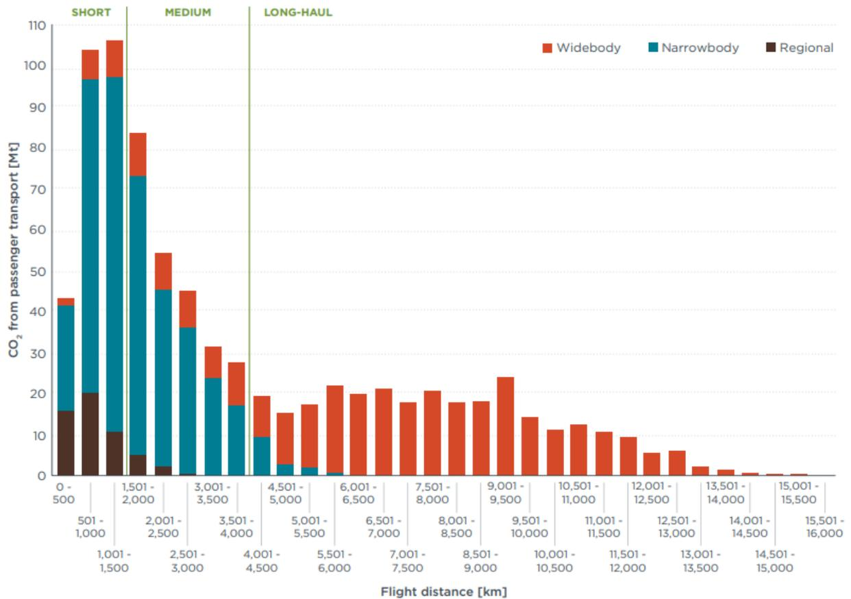
The figure highlights how short to medium-haul flights emit significant shares of the total CO<sub>2</sub> emissions from aircraft. With each stage length group responsible for about one third. Each of the three categories (short-, medium- and long-haul) make up approximately one third of total emissions.
