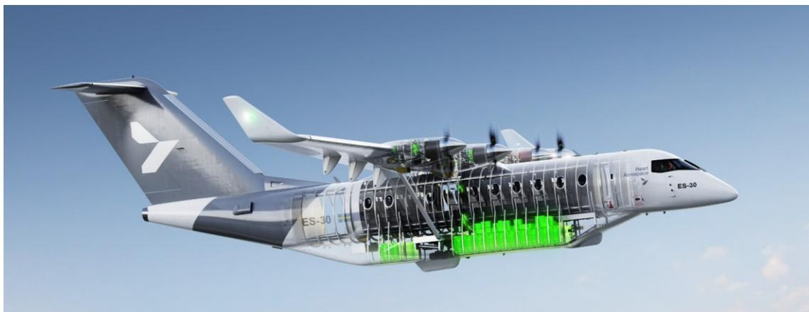
The battery is located as low as possible. In addition, illustration also shows how the wings are attached through a high-wing concept on the fuselage, similar to the configuration on conventional turboprop aircraft.
