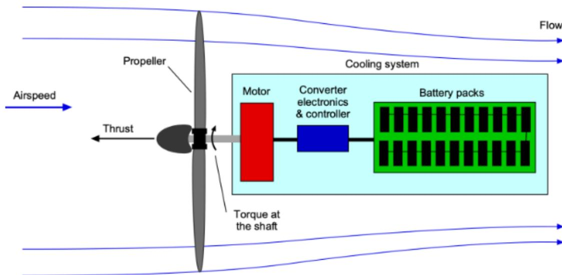
As shown in the figure, thrust is solely generated from the propellers and hence shares conceptual traits with the propellers of a conventional turboprop. As there is no combustion process there is also no exhaust to generate additional thrust, as is the case of the turbofan or, to a lesser degree, the turboprop engine (Embry-Riddle Aeronautical University, 2024c).
