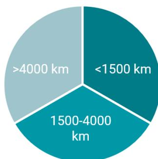
As seen in Figure 30, the emissions of aviation can be roughly divided into three categories each responsible for a third of global CO<sub>2</sub> passenger flight emissions. Narrow body aircraft are the dominant segment for short- and medium-haul flights (<4000 km). In contrast, longer flights of >4,000 km are primarily serviced by wide body aircraft. Regional flights of <500 km
