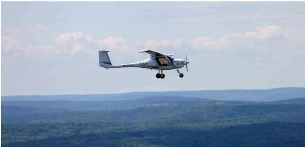
This model is a small two-seater aircraft mainly intended for pilot training with a battery capacity sufficient for up to 50 minutes of flight. Due to its intended use and small size, this aircraft has no relevance to commercial aircraft designed for passenger transport (EASA, 2020a). But this electric plane is the first example of an approved electric aircraft. As such it can be a step, in building experience with regulation and approval processes.
