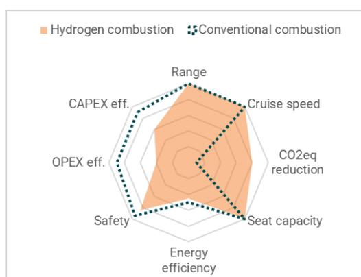
safer than kerosene while in others it has disadvantages. Even though hydrogen might be as safe as kerosene or even better the lack of experience handling hydrogen, leads to hydrogen scoring slightly lower safe score than conventional aircraft.
