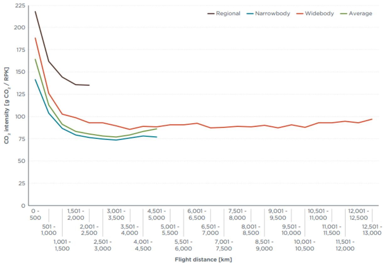
The graph from ICCT (2020) shows the CO<sub>2</sub> intensity across different flight distances for the three categories of aircraft. The three categories can be defined as the following:
